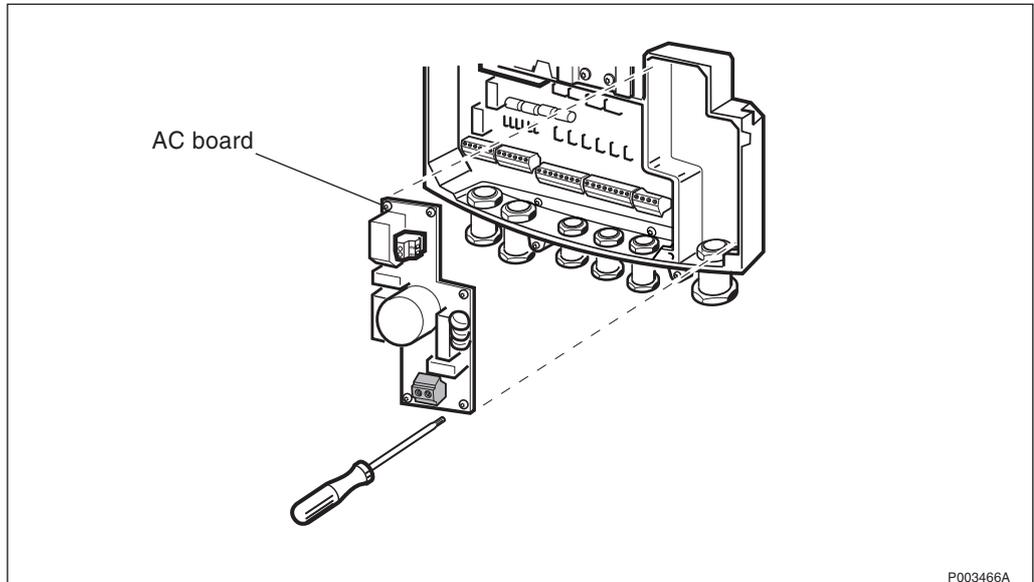
Figure 451 Removing the AC board
