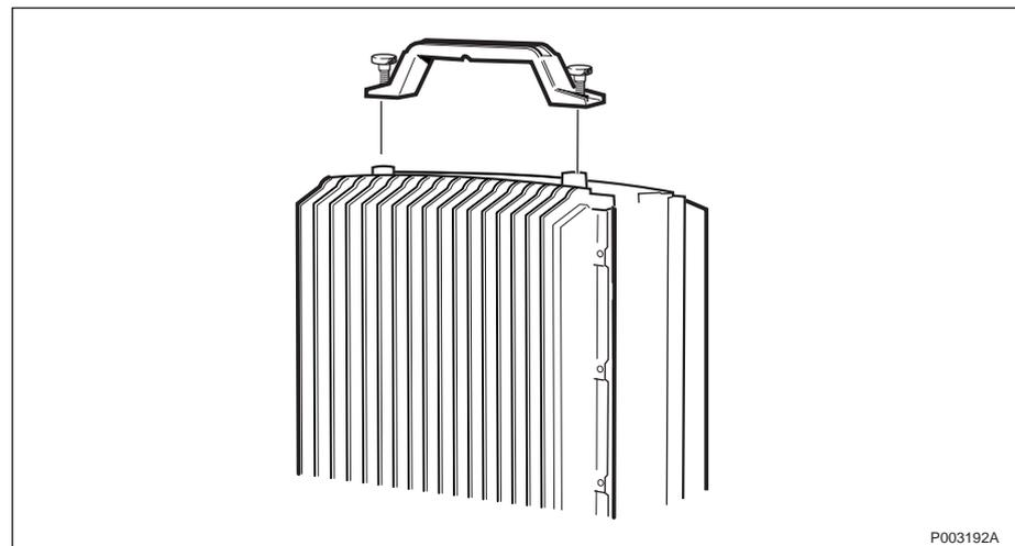
Figure 501 Mounting the optional lifting handle
