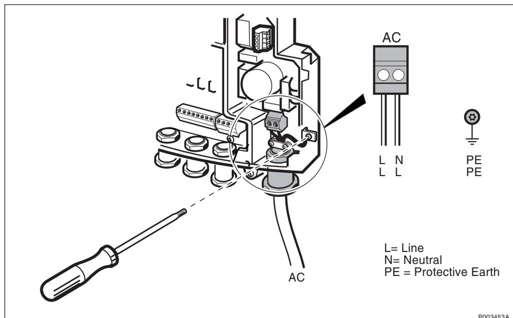
Figure 287 Connecting AC Mains Power
