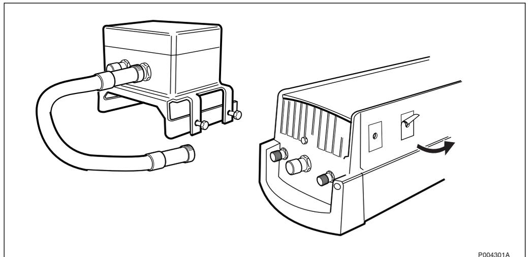
Figure 91 Removing the protective plastic tape
