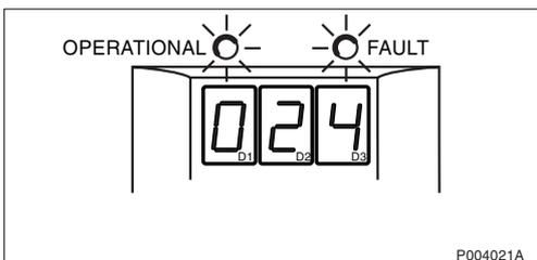
*Battery Fault.* Defective batteries or charging circuits are malfunctioning. Replace the batteries/power cabinet.
