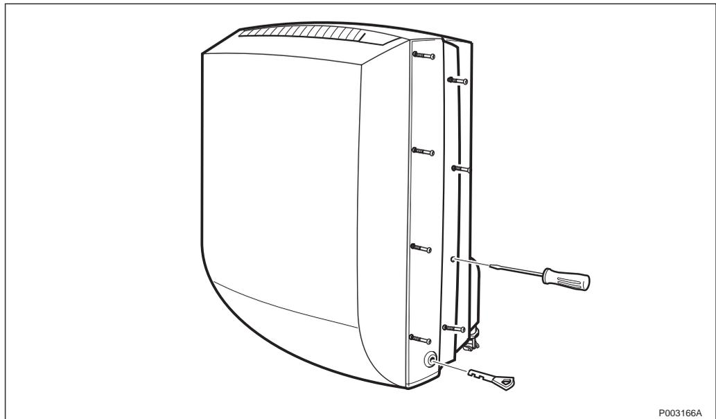
Figure 388 Sealing screws and key for the installation box door
