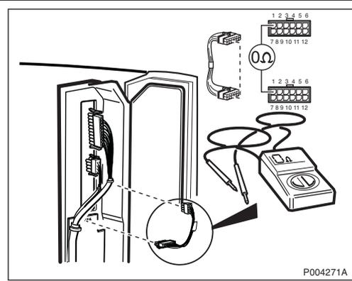
3/ The display cable is faulty. If there is 115/230 V present to the battery cabinet, verify that the display cable is properly connected and functional. This is done by measuring the resistance from pin to pin.
