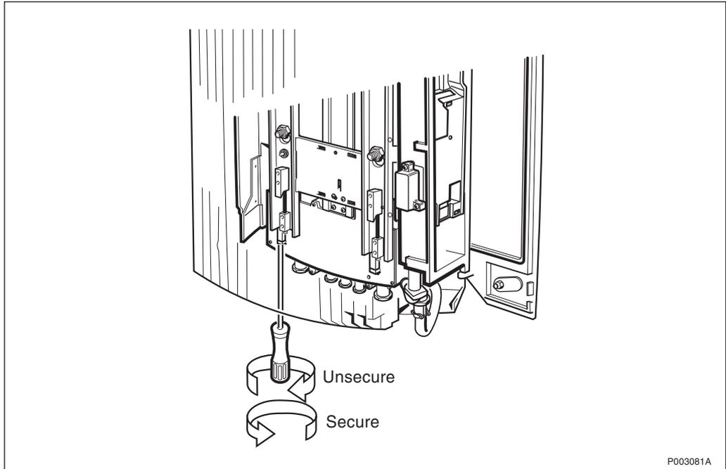
Figure 429 Unscrewing the locking device
