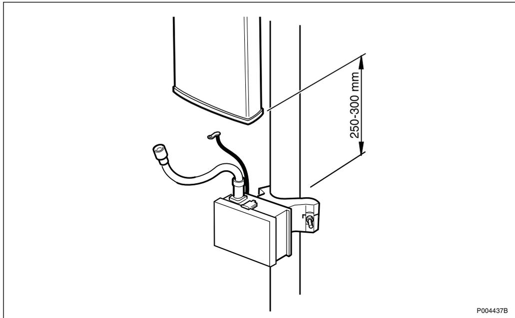
Figure 582 Lightning protection for 500 W EIRP GSM 1900 antenna
