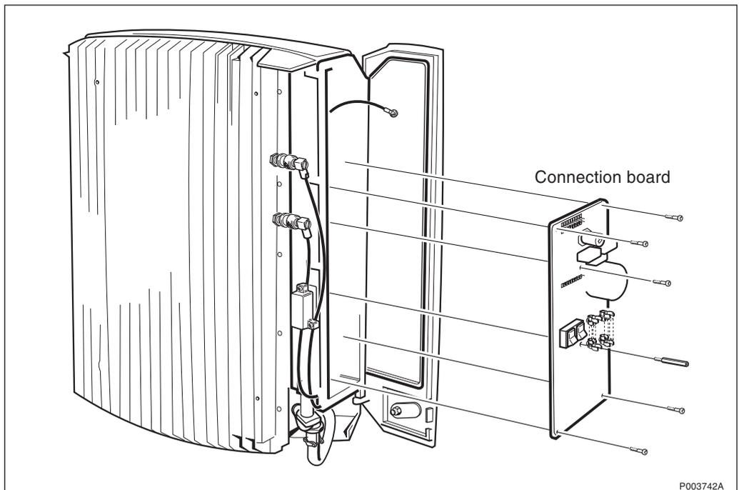
Figure 441 Removing the connection board
