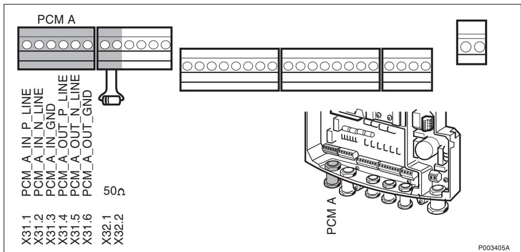
Figure 291 Connect the PCM A
