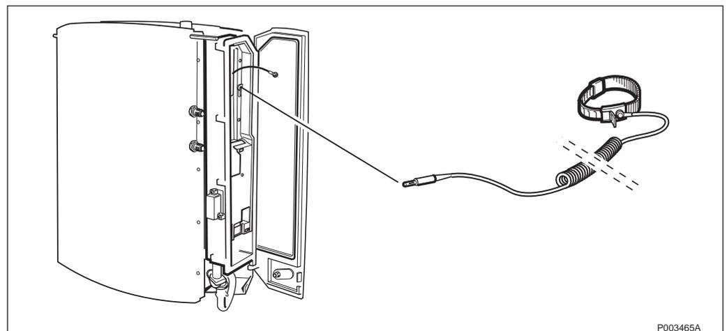
Figure 450 Connecting the ESD wrist strap
