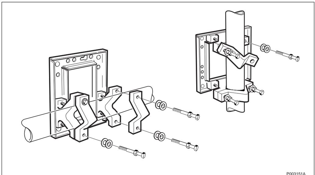
Figure 565 Pole fixture and mounting plate mounted on a tube
