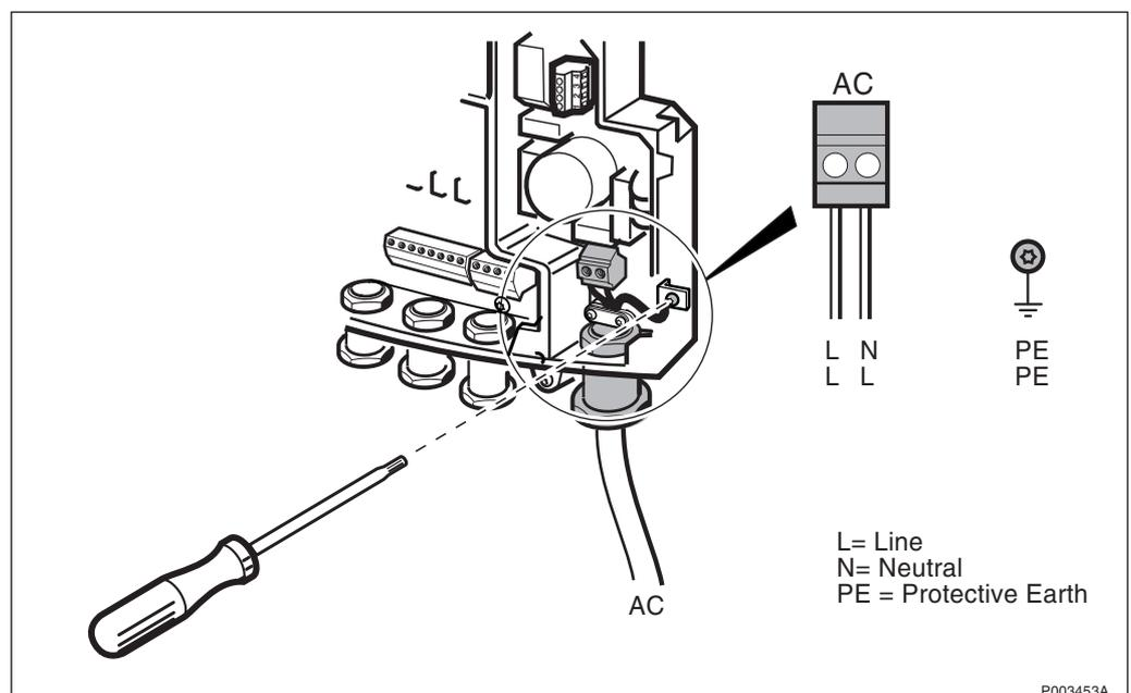
Figure 455 Loosening the Protective Earth in the AC section of the interface box
