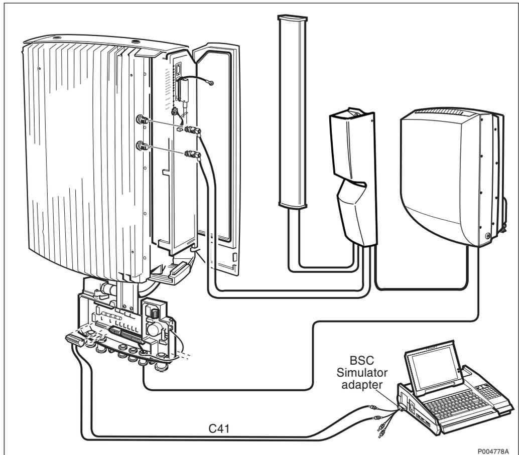
Figure 362 Test setup for GSM 900: 2 TRX Sector Configuration for T1 100  $\Omega$  (1.5 Mbit/s) and E1 120  $\Omega$  (2.0 Mbit/s)
