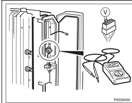
Measure that 115/230 V is present at the connector of the internal AC cable attached to the radio cabinet, to verify that the internal AC cable is undamaged. If voltage is present, replace the radio cabinet.
