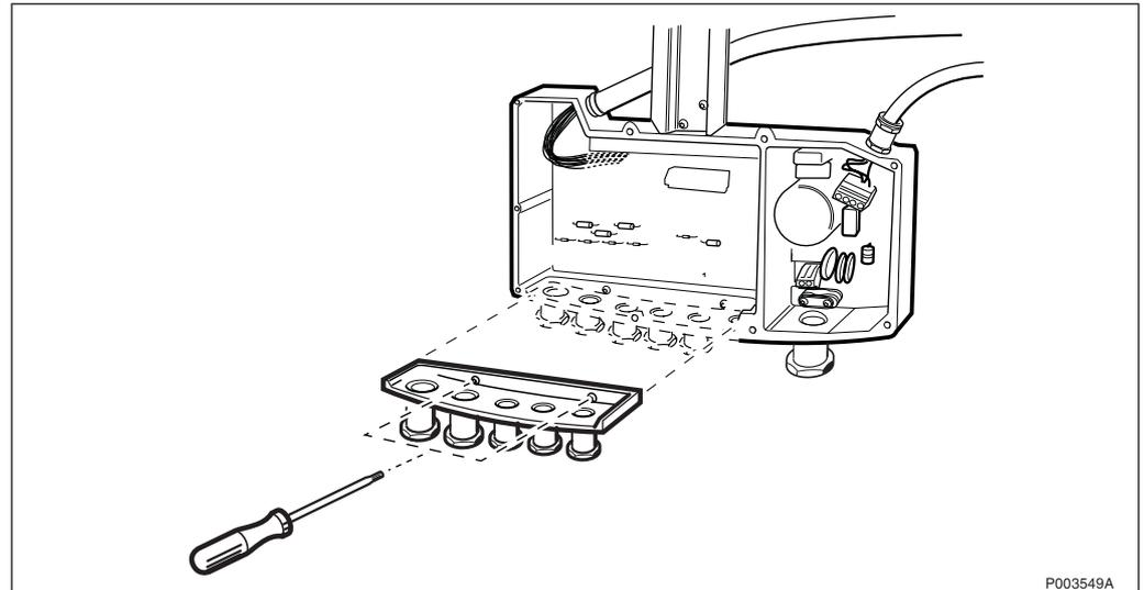
Figure 466 Loosening the gland plate
