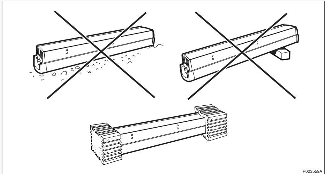
Figure 80 Handle the antenna with care
