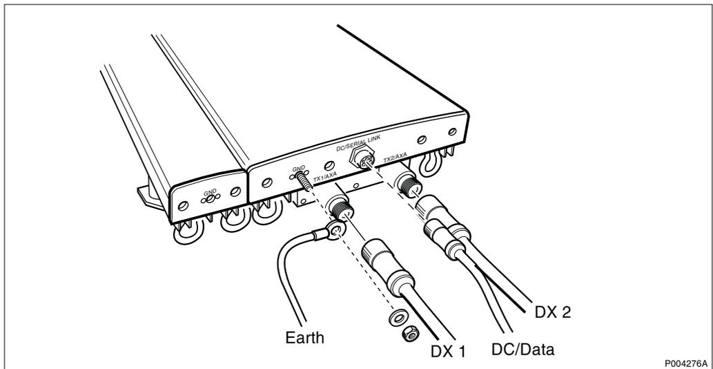
Figure 225 Connector overview of the GSM 1900 antenna 1250 W EIRP
