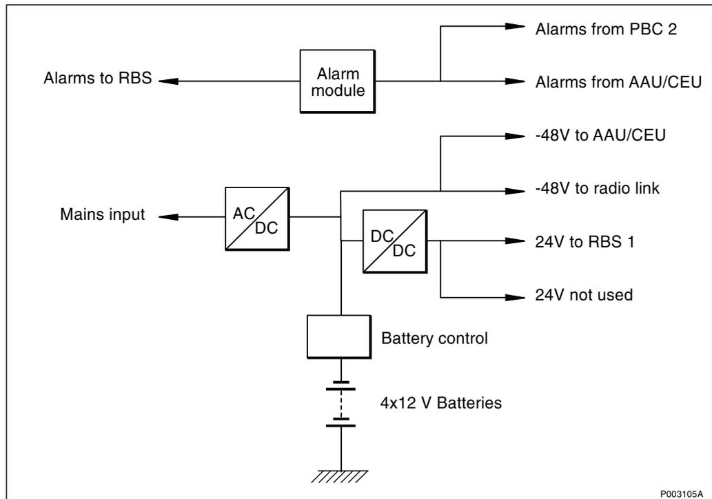
Figure 46 Block diagram of Power and Battery Cabinet
