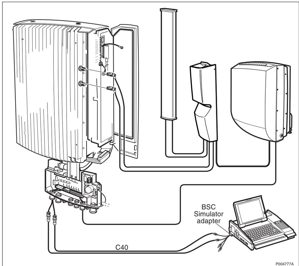
Figure 360 Test setup for GSM 900: 2 TRX Sector Configuration for E1 75  $\Omega$  (2.0 Mbit/s)
