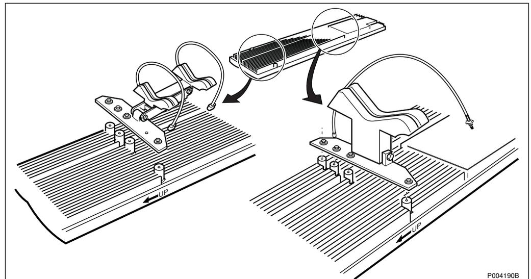
Figure 101 Attaching the upper and lower mounting fixture to the Base antenna and TX antenna (1250 W EIRP)
