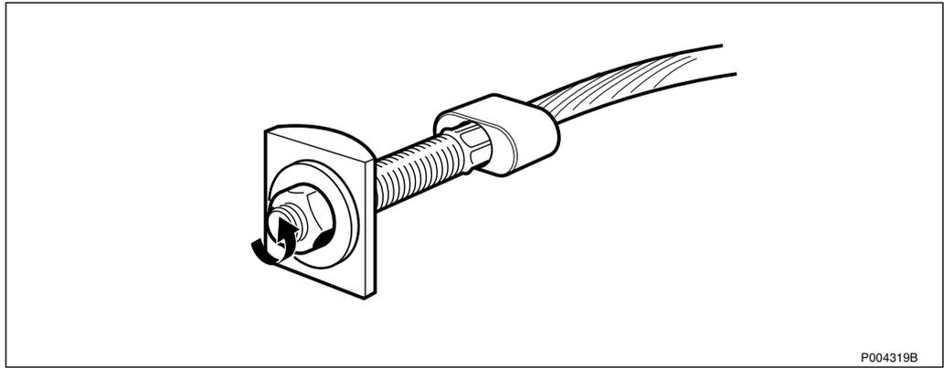
Figure 102 Adjusting the harness cable tightener
