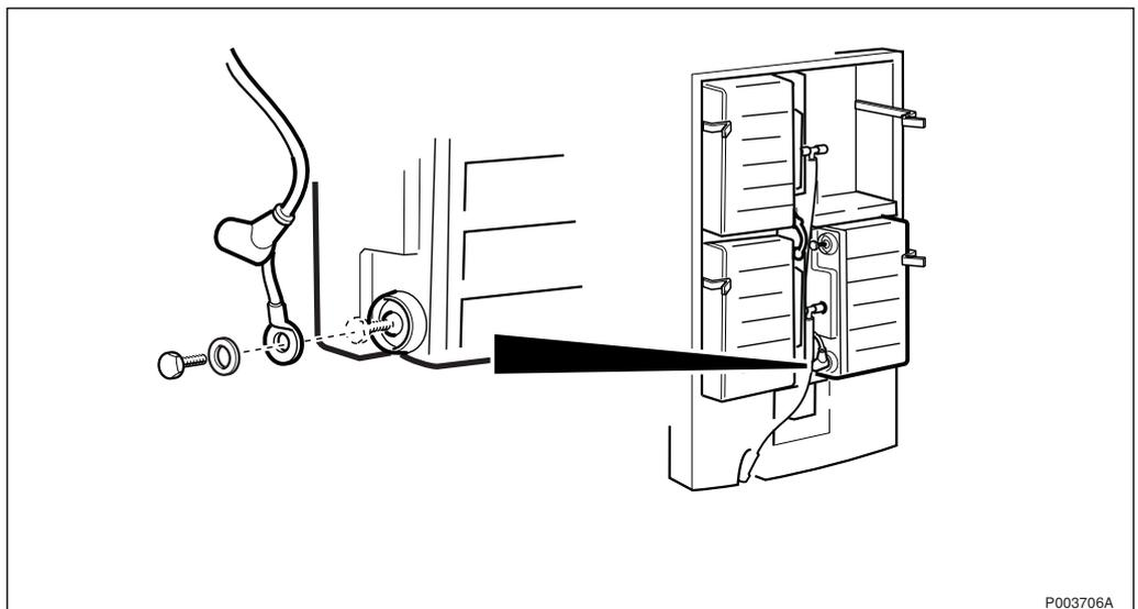
Figure 476 Disconnecting the minus-pole (-) of battery 3
