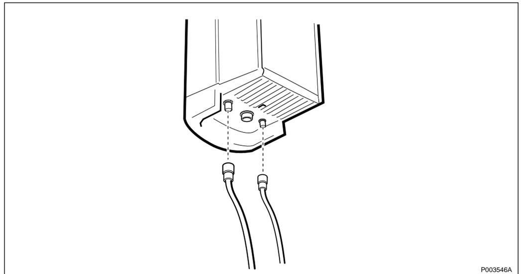
Figure 245 Antenna Coaxial connectors
