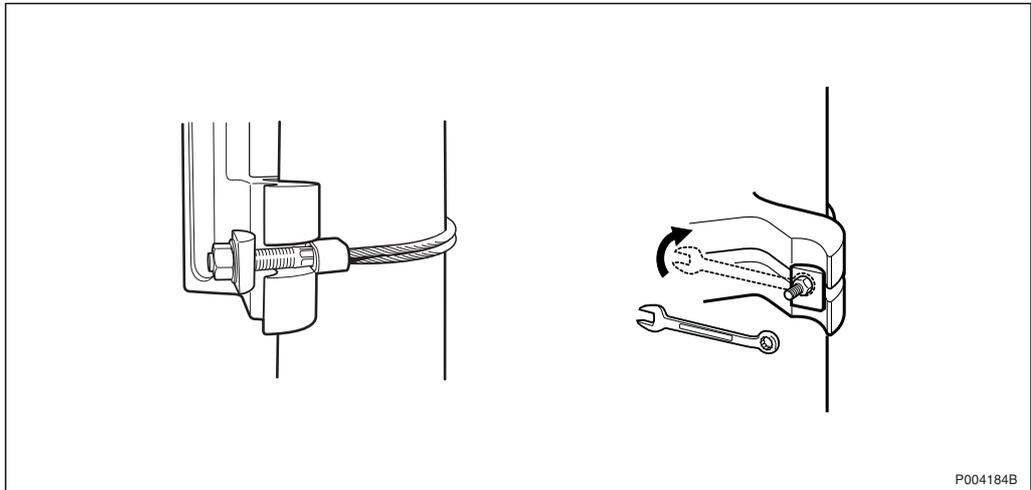
Figure 108 Tightening the harness cable
