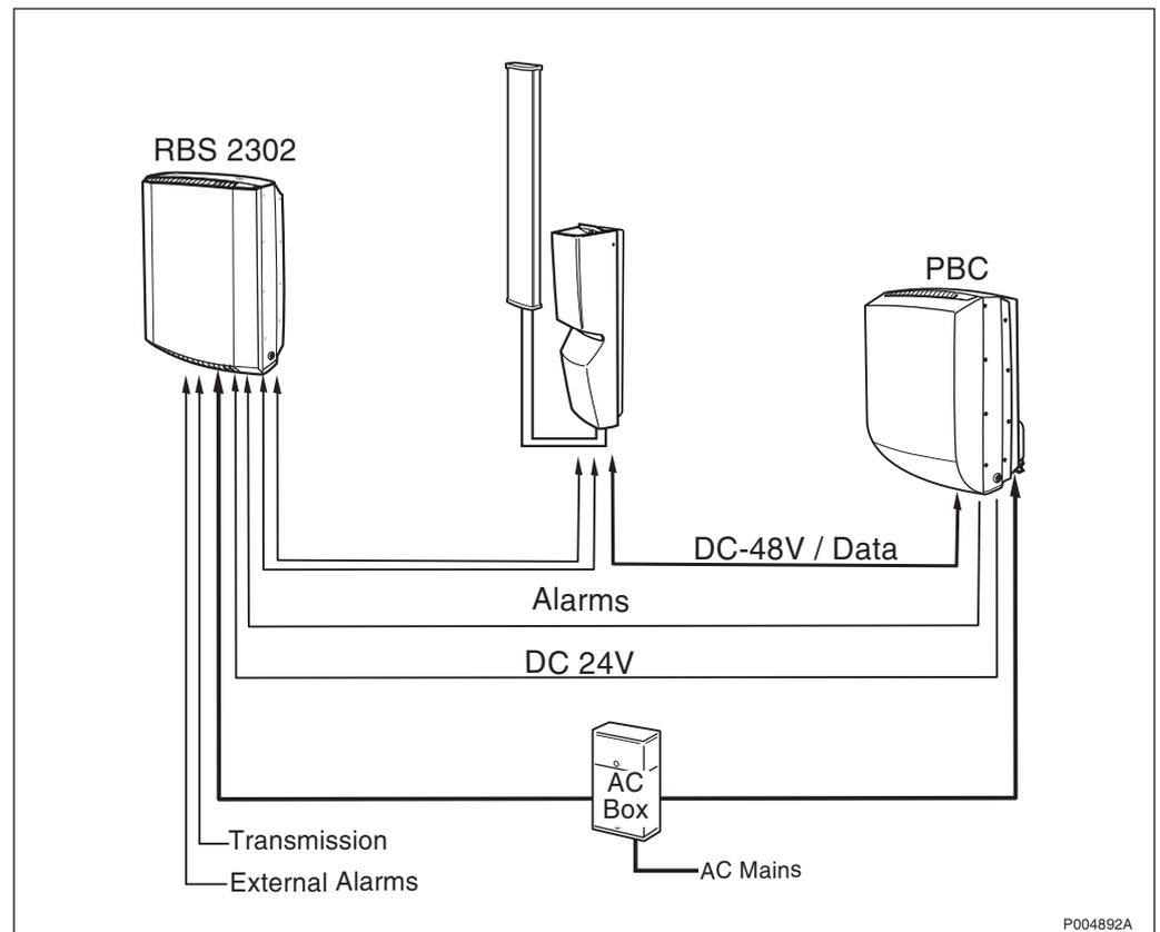
Figure 47 Configuration with 2 TRX
