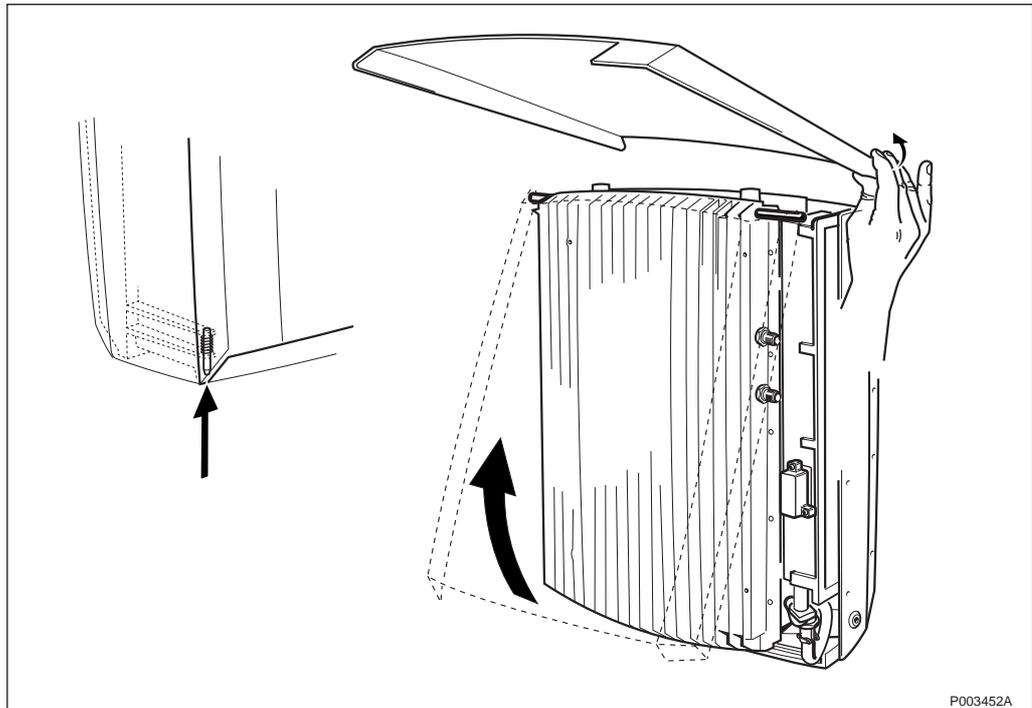
Figure 407 Replacing the front sunshield
