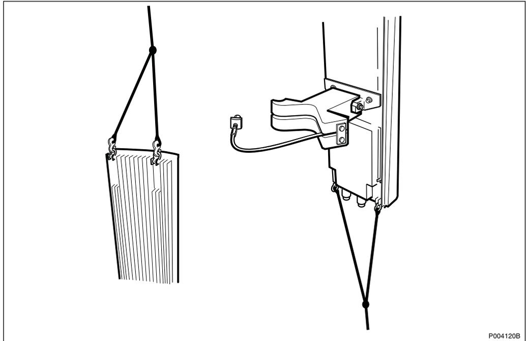
Figure 581 Lifting eyes
