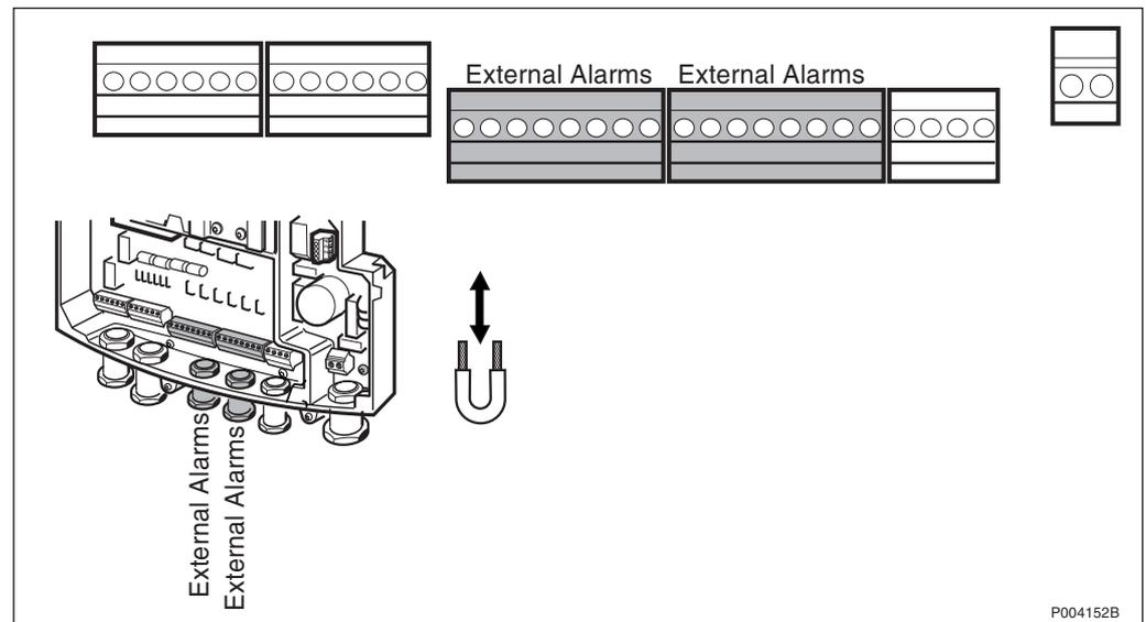
Figure 341 Test of closing alarm
