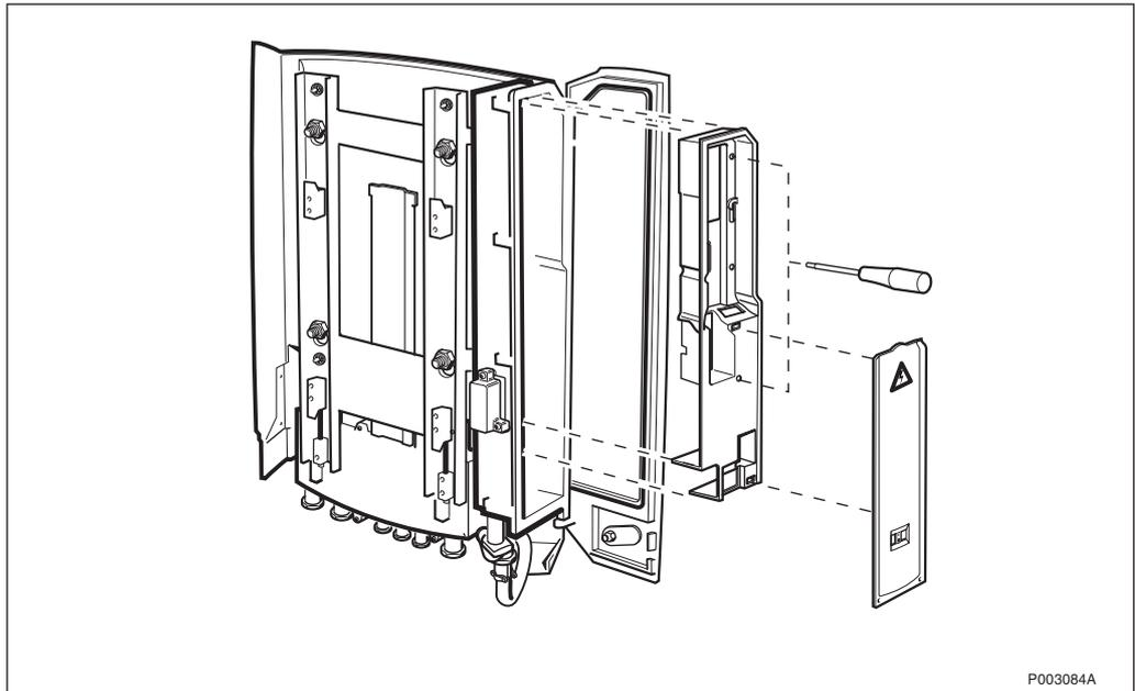
Figure 174 Removing the protection covers
