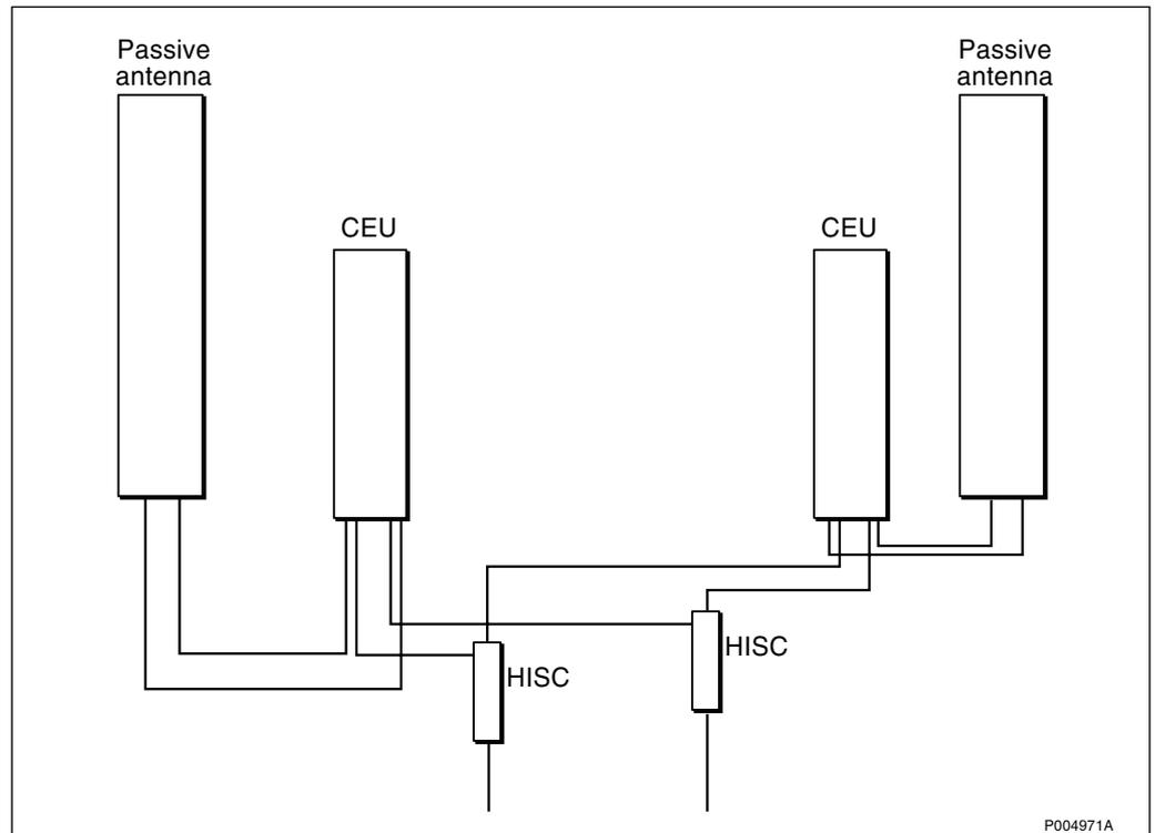
Figure 222 Connection of the HISC (Highway Splitter Combiner)
