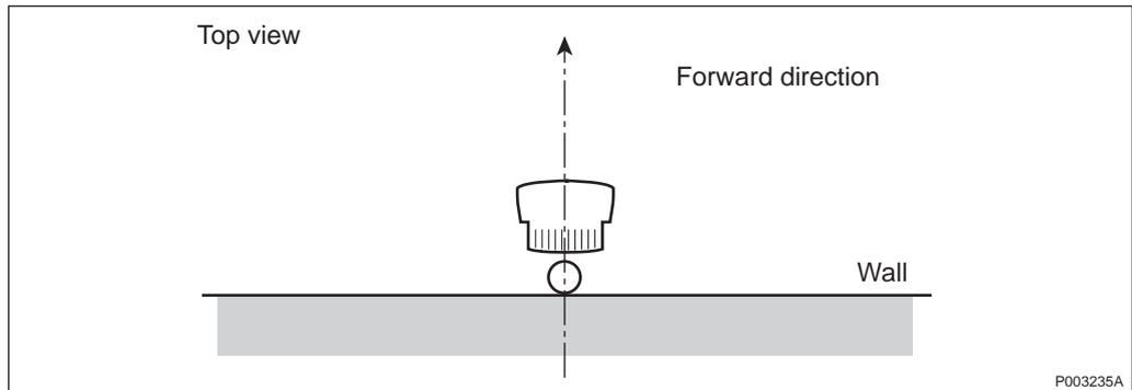
Figure 22 Ideal direction (perpendicular to the wall)
