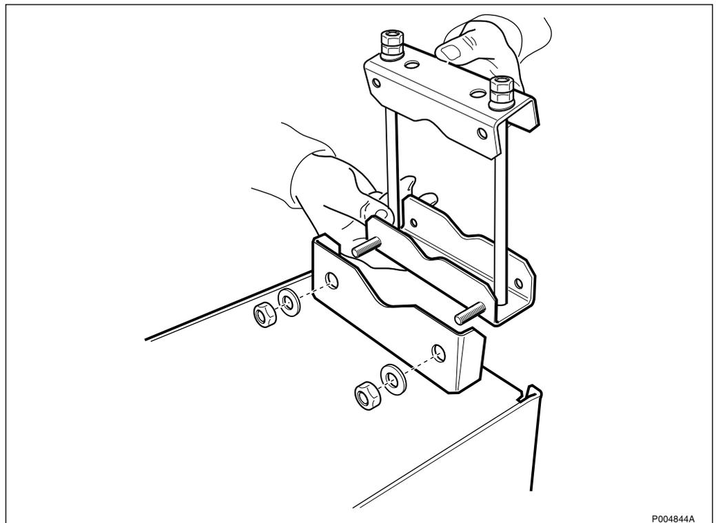
Figure 58 Mounting the lower mounting fixture with nuts and washers
