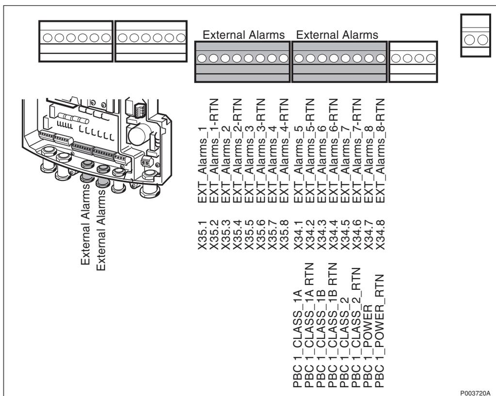
Figure 308 Examples of alarm input configurations
