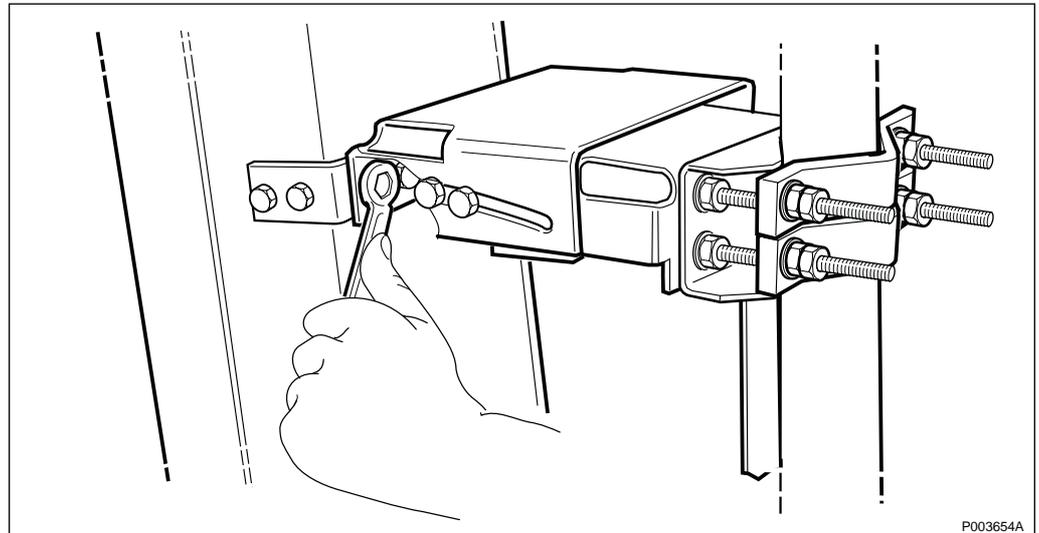
Figure 524 Loosening the four screws on the upper support
