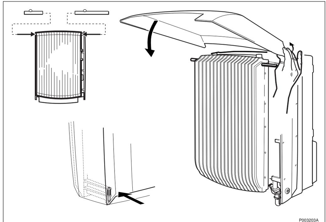
Figure 155 Mounting the front sunshield
