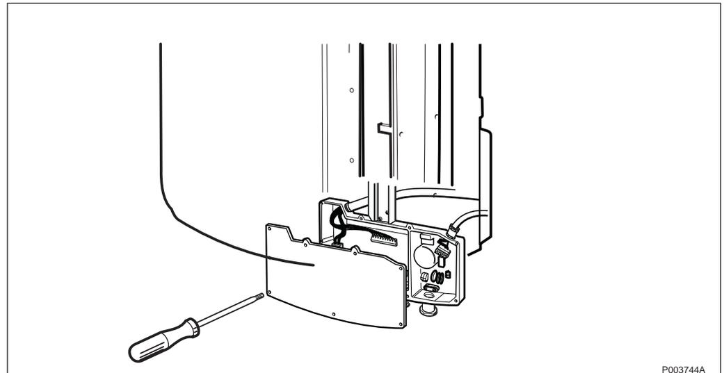
Figure 511 Loosening the interface box cover
