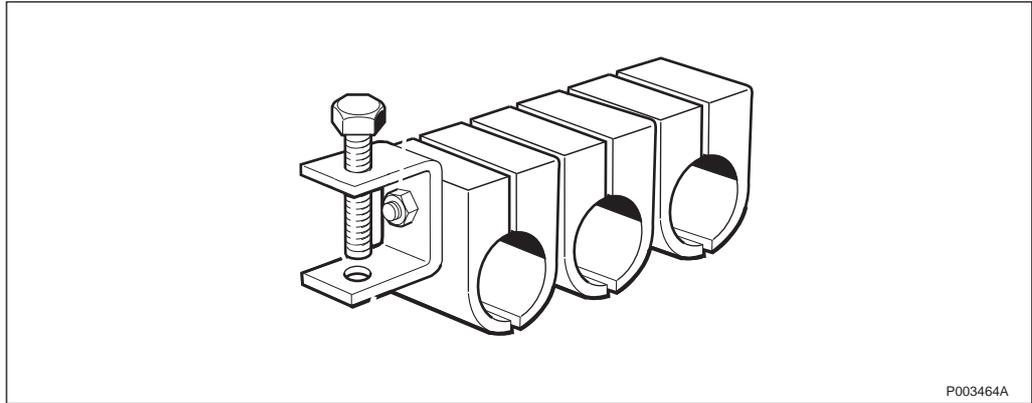
Figure 261 Cable Clamp NTM 201 215/3
