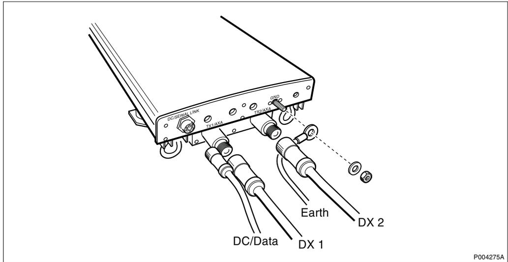
Figure 224 Connector overview of the GSM 1900 antenna 500 W EIRP
