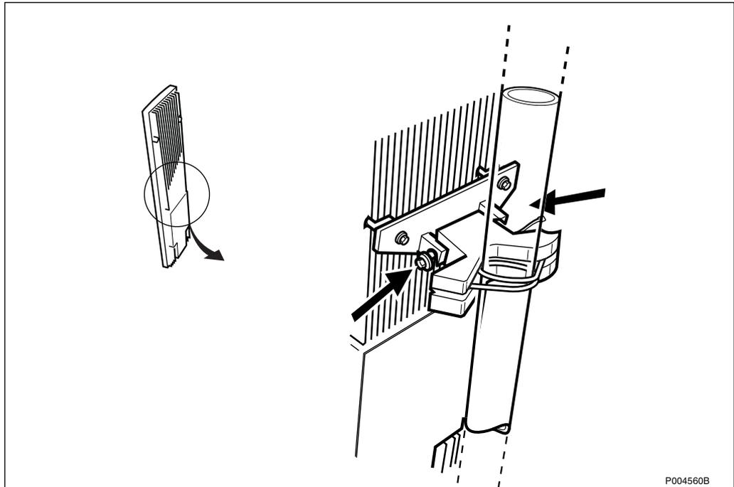
Figure 537 Tightening the two screws on the lower mount
