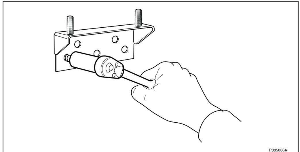
Figure 68 Fastening the upper mounting bracket to the wall
