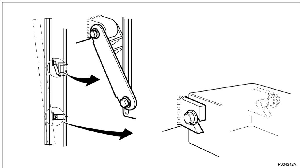
Figure 109 Fixing screws for the tilt linkage, and supporting screws on the lower pipe clamp
