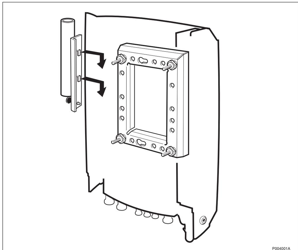
Figure 198 Mounting the lifting device
