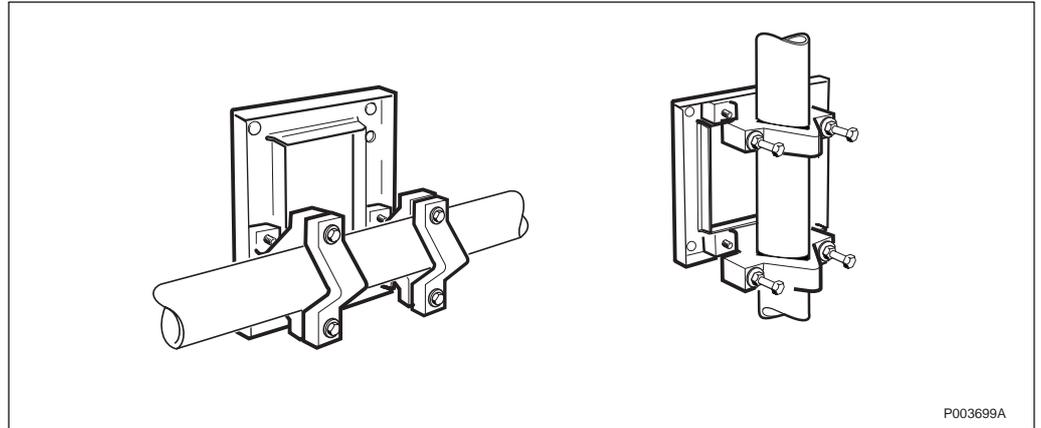
Figure 120 Mounting alternatives
