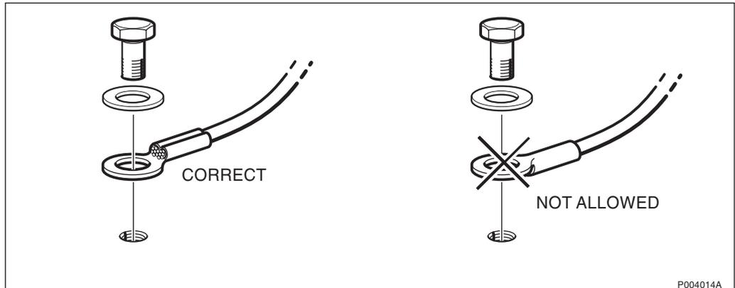
Figure 480 Connecting cable lugs to batteries
