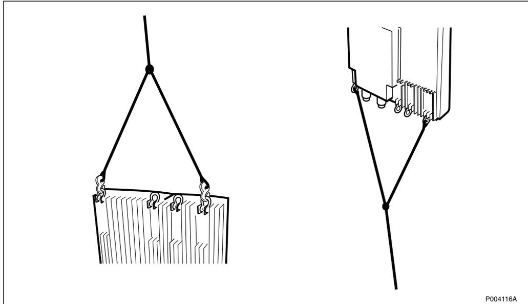
Figure 585 Lifting eyes
