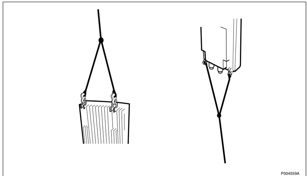
Figure 531 Securing the antenna in the lifting eyes
