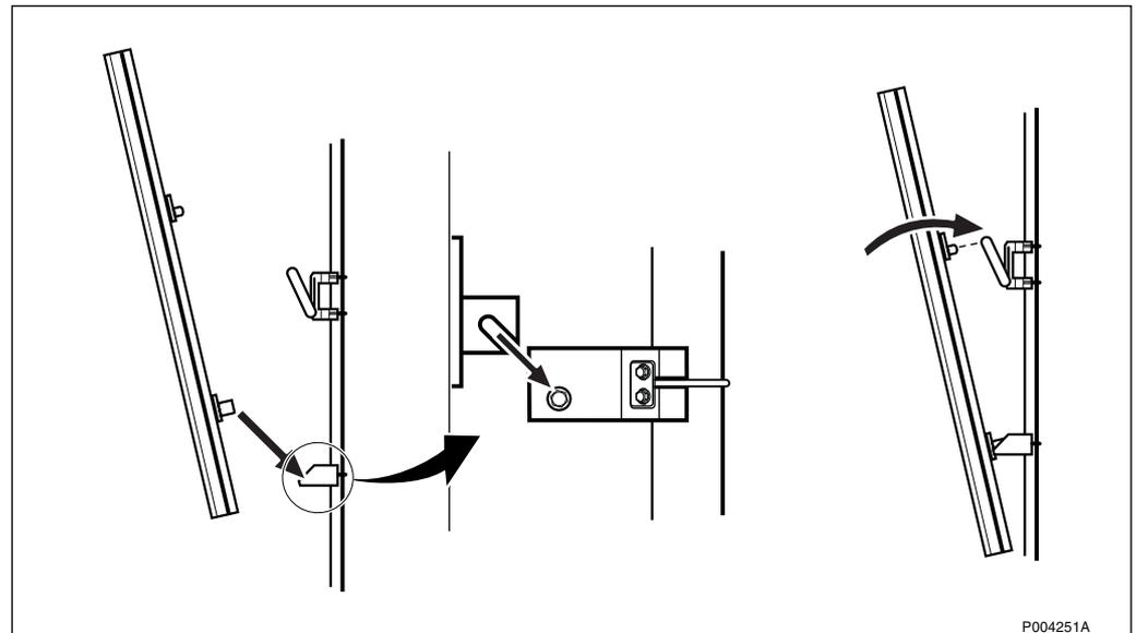
Figure 544 Sliding the antenna into the lower mount and tilt it up
