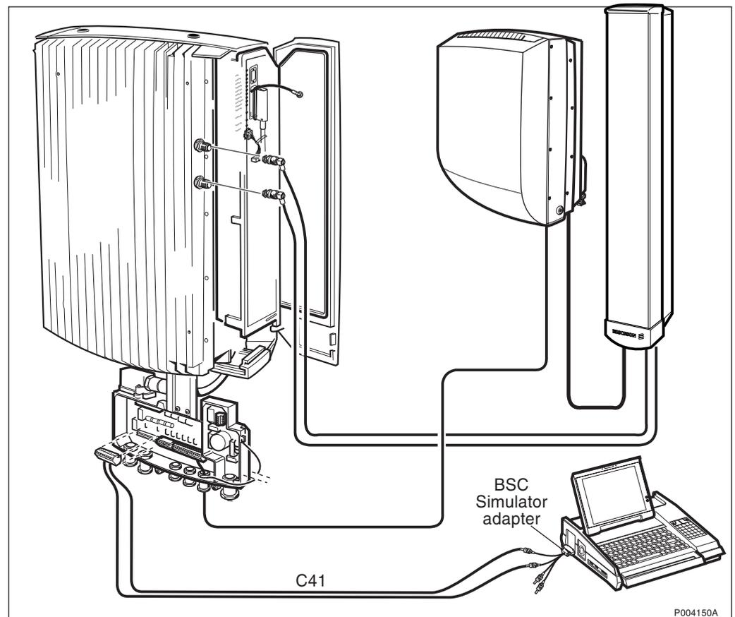
Figure 363 Test setup for GSM 1800 and GSM 1900: 2 TRX Sector Configuration for T1 100  $\Omega$  (1.5 Mbit/s) and E1 120  $\Omega$  (2.0 Mbit/s)
