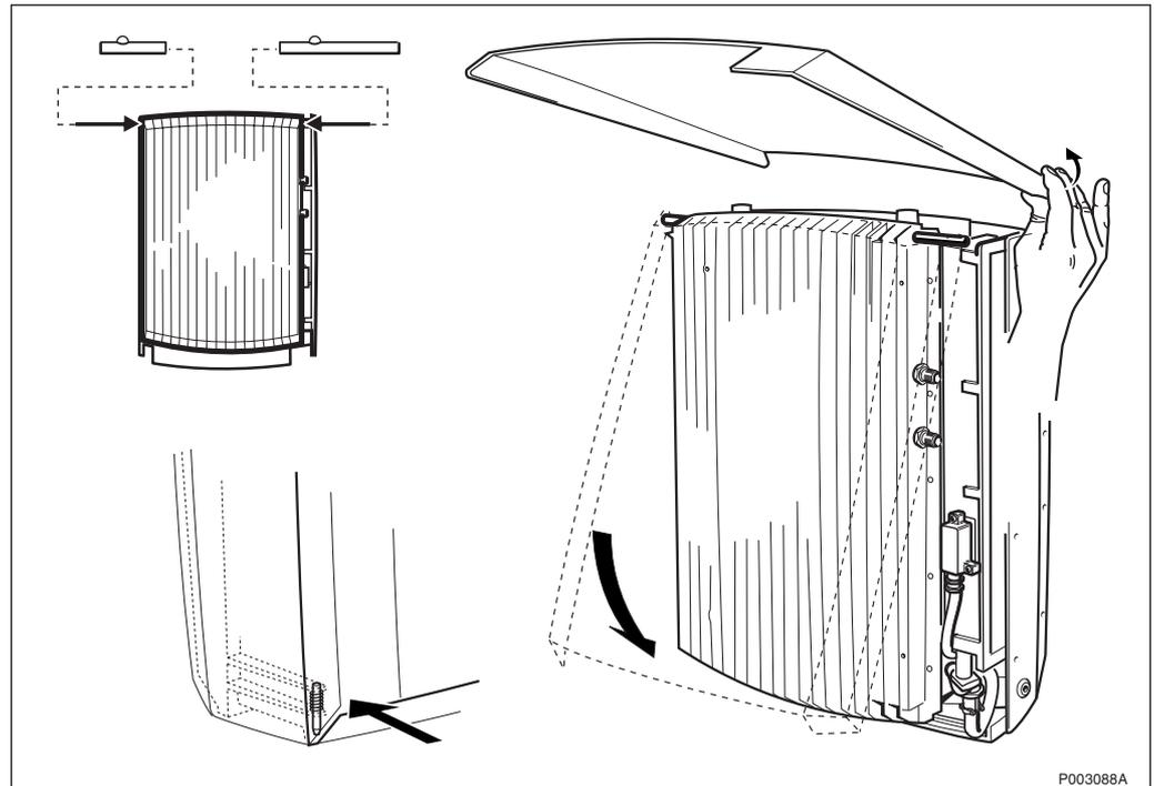
Figure 192 Mounting the front sunshield
