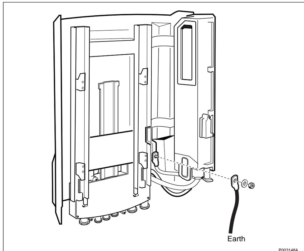
Figure 417 Removing the earth cable
