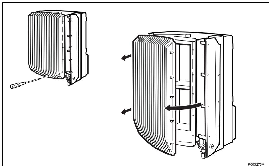
Figure 491 Opening the Battery cabinet door
