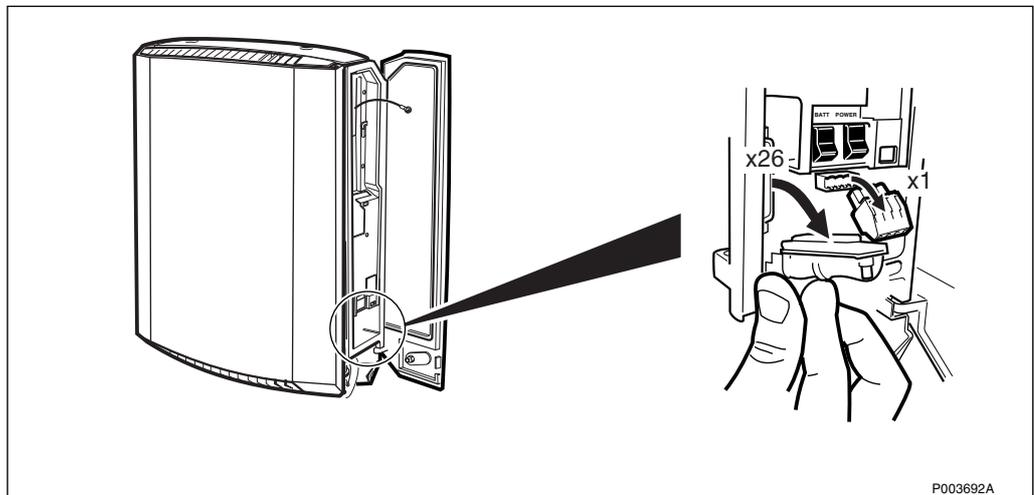
Figure 436 Disconnecting the transmission cable and AC cable
