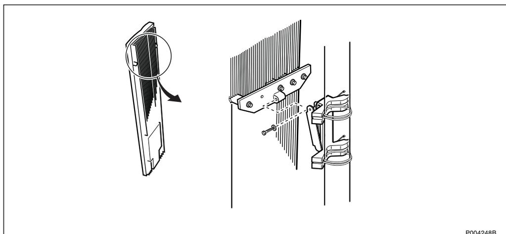
Figure 541 Unscrewing the screw on the upper mount
