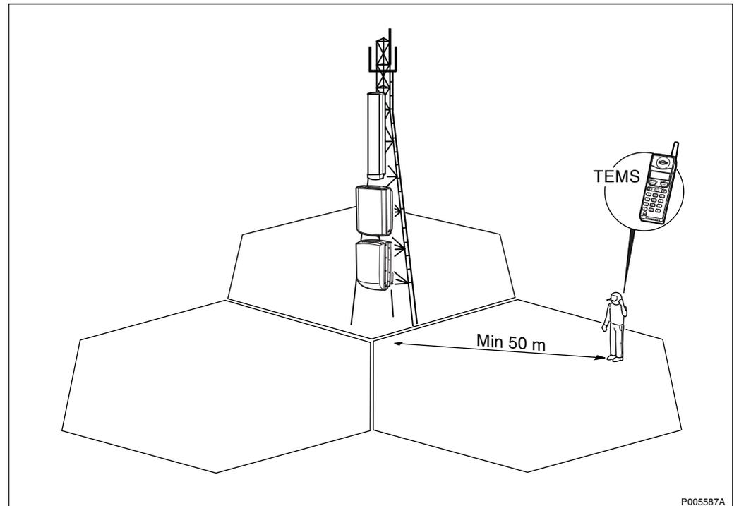
Figure 373 A forced handover test using the TEMS
