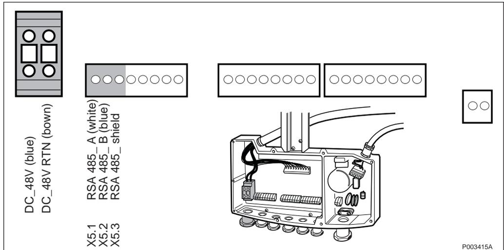
Figure 275 DC/Data termination block
