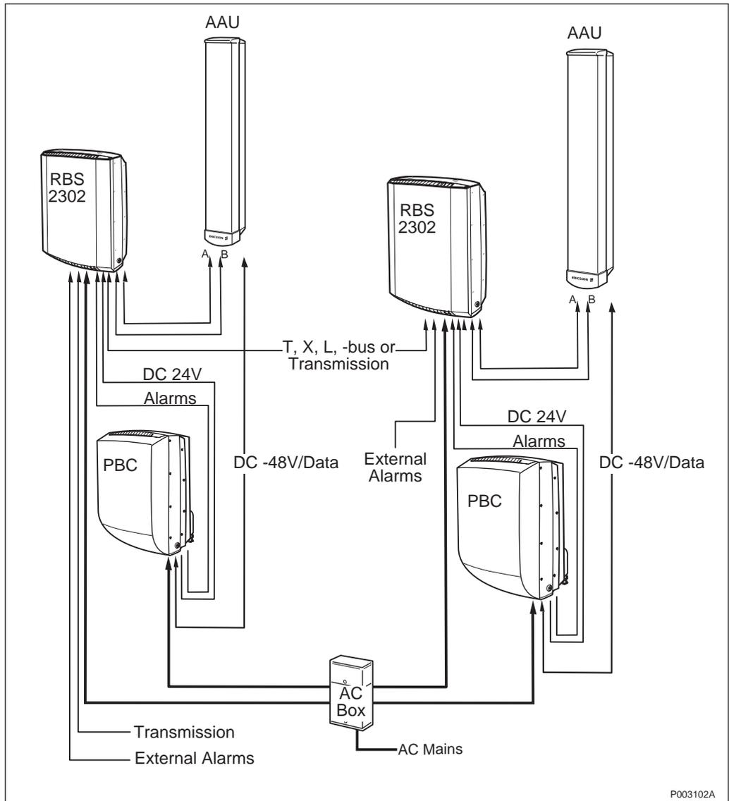
Figure 52 Configuration with 4 TRX
