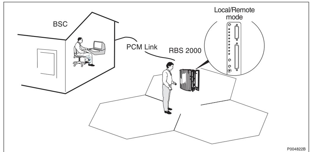
Figure 368 Integrating the BTS into the Network which is operated by the BSC
