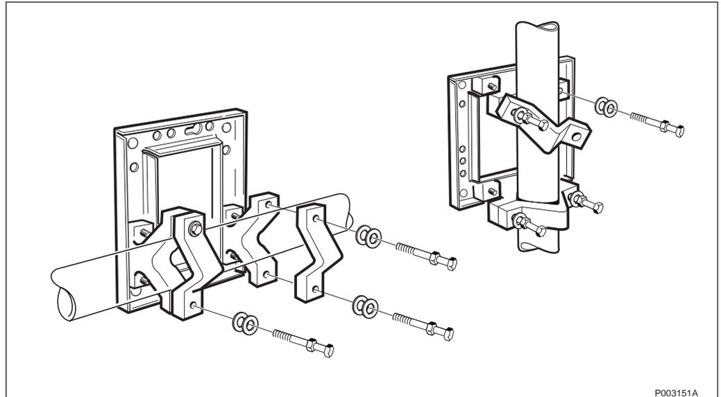
Figure 168 Placing the mounting plate correctly
