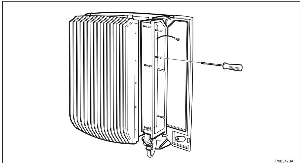
Figure 490 Loosening the installation box
