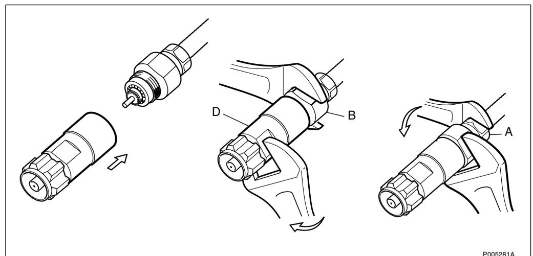
Figure 256 Mounting the connector head
