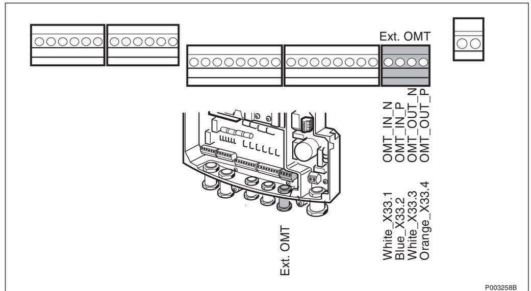
Figure 309 Extended OMT termination board (option)
