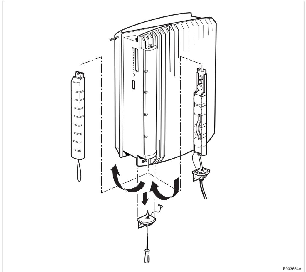
Figure 176 Switching the internal battery to the PSA
