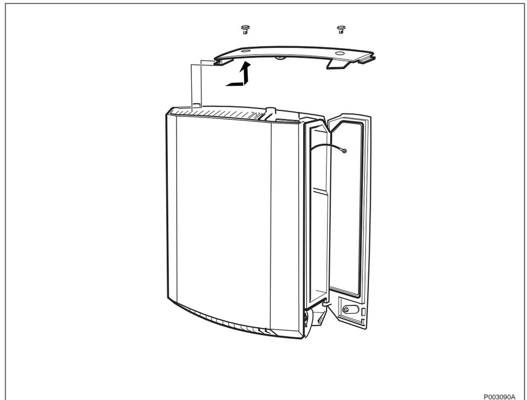
Figure 410 Replacing the upper sunshield
