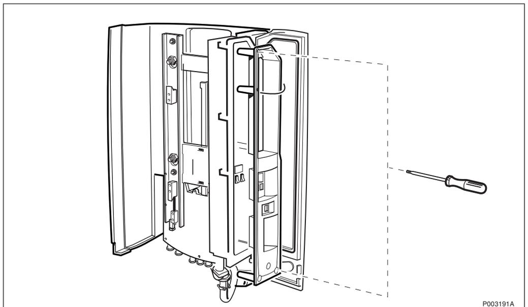
Figure 129 Removing the protection cover
