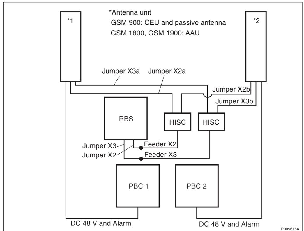
Figure 366 Jumper definition
