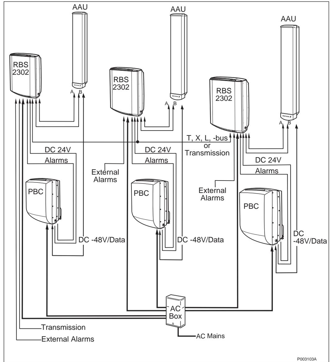
Figure 53 Configuration with 6 TRX
