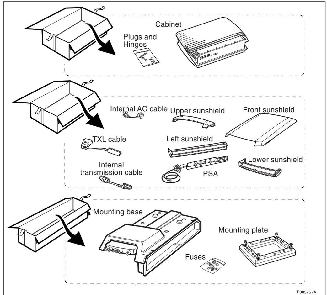
Figure 157 Unpacking the cabinet, sunshields and cables, and the mounting base
