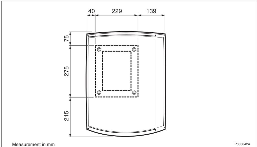
Figure 567 Mounting plate and equipment contour
