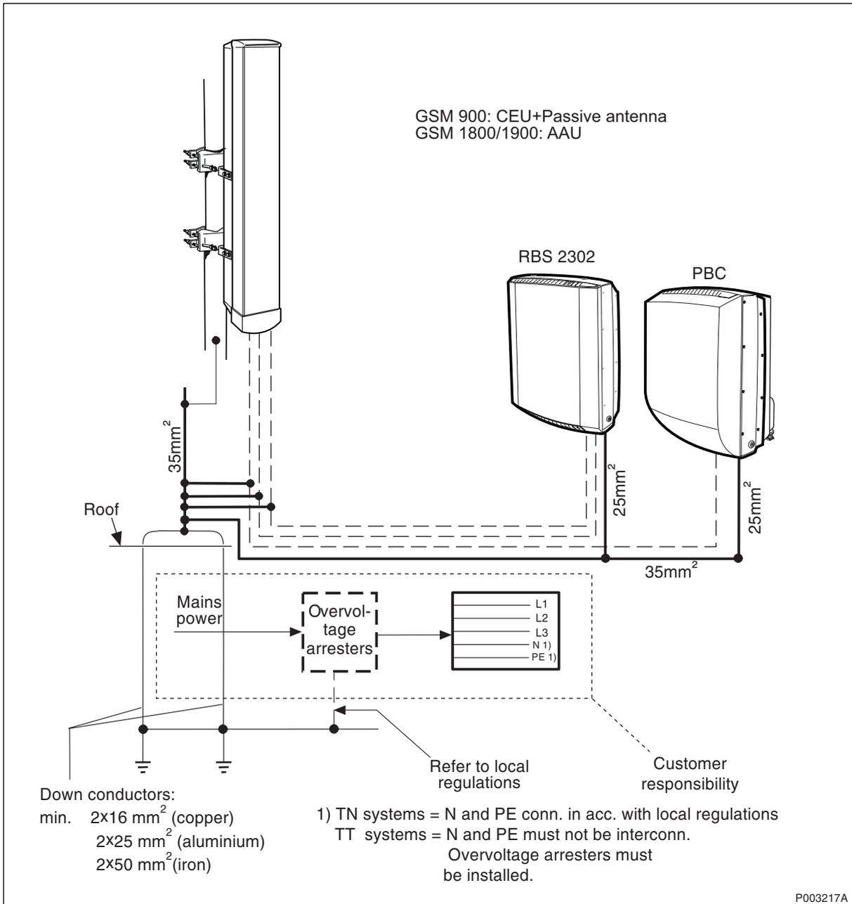
Figure 32 Block diagram outdoor earthing
