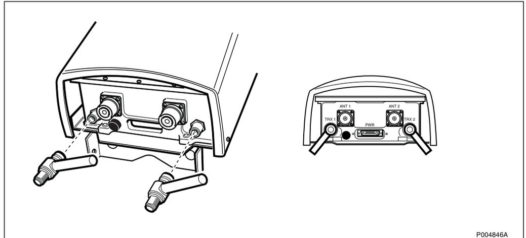
Figure 219 Connection of Lightning Protection
