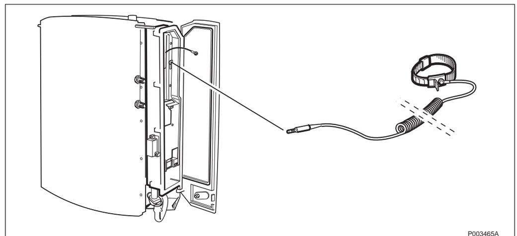
Figure 413 Connecting the ESD wrist strap
