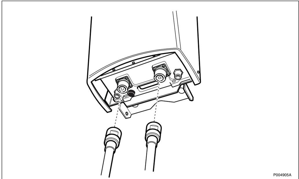
*Figure 221 Connection of the Antenna Jumper Cables*
