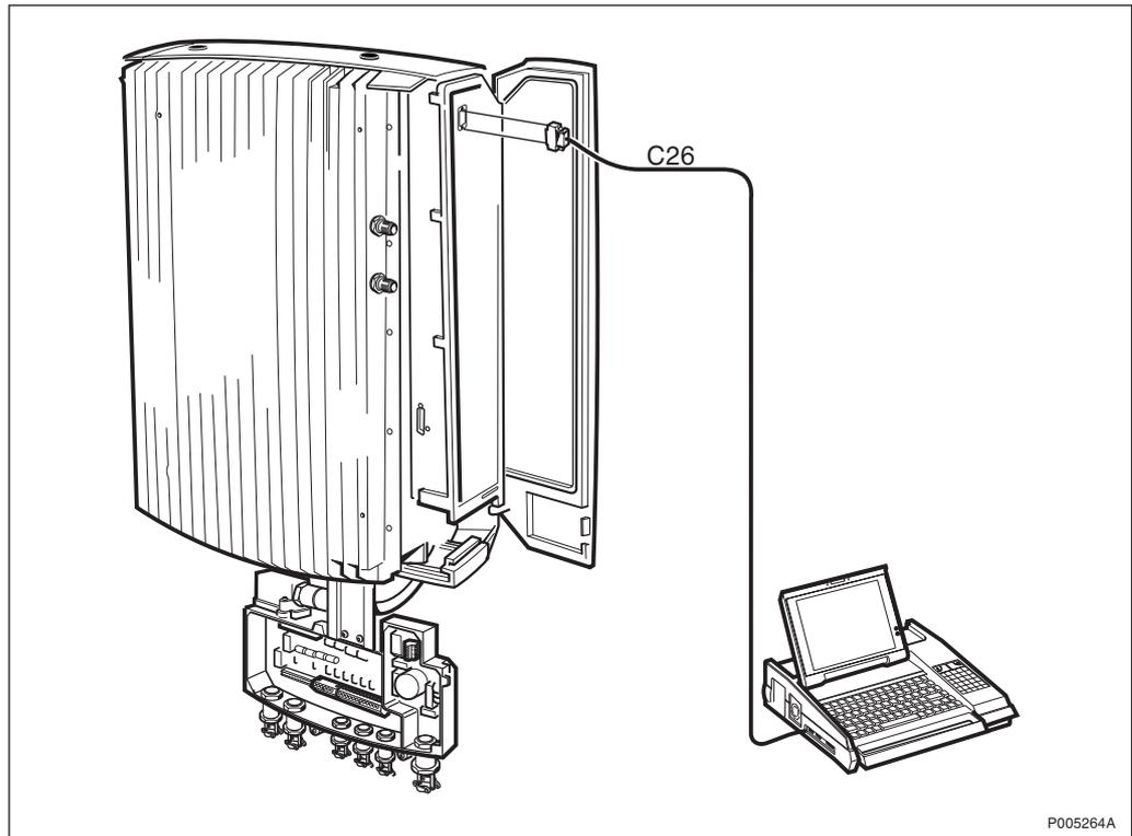
Figure 338 Connecting the OMT
