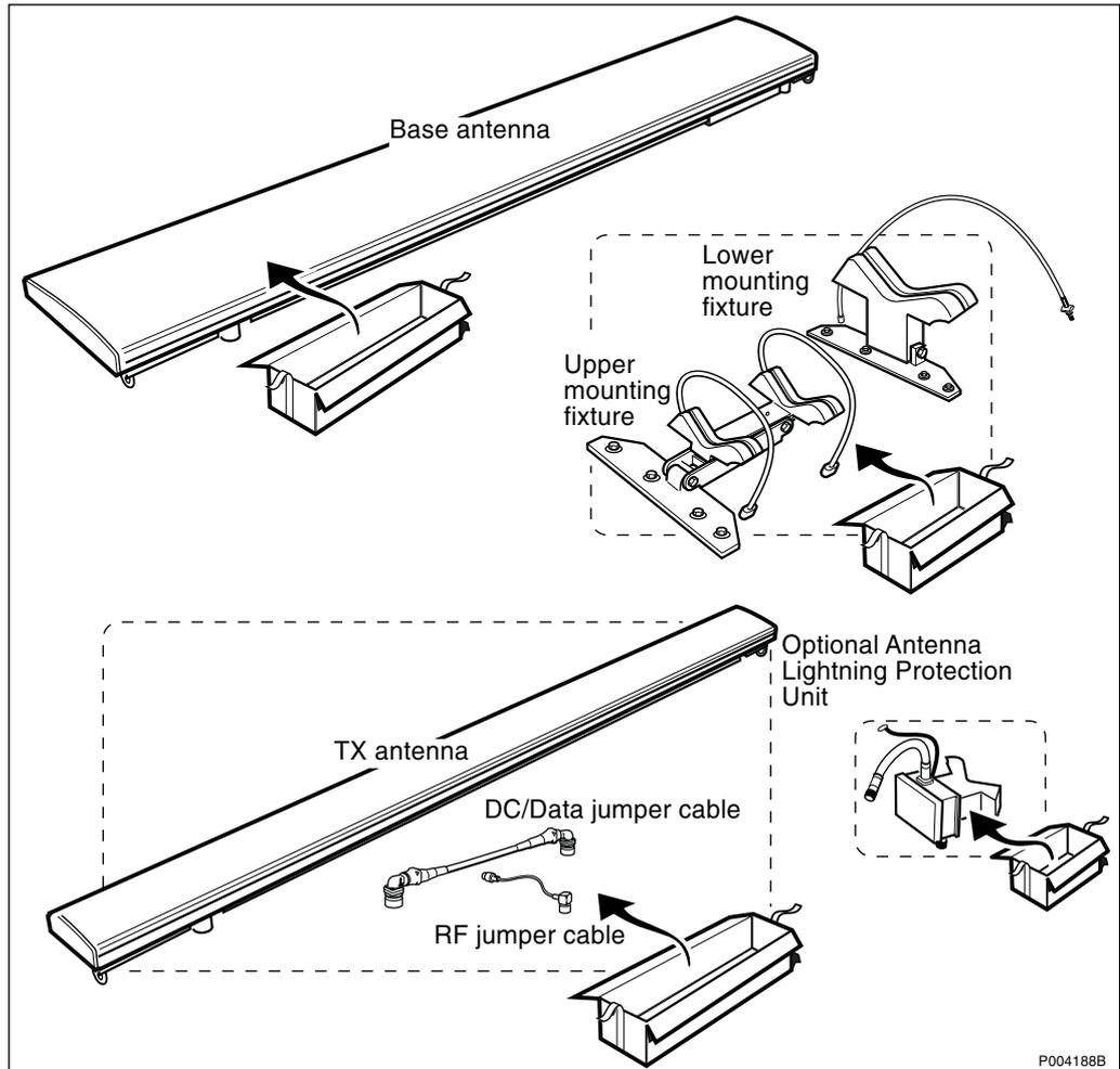
Figure 98 Contents of the AAU package for GSM 1900, 1250 W EIRP
