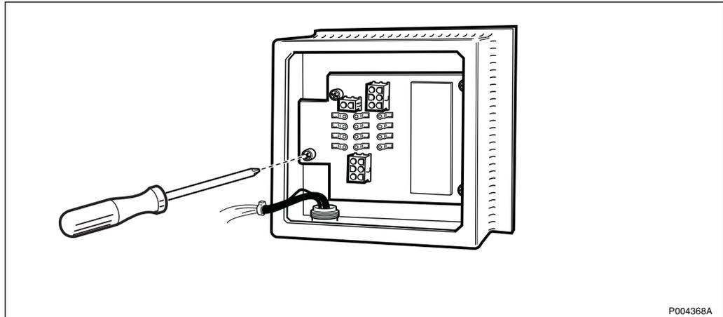
Figure 548 Removing the faulty board
