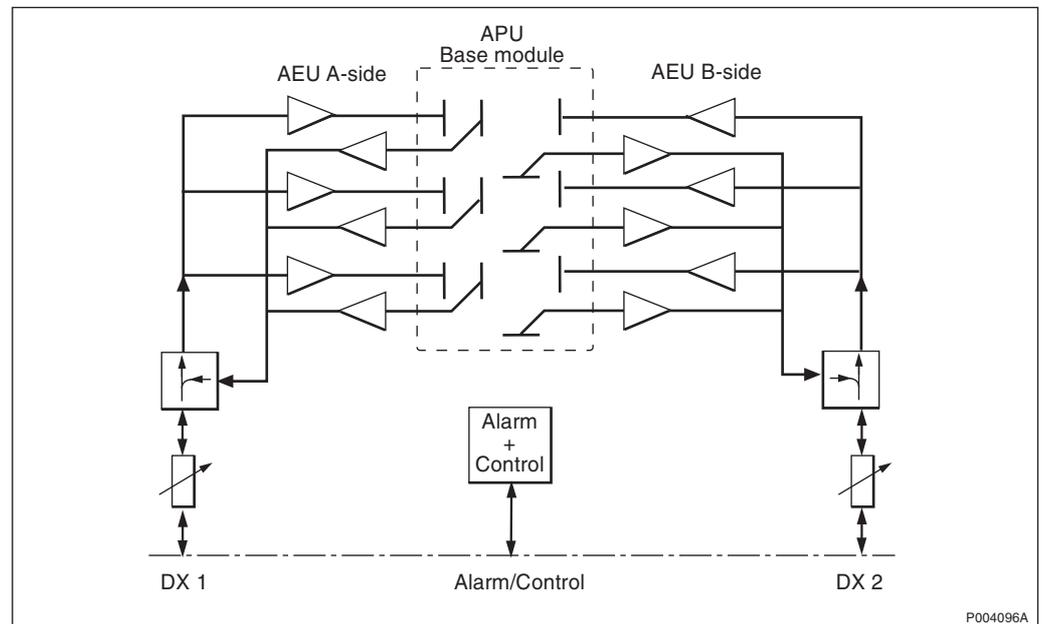
Figure 42 Block diagram Active Antenna Unit – 500 W EIRP for GSM 1900
