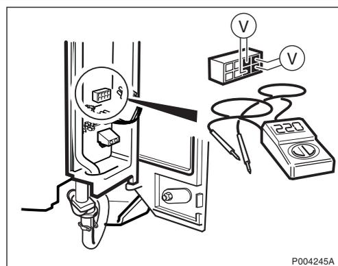
Measure that 155/230 V is present at the connector to the internal AC cable to verify that the EMC board is not faulty.
