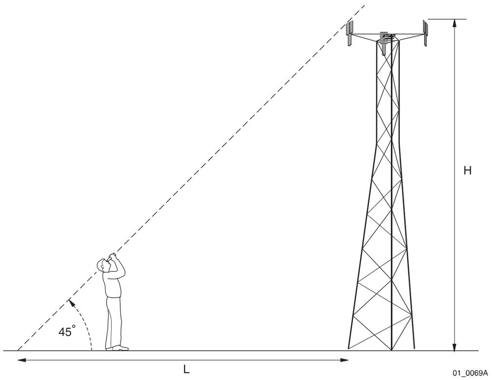
Figure 15 The 45° method of measuring a tower
