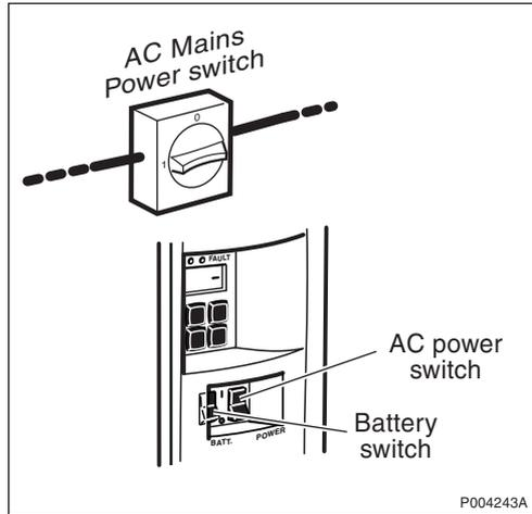
Confirm that the Mains switch is set to the ON position and that the AC switch on the PBC is set to the ON position.
