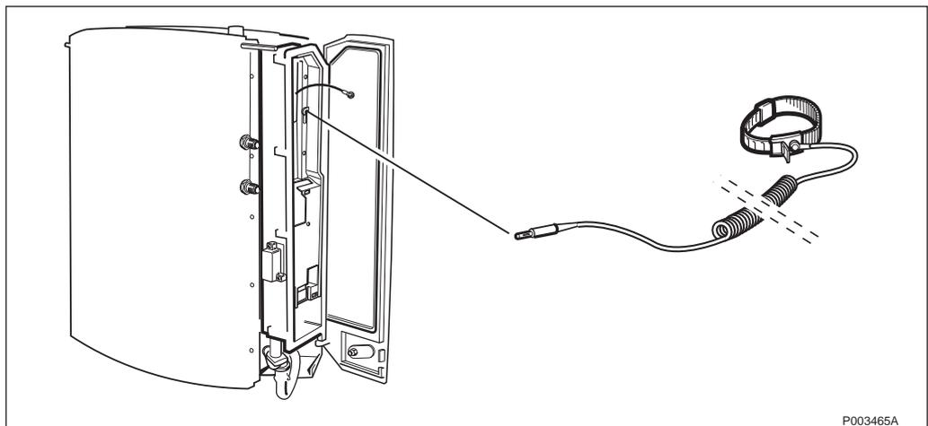
Figure 453 Connecting the ESD wrist strap
