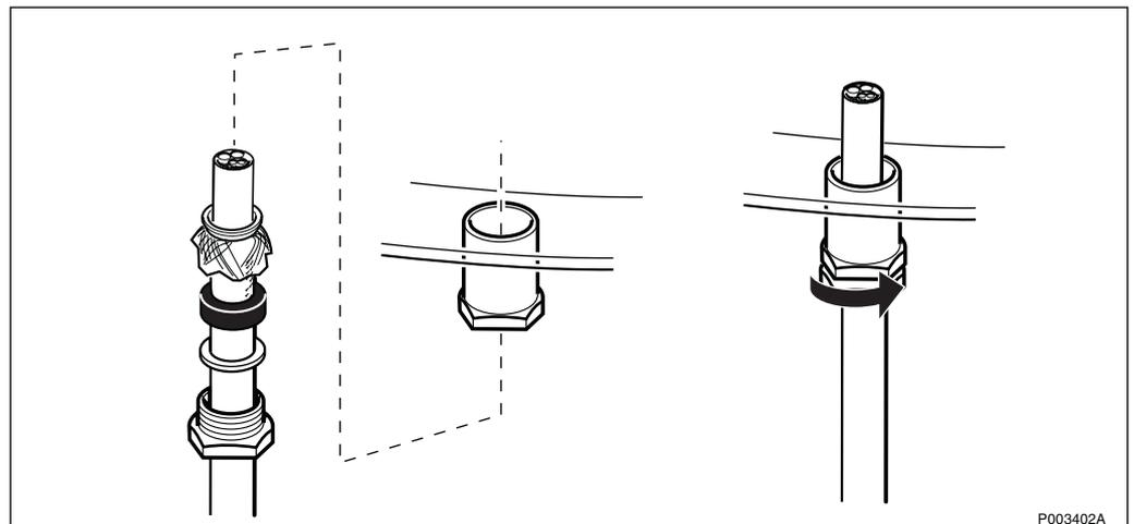
Figure 274 Mounting the cable inlet
