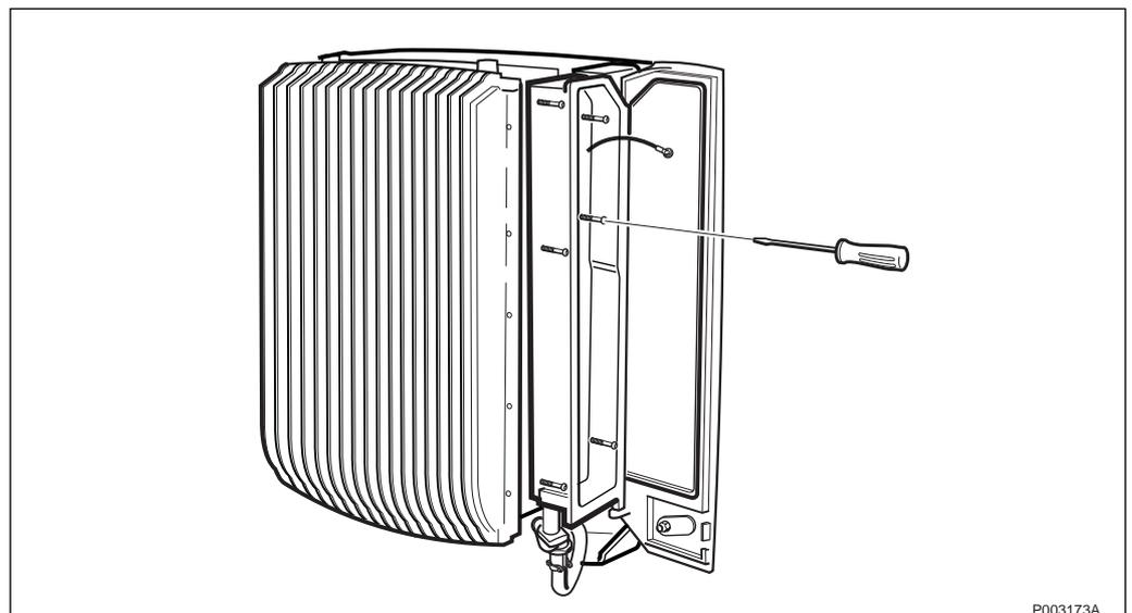
Figure 136 Fastening the installation box
