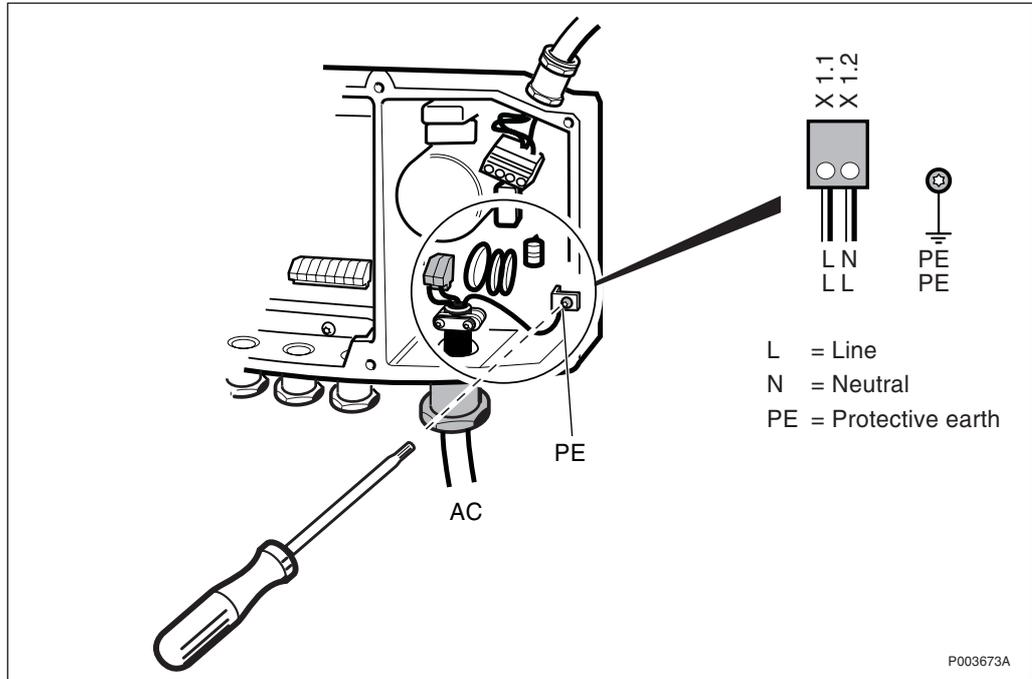
Figure 272 AC Mains power section in the interface box
