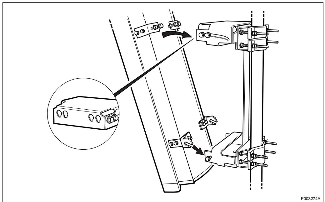
Figure 88 Attaching the antenna to the mounting fixture
