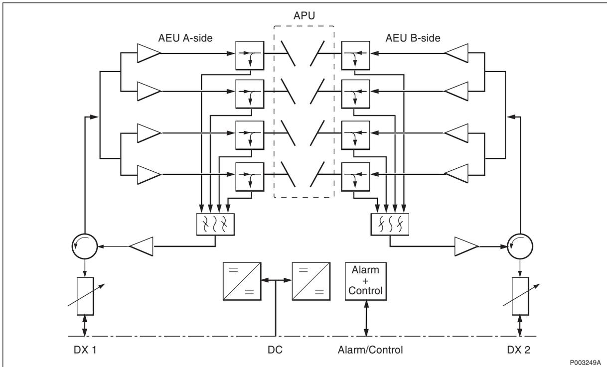
Figure 41 Block diagram Active Antenna Unit – 500 W EIRP for GSM 1800
