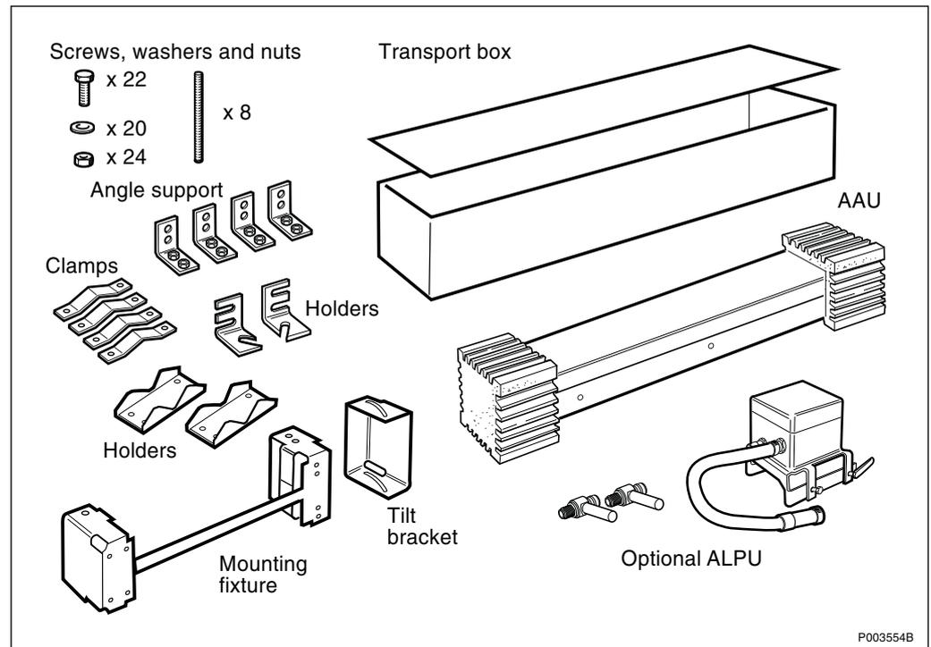
Figure 79 Contents of the antenna package
