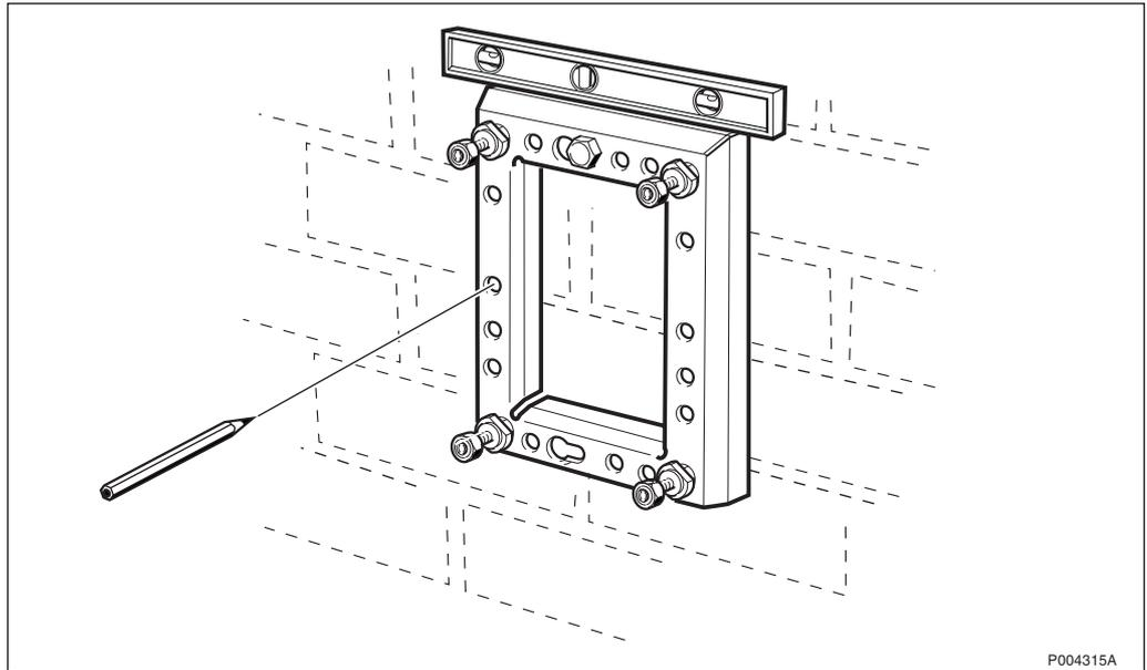
Figure 118 Marking the rest of the holes
