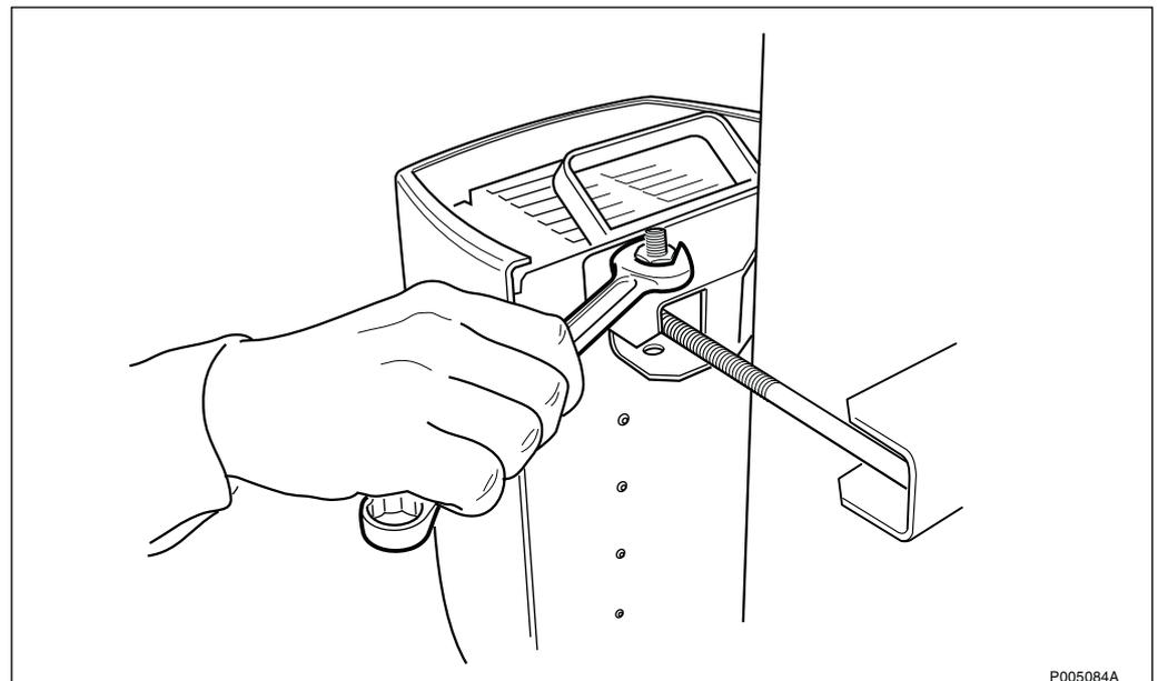
Figure 65 Fastening the CEU to the upper mounting fixture
