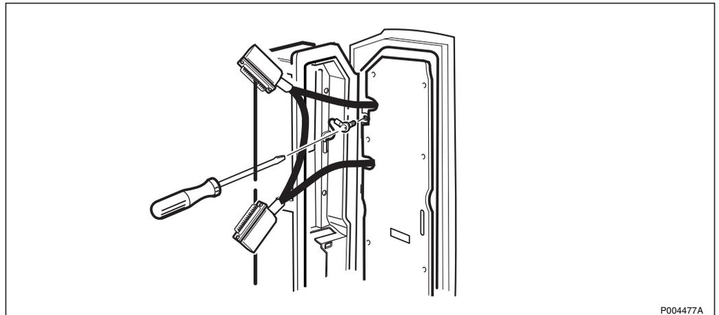
Figure 173 Mounting the earth cable, Installation Box Door with HDSL
