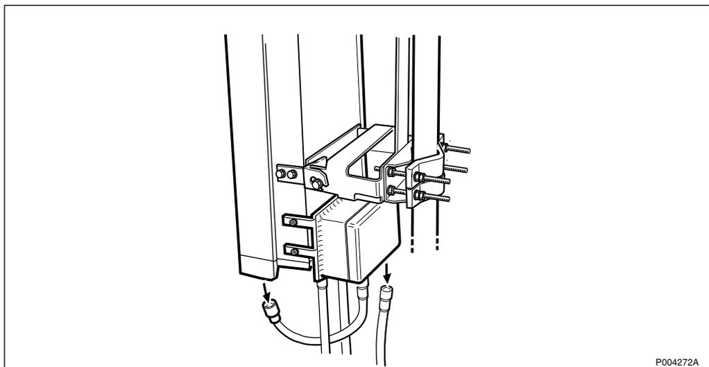
Figure 528 *Disconnecting the cables*
