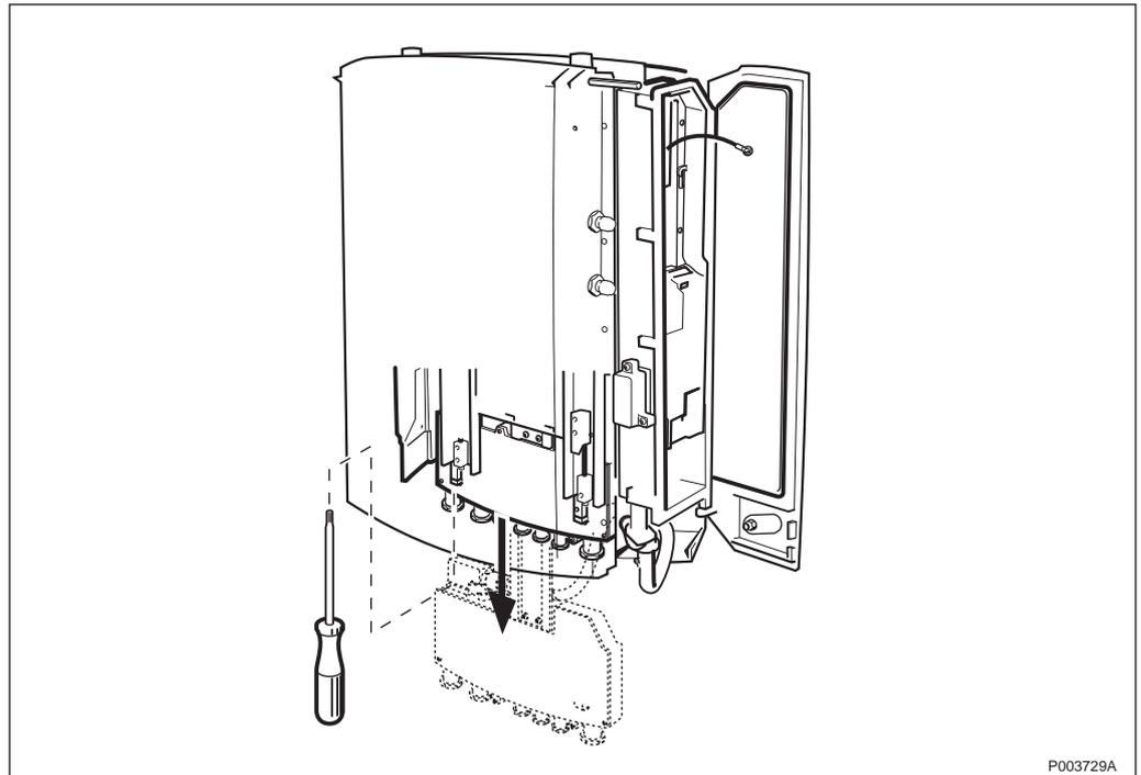
Figure 281 Pulling down the interface box
