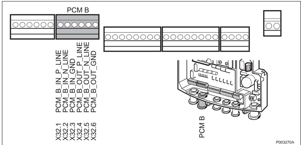
Figure 293 Connecting PCM B to the termination block (Cascade connection)
