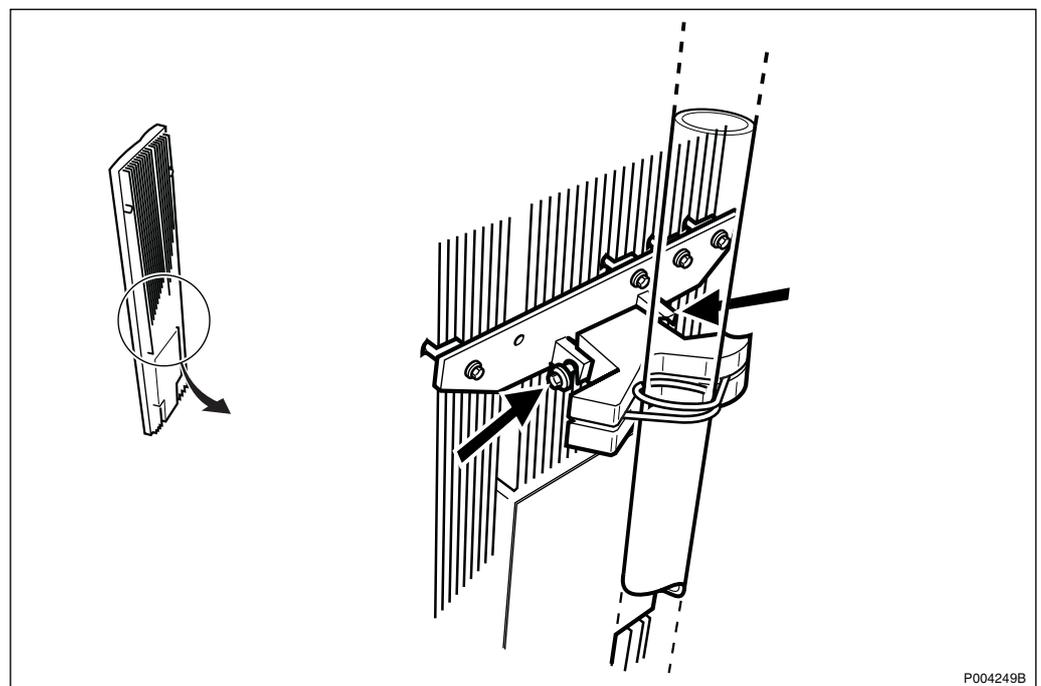
Figure 545 Tightening the two screws on the lower mount
