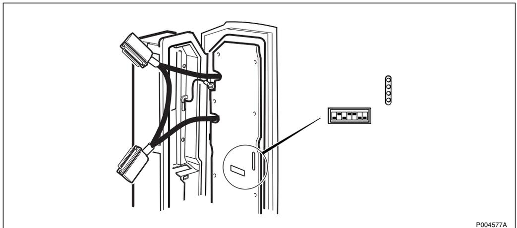
Figure 405 Position of the DIP switches
