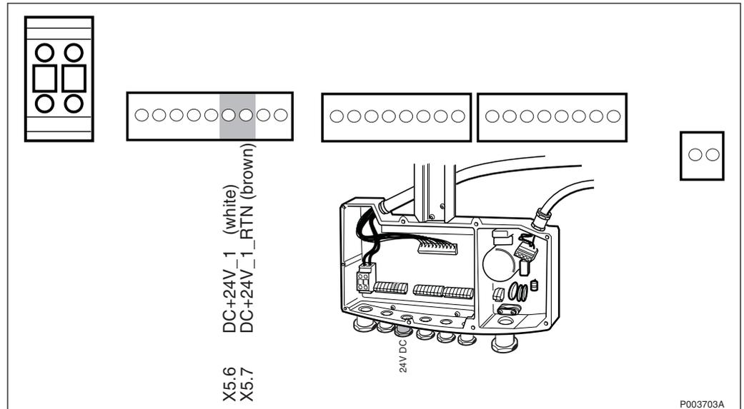
Figure 276 PSA termination block
