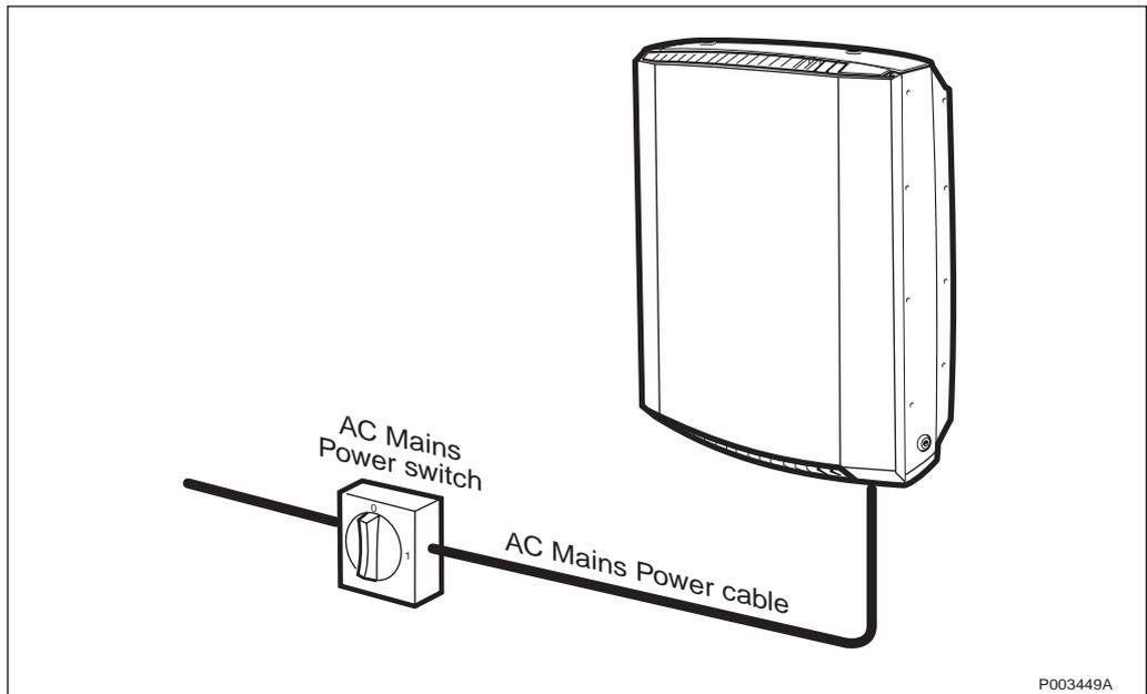
Figure 396 AC mains power switch turned off
