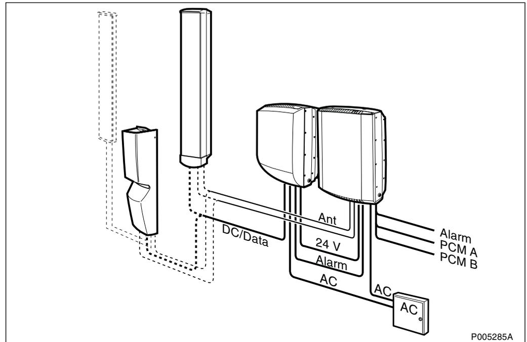
Figure 211 Basic Maxite configurations with Active Antenna Unit (AAU) or Coverage Extension Unit (CEU)
