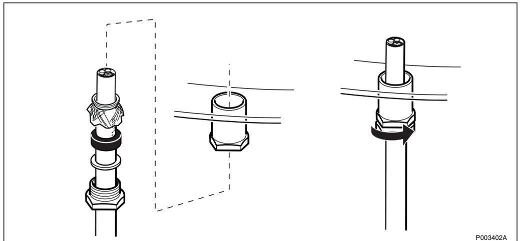
Figure 289 Mounting the cable inlet
