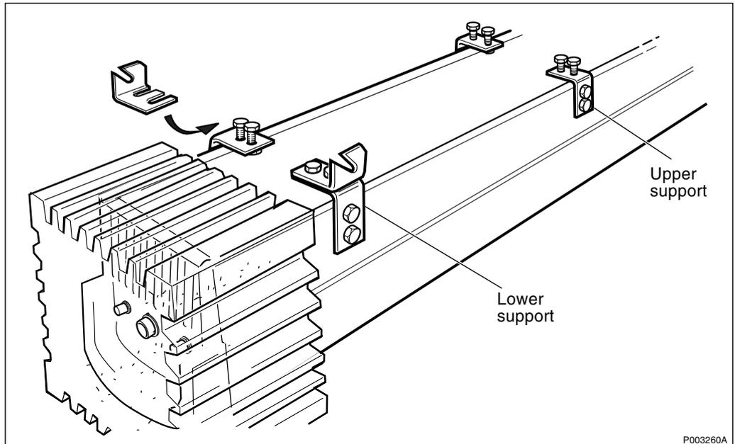
Figure 82 Attaching the two holders to the lower angle supports
