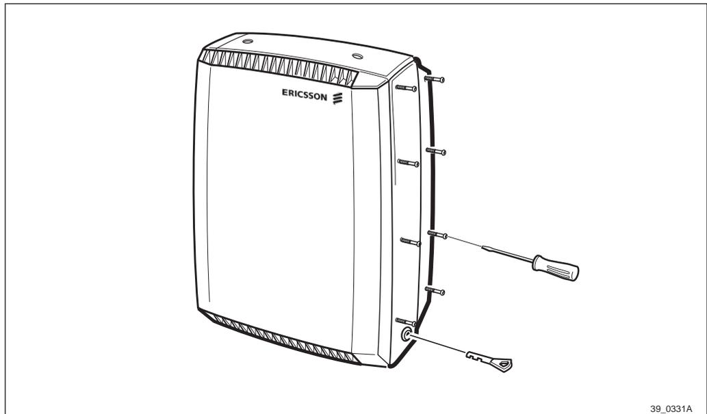
Figure 316 Sealing screws and key for the installation box door
