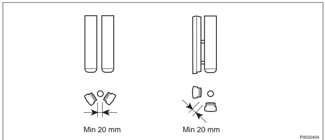
Figure 19 Antennas in different cells
