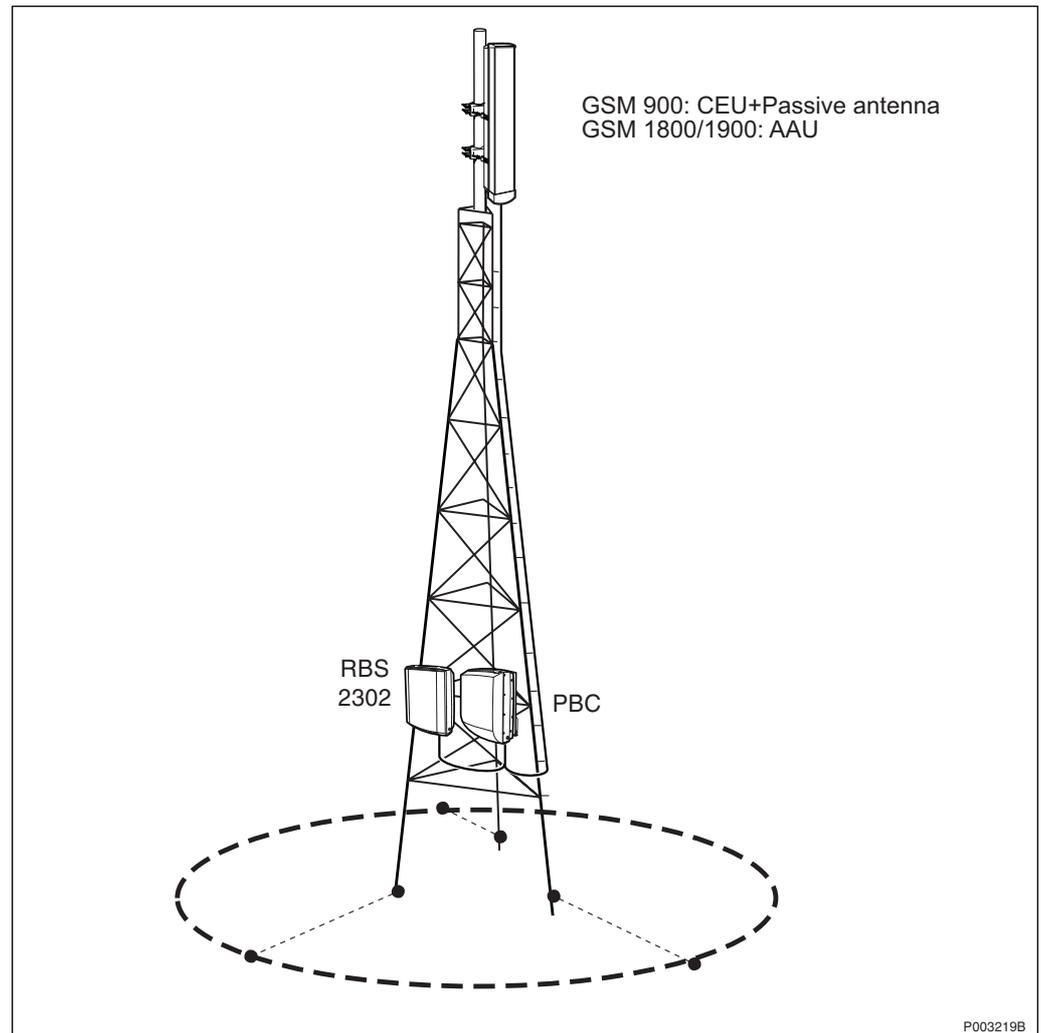
Figure 31 Typical ring earth electrode arrangement on ground
