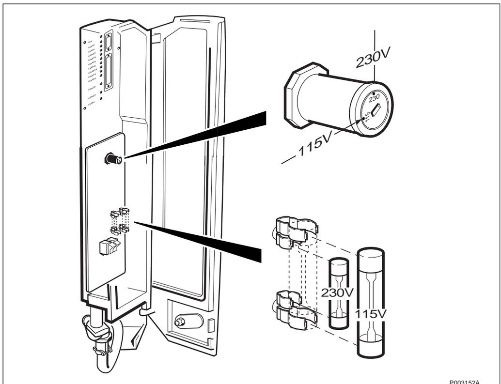
Figure 175 Installing the fuses and checking the voltage selector
