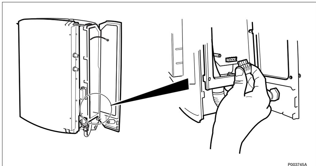
Figure 508 Disconnecting the AC cable
