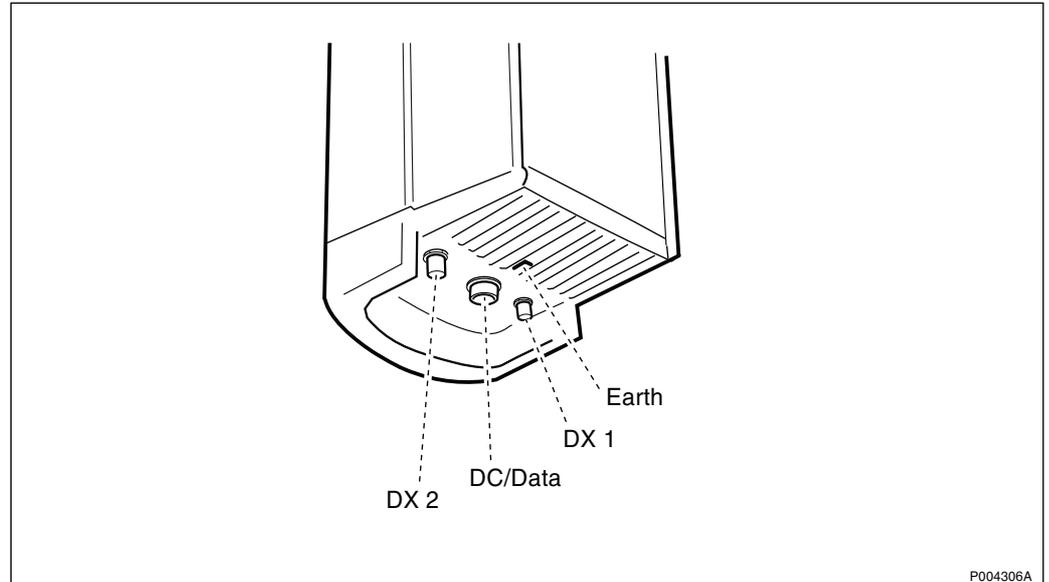
Figure 226 Connection overview of the GSM 1800 antenna 500 W EIRP
