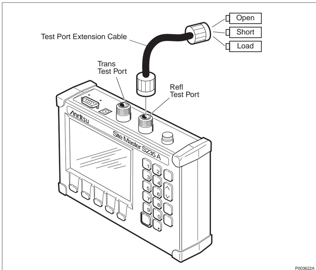
Figure 329 Different connections for calibration
