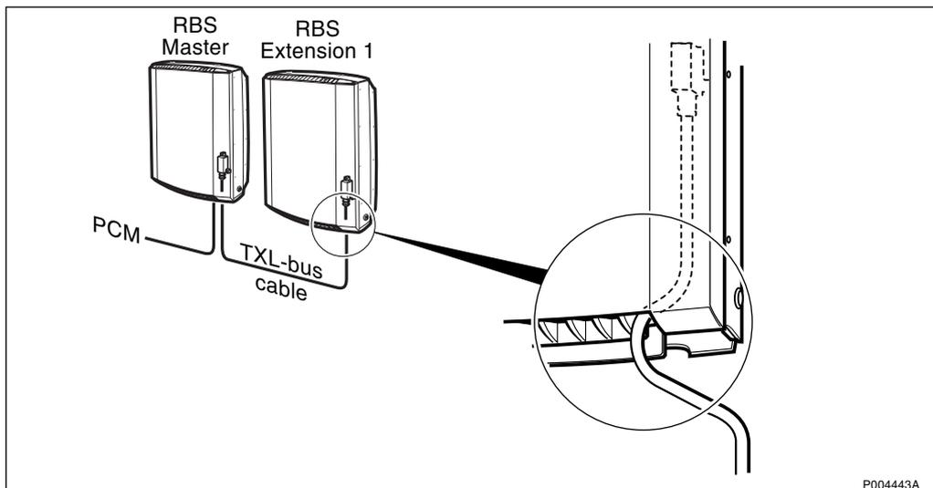
Figure 314 TXL-bus connection for 4 TRX configuration
