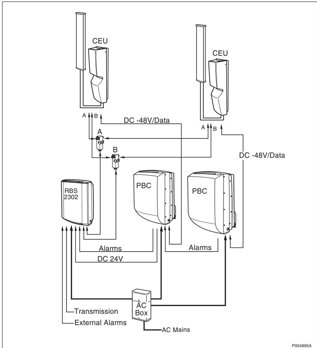
Figure 50 Highway configuration
