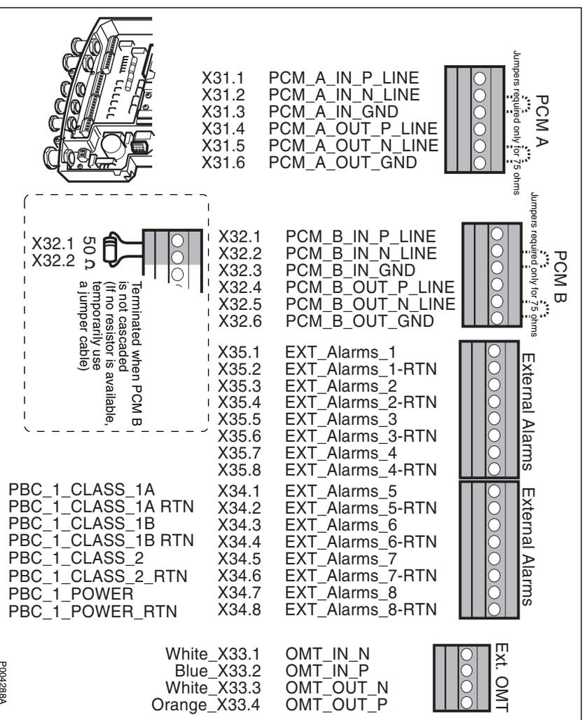
Figure 400 Cable connections for RBS 2302
