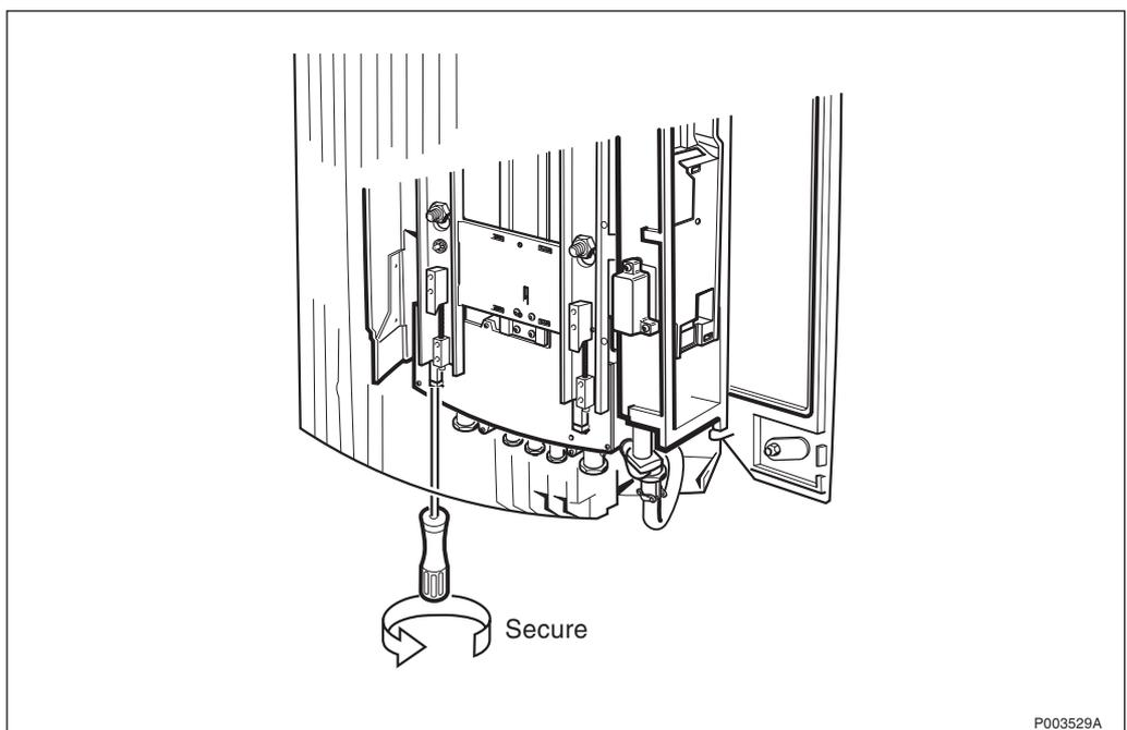
Figure 181 Securing the cabinet
