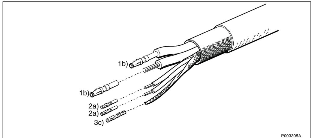
*Figure 233 Crimping the contact pin*
