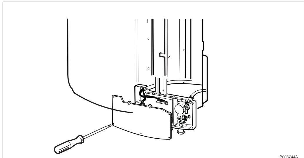
Figure 266 Loosening the interface box cover
