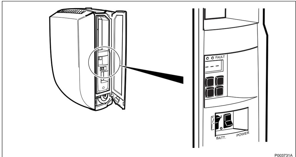
Figure 470 Battery switch
