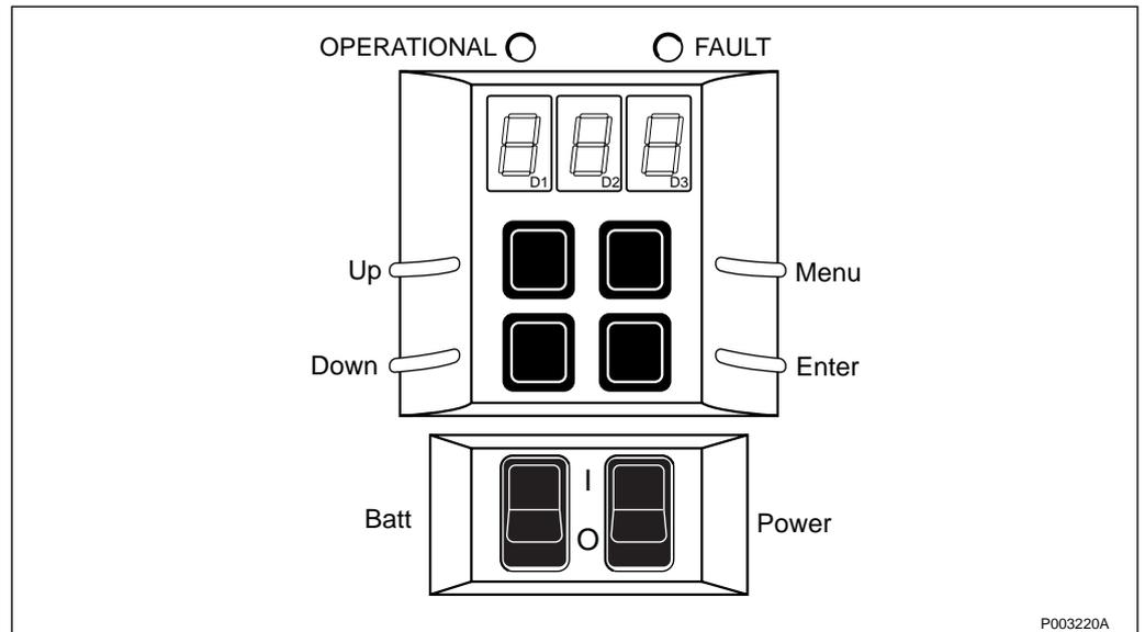
Figure 320 PBC control panel
