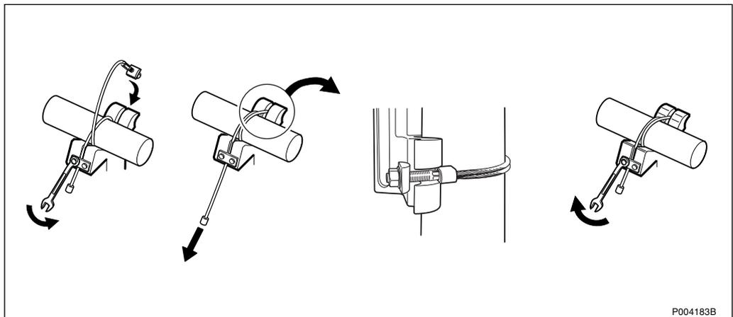
Figure 103 Loosening the locking plate and adjusting the harness cable
