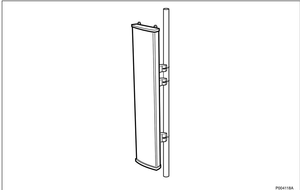
Figure 95 Antenna 500 W EIRP mounted on a pole
