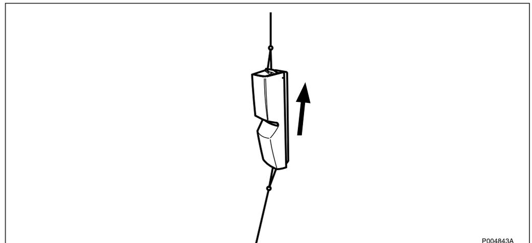
Figure 62 Using the control rope to control the CEU when hoisted
