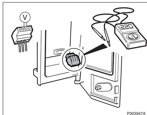
Measure that 155/230 V is present at the incoming AC plinth on the EMC board to verify that the cables are not faulty.
