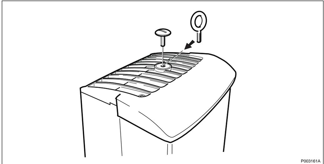
Figure 522 Mounting the lift eye on top on the AAU
