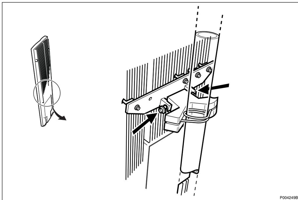
Figure 540 Releasing the two screws on the lower mount
