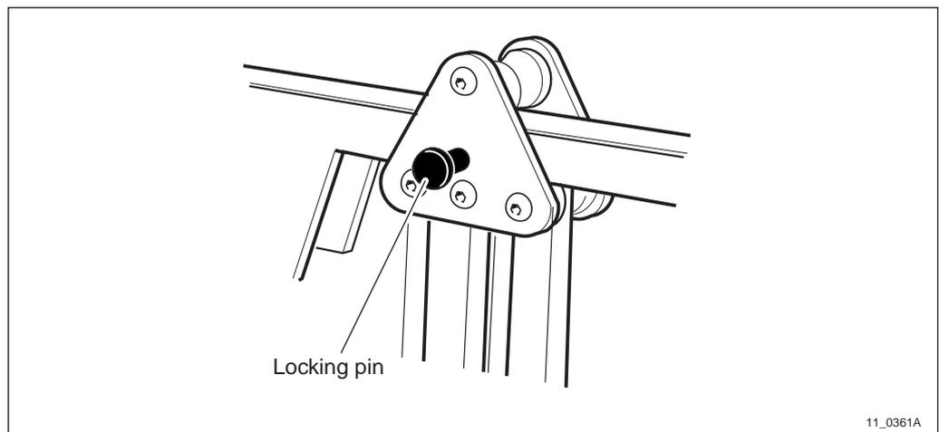
Figure 205 Releasing the trolley
