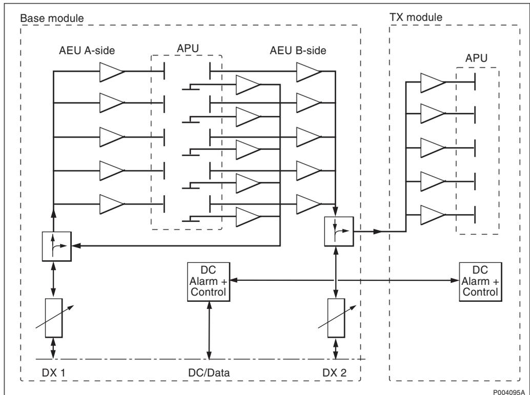
Figure 43 Block diagram Active Antenna Unit – 1250 W EIRP for GSM 1900
