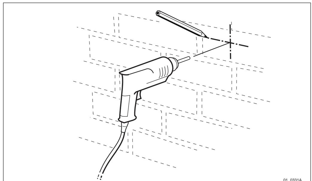
Figure 161 Marking the position of the mounting plate and drilling the hole
