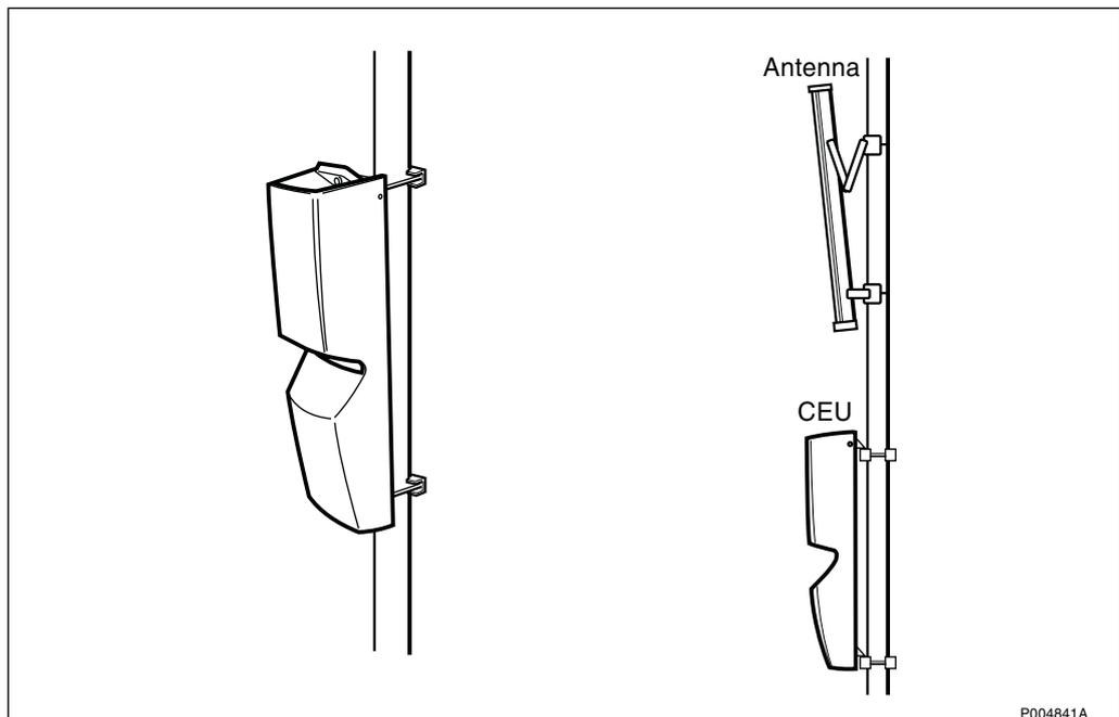
*Figure 55 The CEU mounted on a pole*
