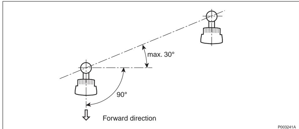
Figure 20 Directions not perpendicular to the mounting structure
