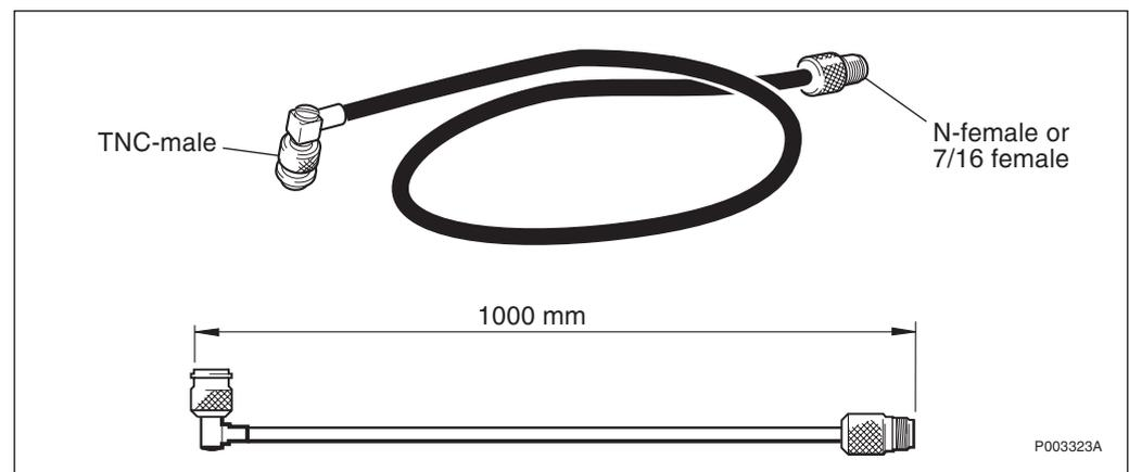
Figure 560 Jumper Cable
