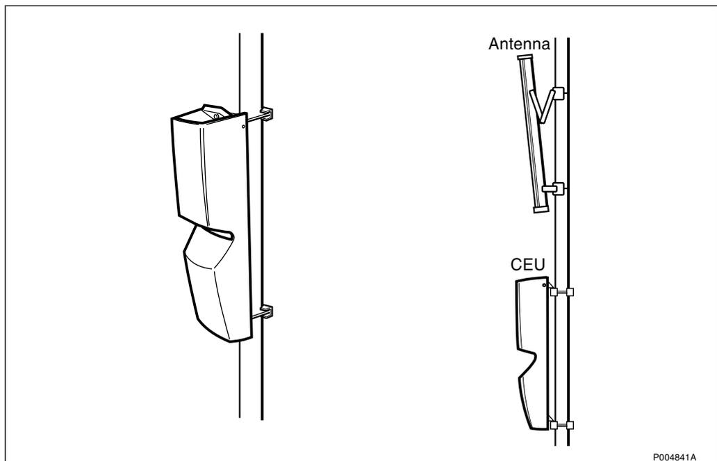
Figure 569 CEU mounted on a pole
