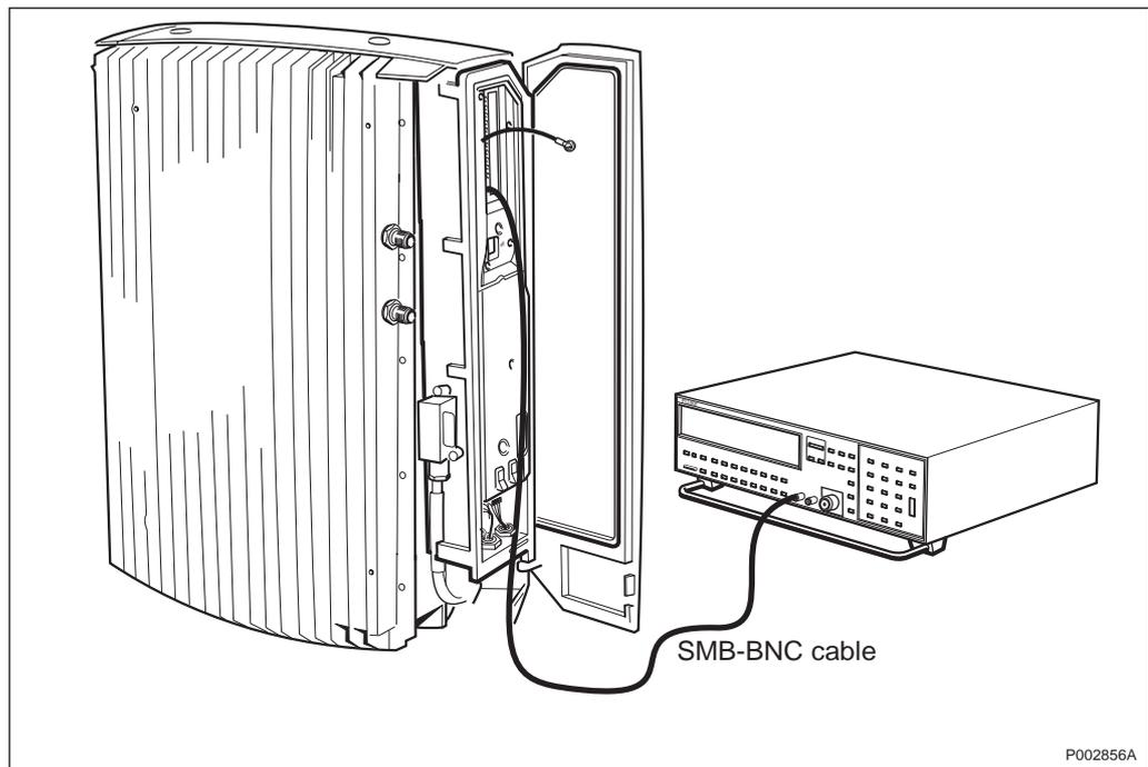
Figure 549 Calibrating the Radio cabinet
