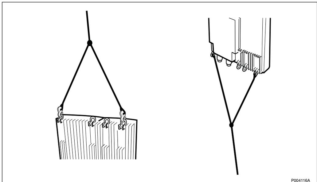
Figure 539 Securing the antenna in the lifting eyes
