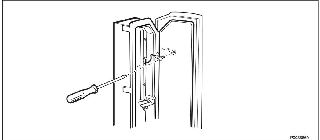
Figure 172 Mounting the earth cable, Installation Box Door without HDSL
