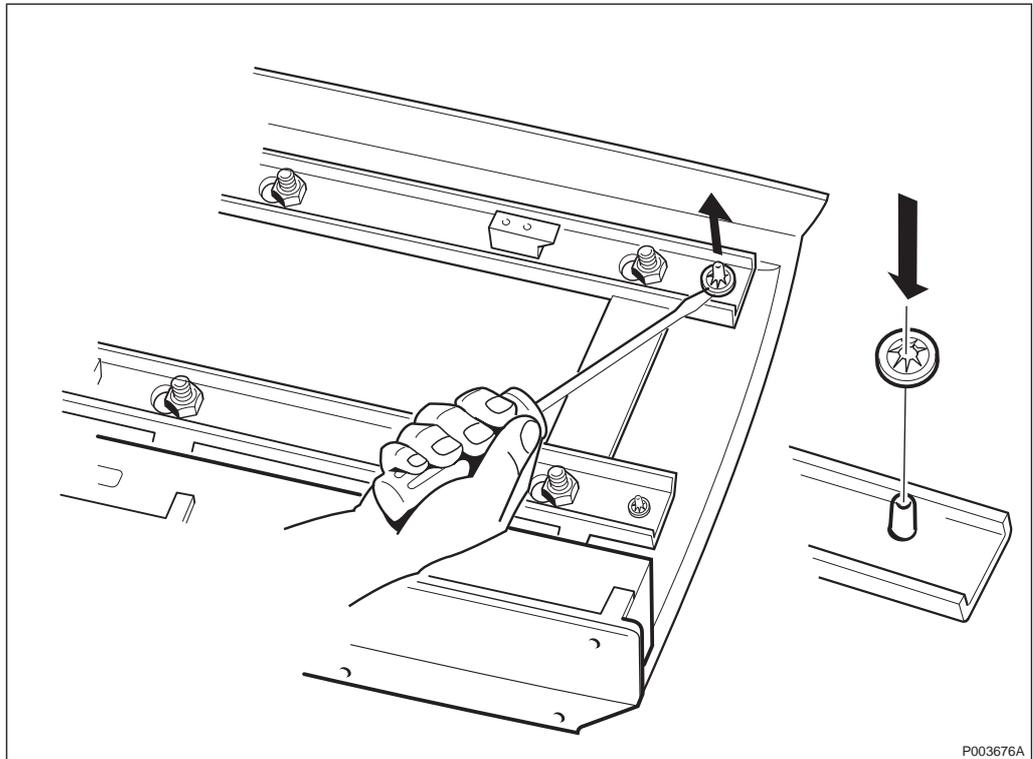
Figure 418 Removing locking washers
