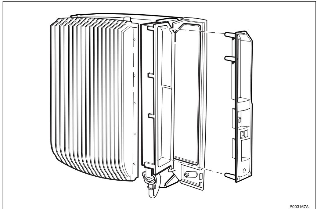
Figure 505 Removing the protective cover
