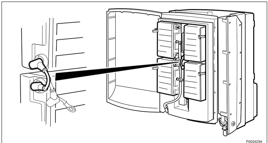
Figure 146 Connecting battery 3 and 4
