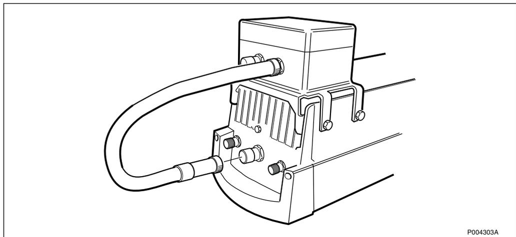
Figure 93 Tightening the screws and connecting the DC/Data jumper cable
