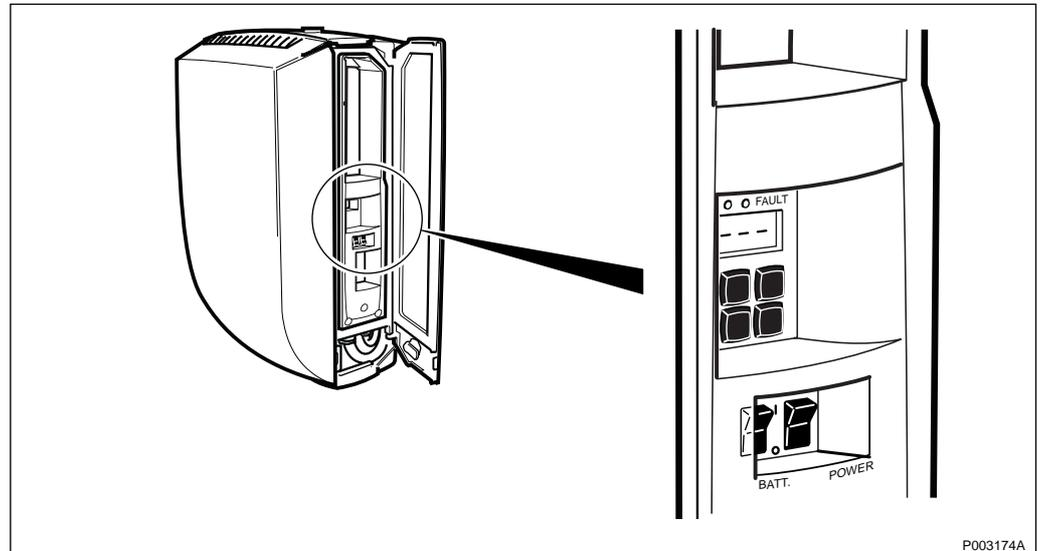
Figure 395 Battery and AC switch in the PBC
