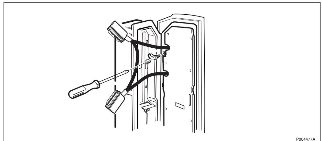
Figure 403 Disconnecting the Protective Earth
