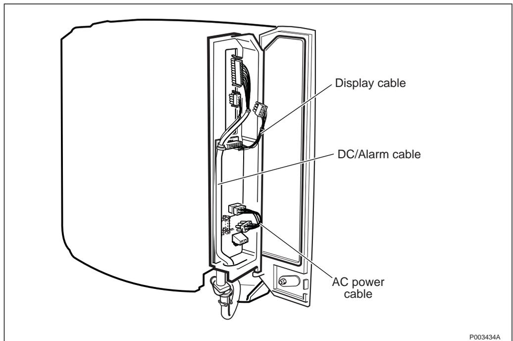
Figure 138 Connecting internal cables
