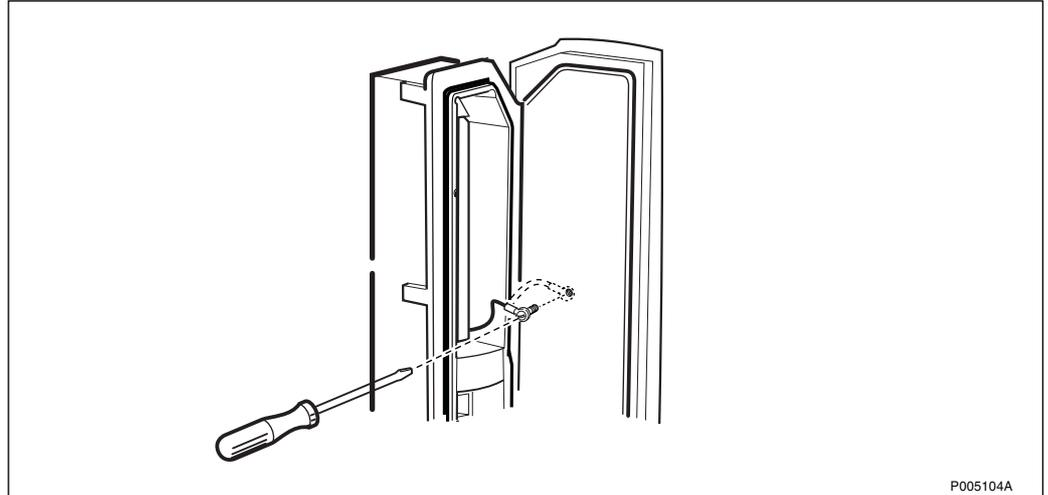
Figure 128 Mounting the earth cable
