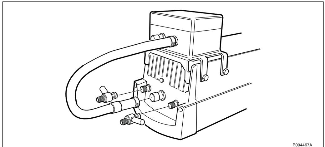
Figure 94 Mounting the RF lightning protectors
