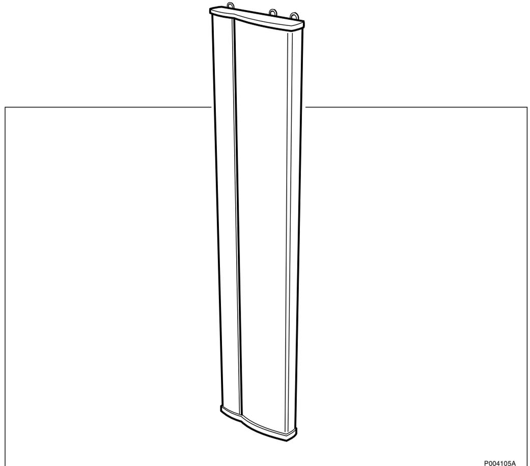
Figure 583 Active Antenna Unit 1250 W EIRP for GSM 1900
