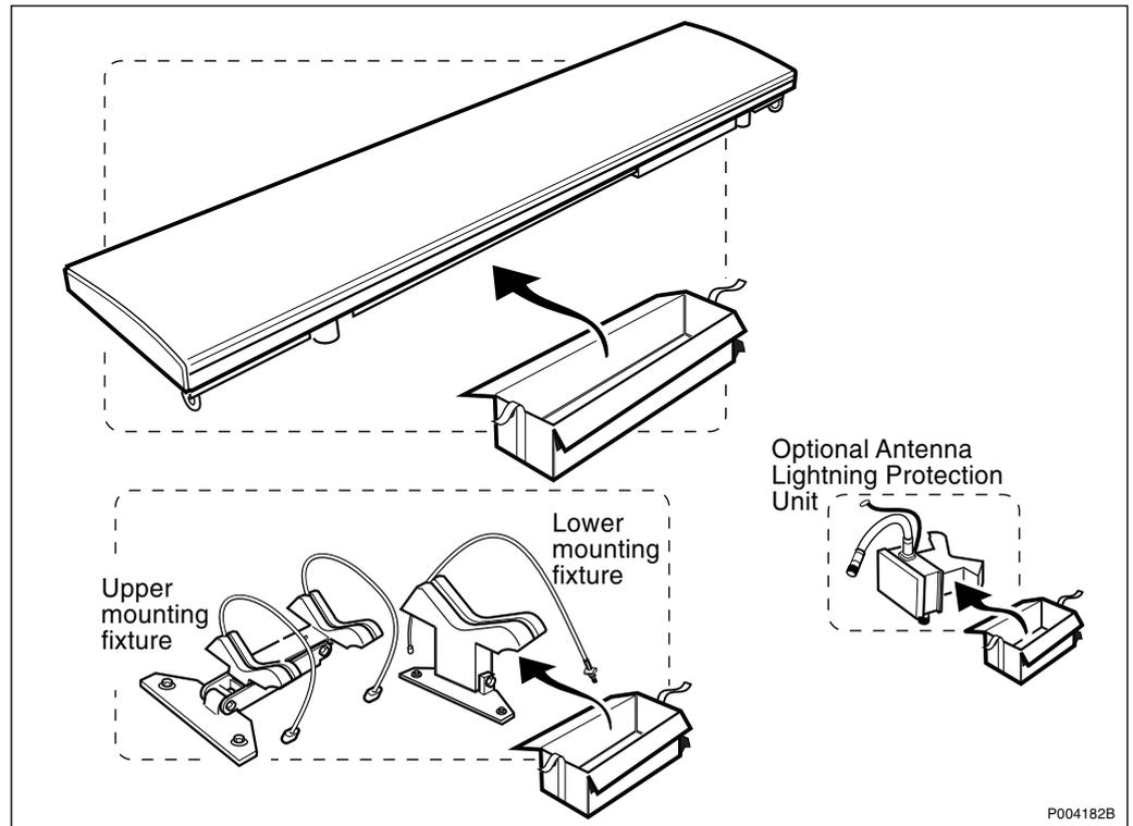
Figure 97 Contents of the AAU package for GSM 1900, 500 W EIRP
