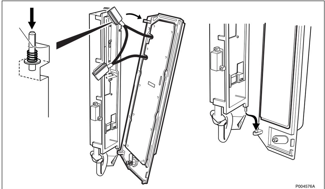
Figure 404 Dismantling the faulty HDSL Modem
