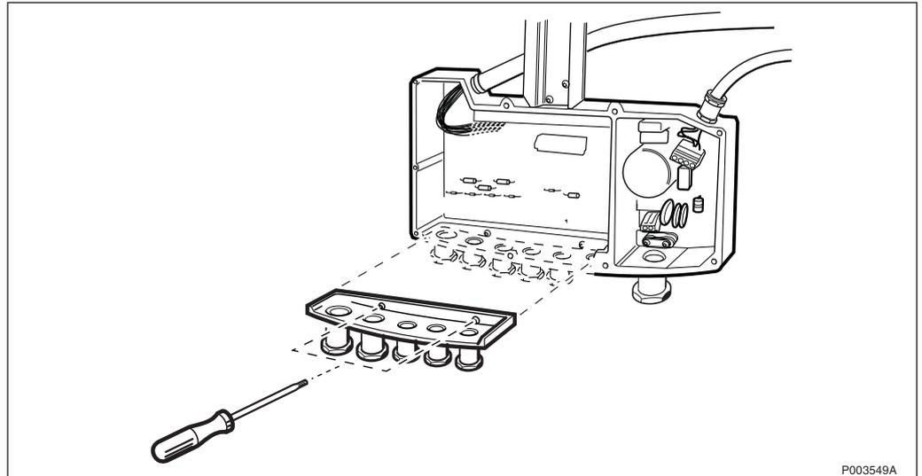
Figure 267 Loosening the gland plate
