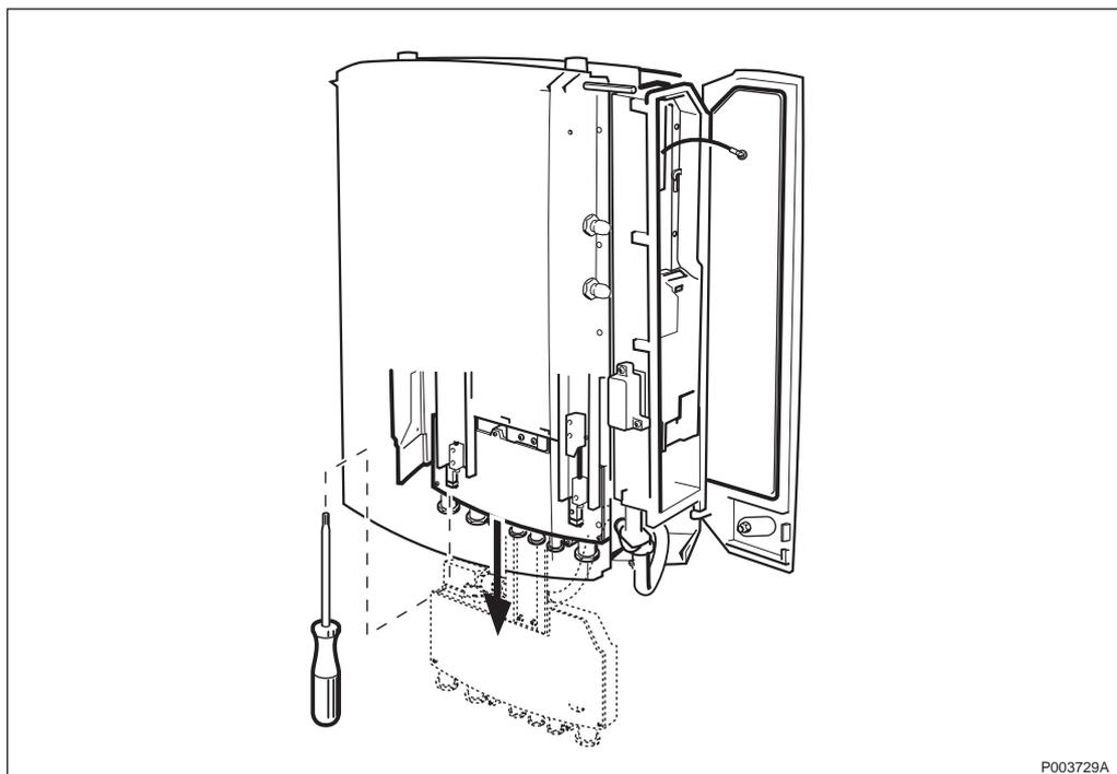
Figure 448 Loosening the interface box
