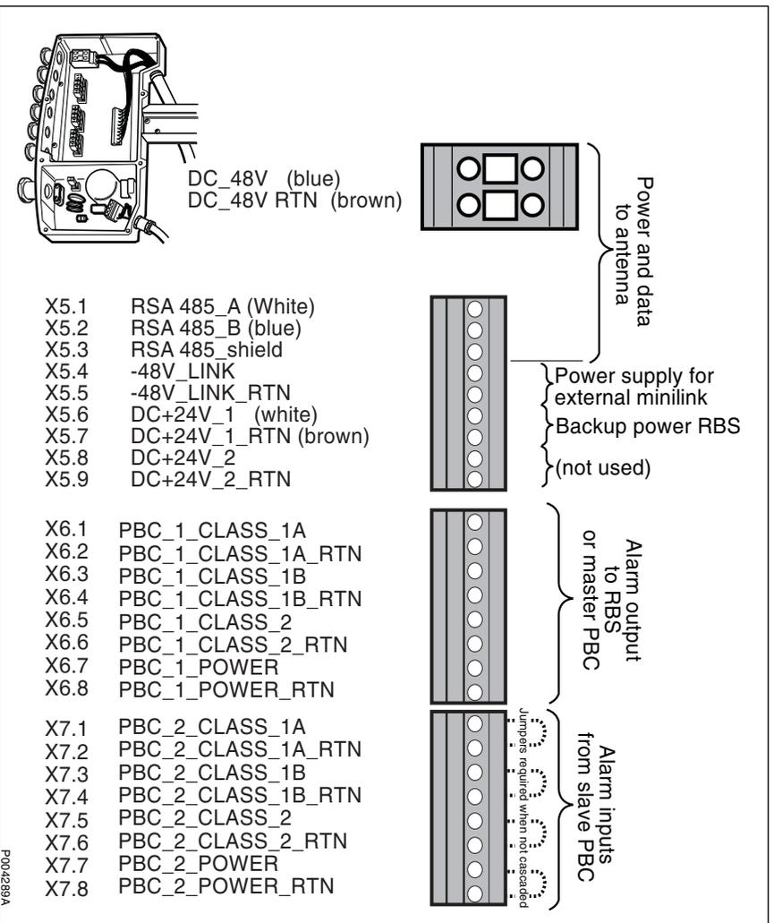
Figure 401 Cable connections for PBC
