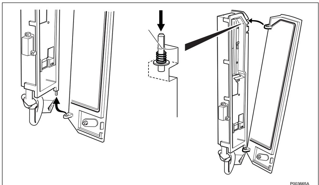
Figure 171 Mounting the installation box door
