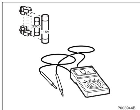
Switch off the Mains switch and the AC switch on the PBC. Measure the resistance of the fuses with a multimeter to verify that they are undamaged. (The resistance should be  $0 \Omega$ ). Then turn the power back on.
