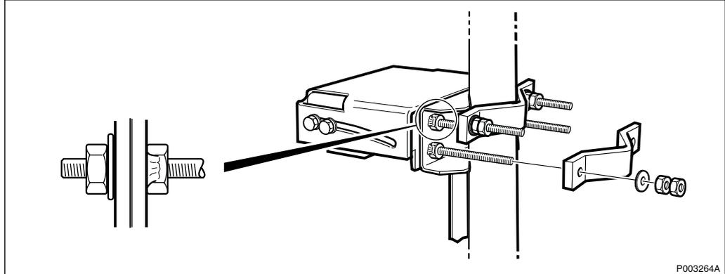
Figure 86 Fastening the mounting fixture using the clamps
