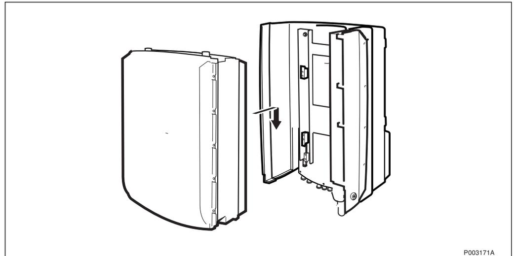
*Figure 132 Mounting the cabinet*
