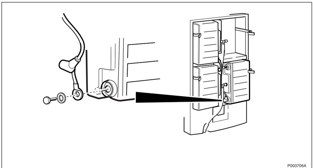
Figure 496 Disconnecting the minus-pole (-) of battery 3
