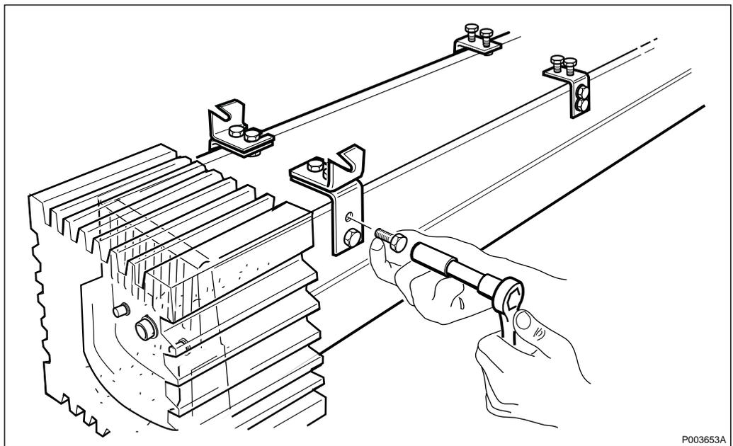
Figure 527 Mounting supports
