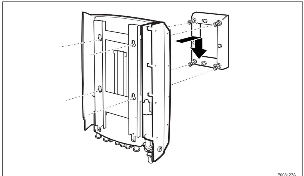
Figure 169 Mounting the mounting base on the mounting plate
