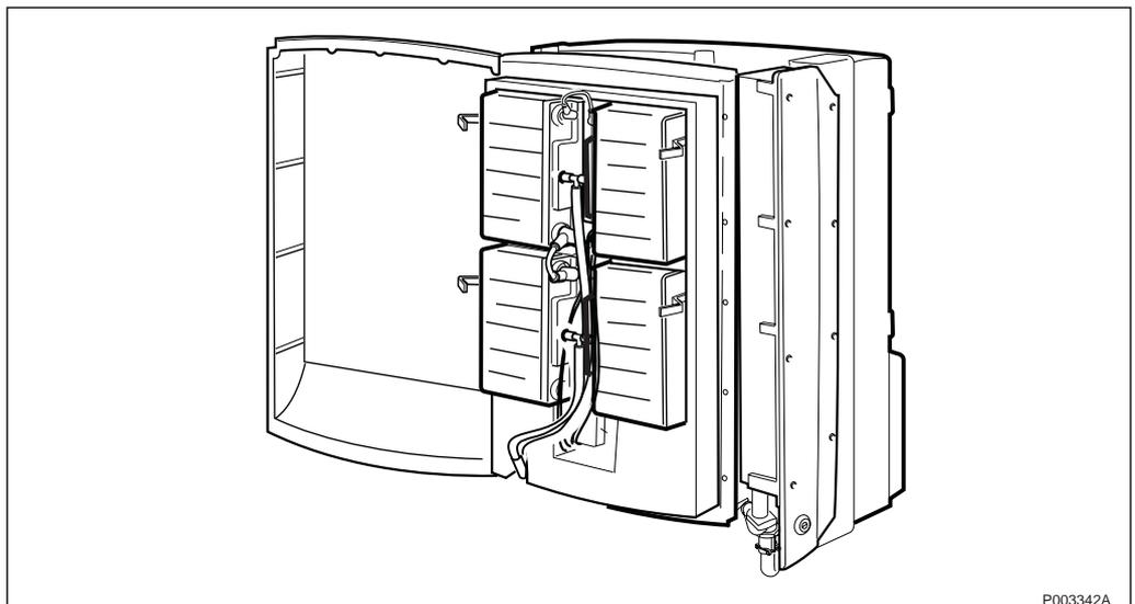
Figure 150 Power and Battery Cabinet
