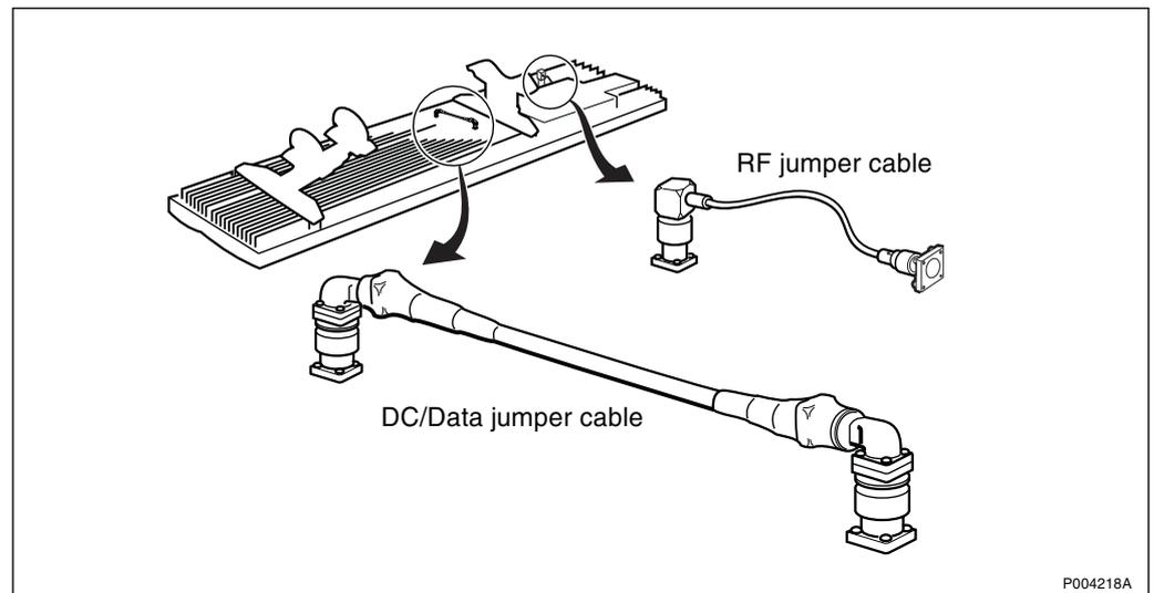
Figure 104 Connecting the DC/Data jumper cable and RF jumper cable to the antenna
