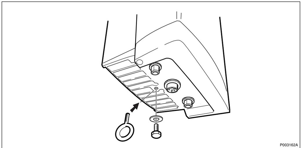
Figure 83 Preparing the lower end of the antenna for lift, by replacing the earthing screw with an eyebolt
