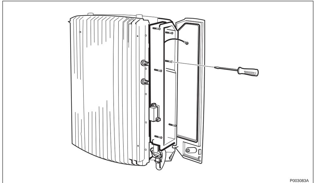
*Figure 210 Fastening the installation box*
