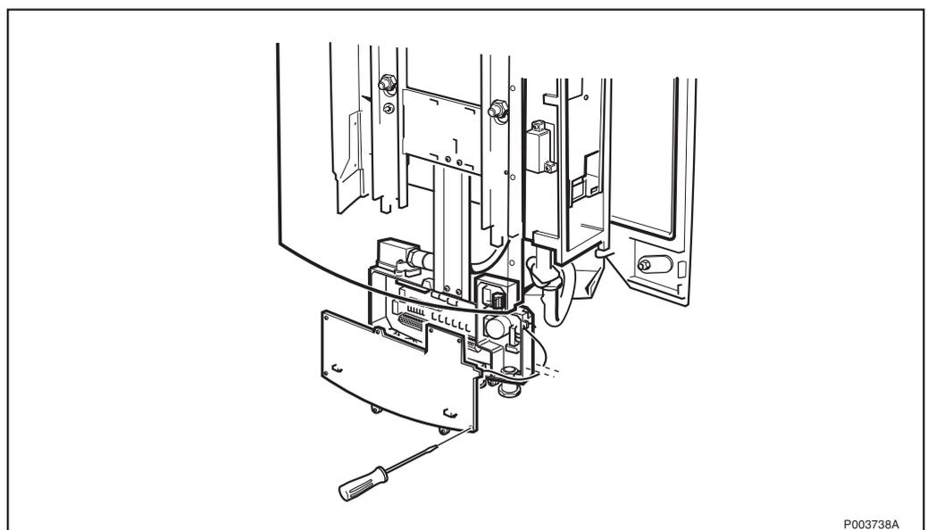
Figure 282 Loosen the interface box lid
