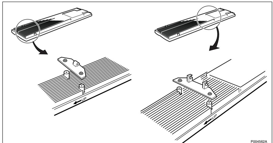
Figure 535 Remounting the brackets on the new antenna
