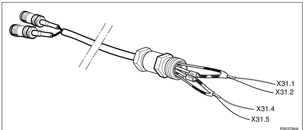
Figure 294 75 Ω PCM cable
