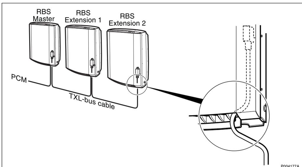
Figure 315 TXL-bus connection for 6 TRX configuration
