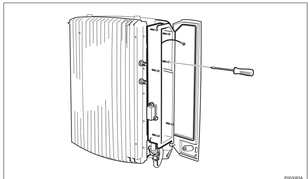
*Figure 428 Loosening the installation box*
