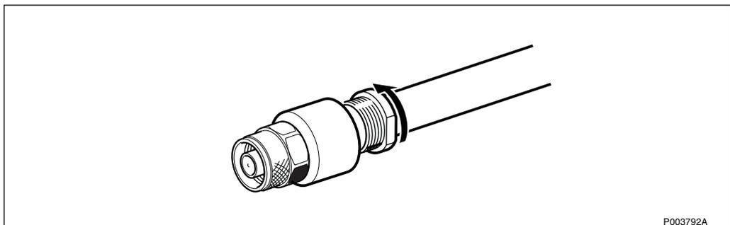
Figure 249 Mounting the front connector body
