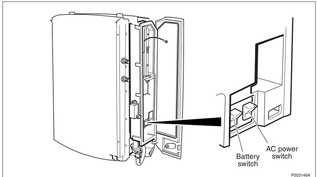
Figure 183 AC power and battery switches
