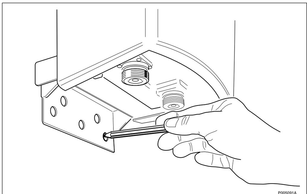
Figure 71 Using the lower wall bracket as a template
