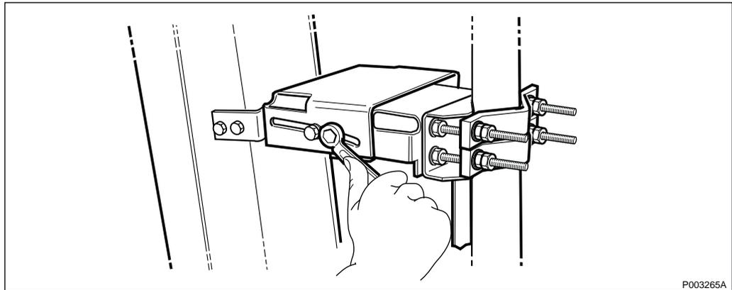
Figure 89 Adjusting the tilt angle
