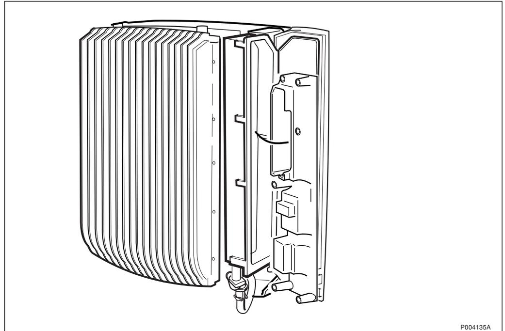
Figure 503 Removing the protective cover
