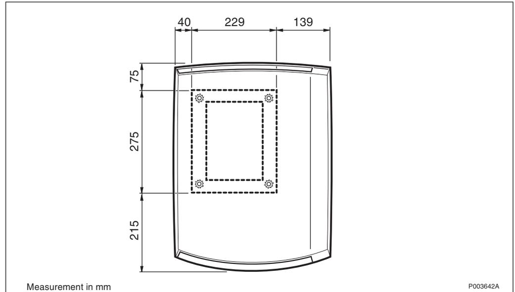
Figure 557 Mounting plate and equipment contour
