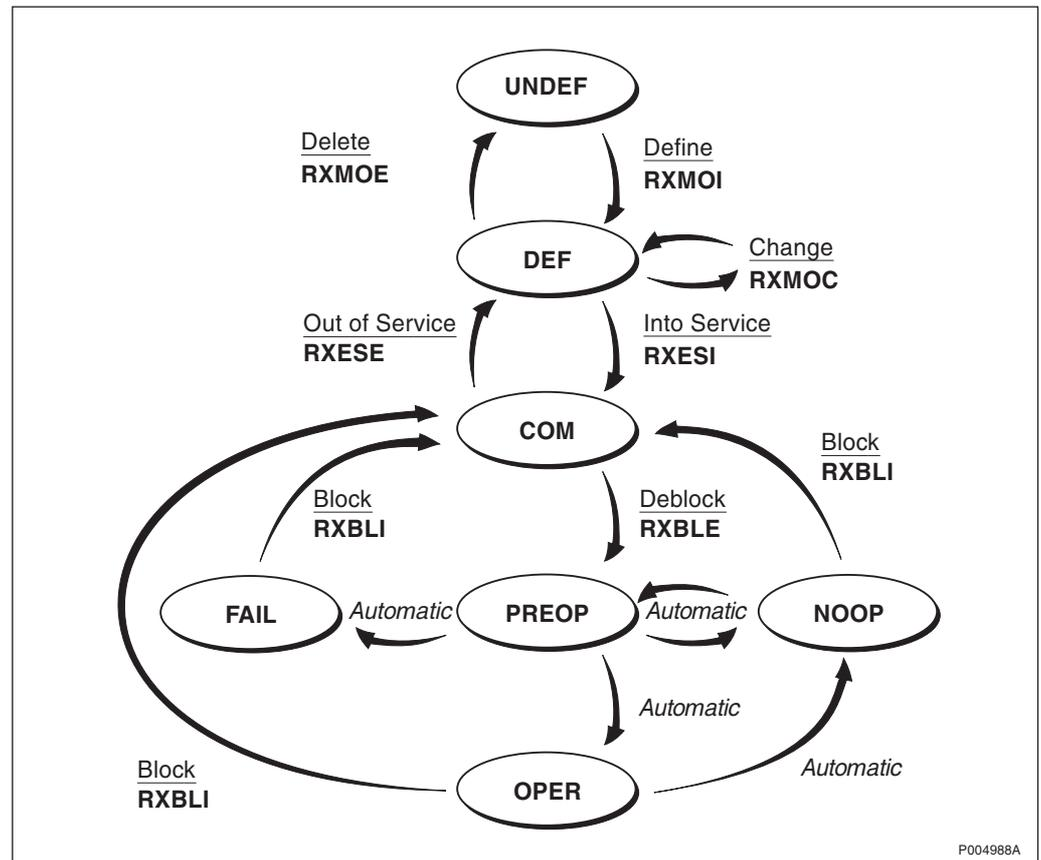
Figure 378 Description of the relation between the different managed object states
