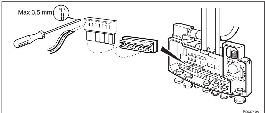
Figure 284 Loosening the termination block
