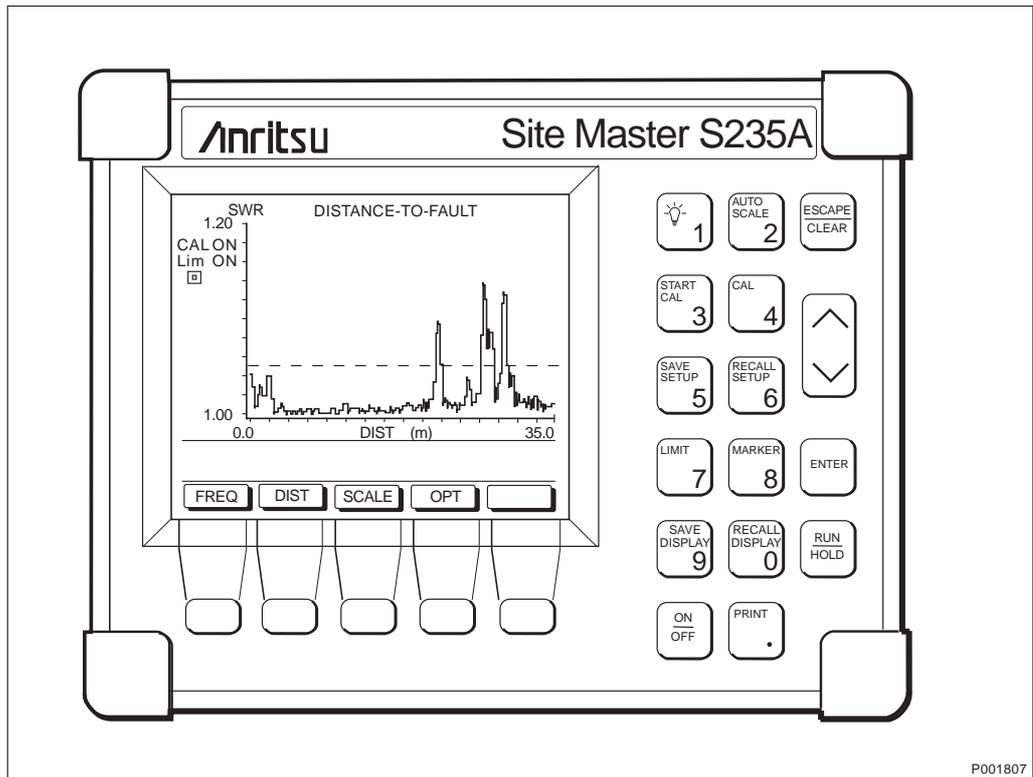
Figure 334 Example showing a bad adapter at the antenna
