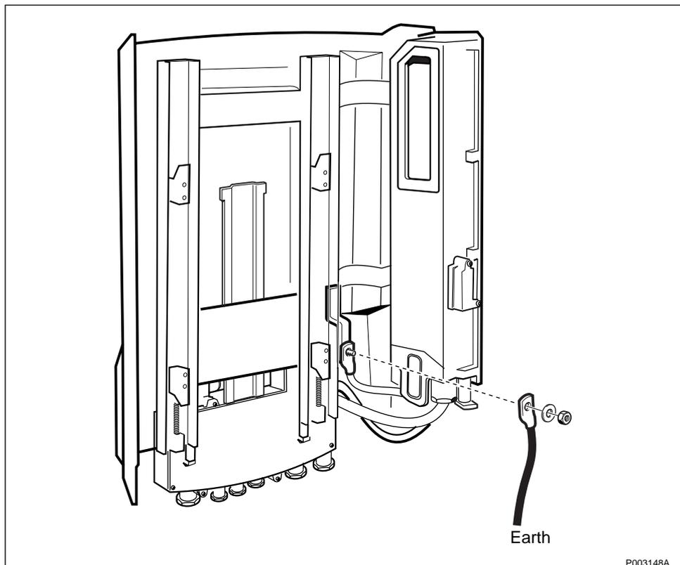
Figure 457 Remove the Earth Cable
