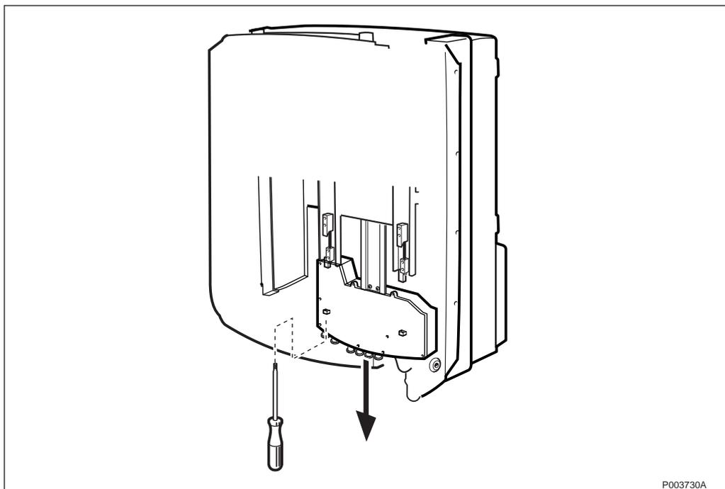
*Figure 510 Loosening the interface box*
