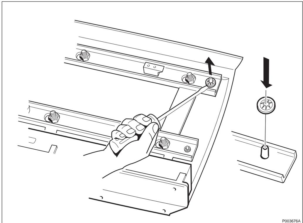
Figure 468 Removing locking washers
