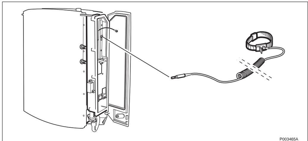
Figure 435 Connecting the ESD wrist strap
