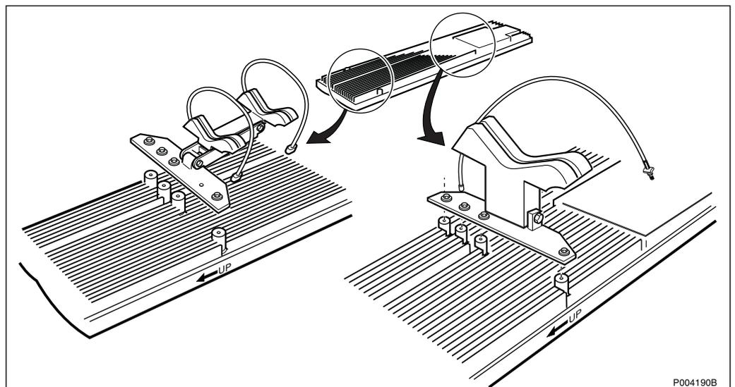
Figure 584 AAU mounting fixture
