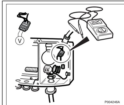
Measure that 115/230 V is present at the upper AC plinth on the AC board to verify that the AC board is not faulty.
