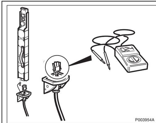
Examine the PSA cable by measuring that 24 V is present on the incoming connector to the PSA. If there is, replace the PSA. If not, replace the cable.
