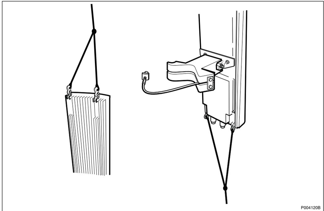
Figure 105 Upper lifting shackles and lower control shackles, antenna 500 W EIRP
