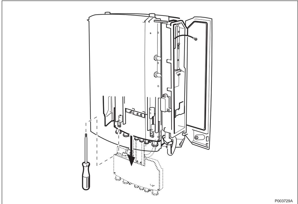
Figure 452 Loosening the interface box
