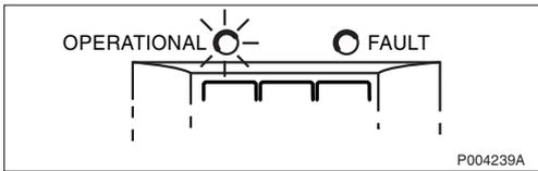
If the green LED "Operational" is lit but not the red LED "Fault" this means that the Power and Battery Cabinet and the AAU are operational and that no affecting alarms are active.
