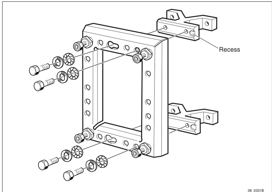
Figure 166 Fastening the clamps and mounting the washers
