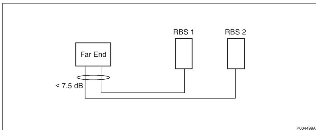
Figure 348 Line Build Out
