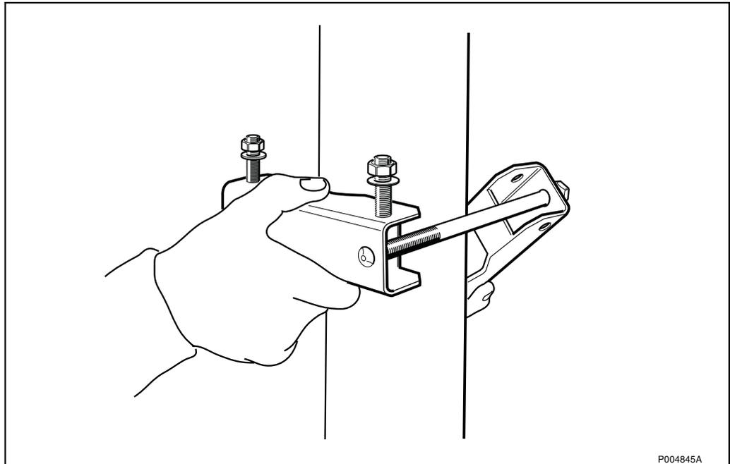
Figure 59 Placing the upper mounting fixture on the pole
