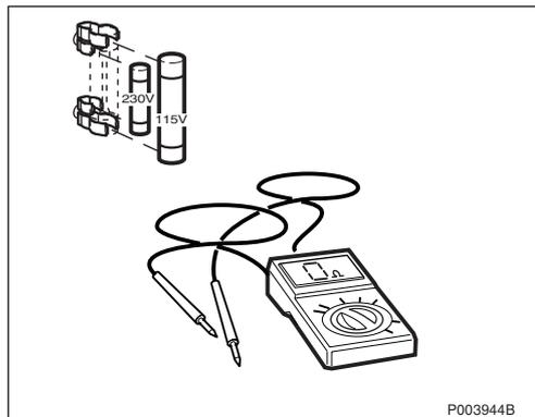
2/ The fuses are damaged and the batteries have been discharged. Turn off the Mains switch and the AC switch on the battery cabinet. Measure the resistance of the fuses with a multimeter to verify that they are undamaged (The resistance should be 0  $\Omega$ ).
