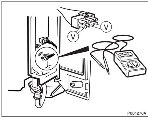
Measure that 155/230 V is present at the connector of the internal AC cable attached to the battery cabinet to verify that the internal AC cable is not faulty. If voltage is present, replace the battery cabinet.
