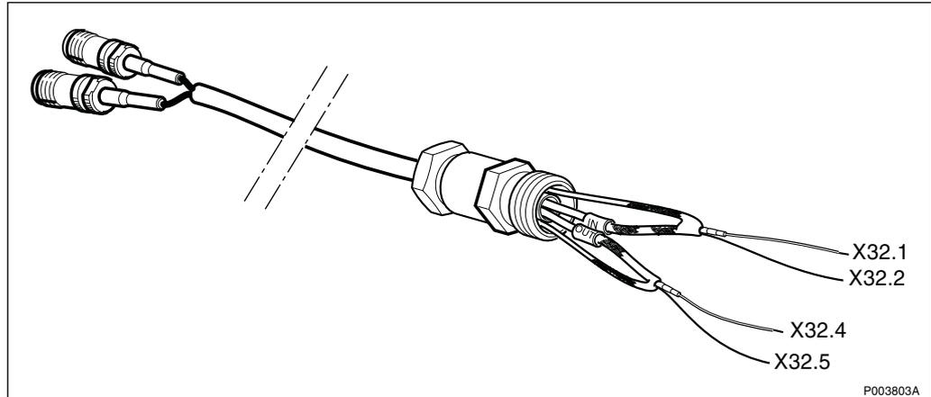
Figure 297 75 Ω PCM cable
