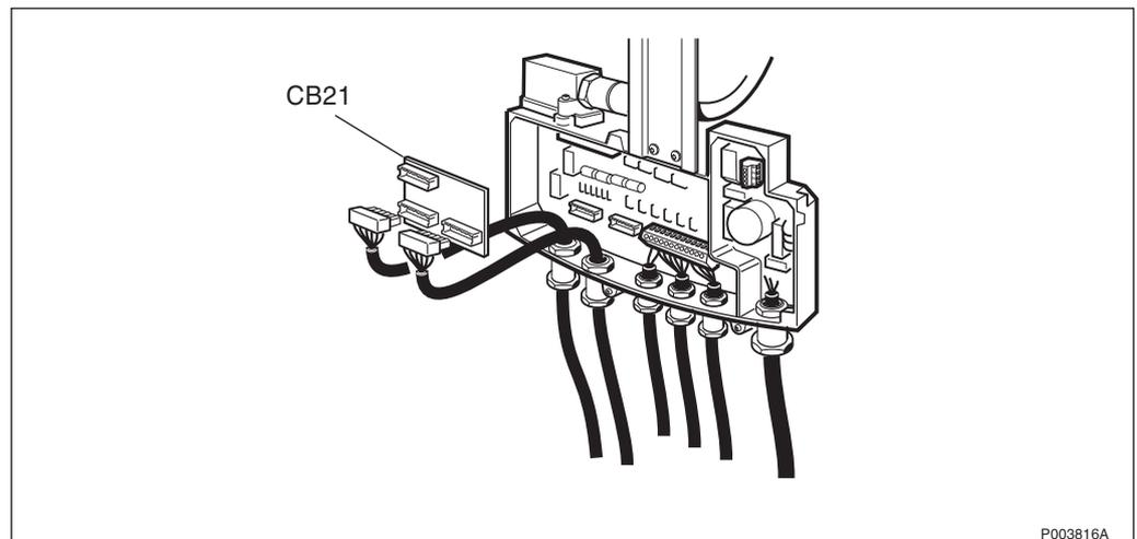
Figure 454 Mounting the CB21 connection board
