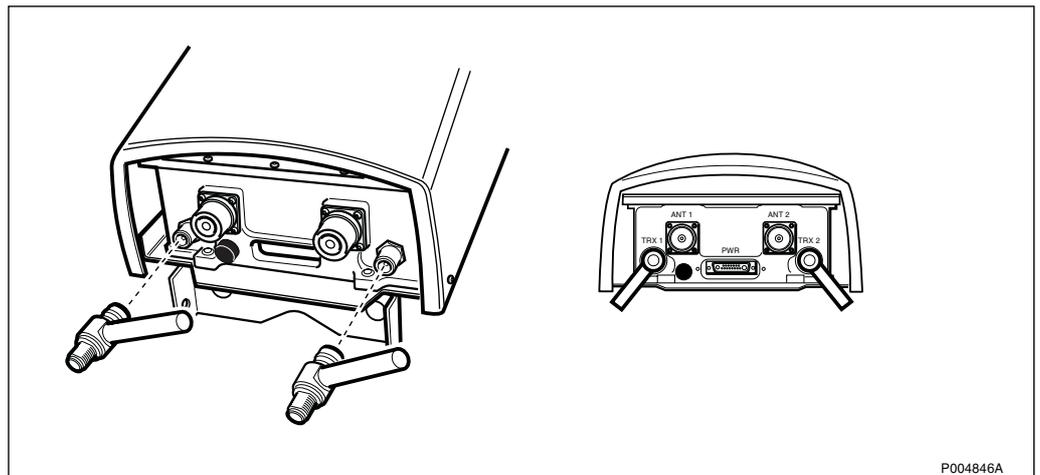
Figure 77 Connecting the RF lightning protectors
