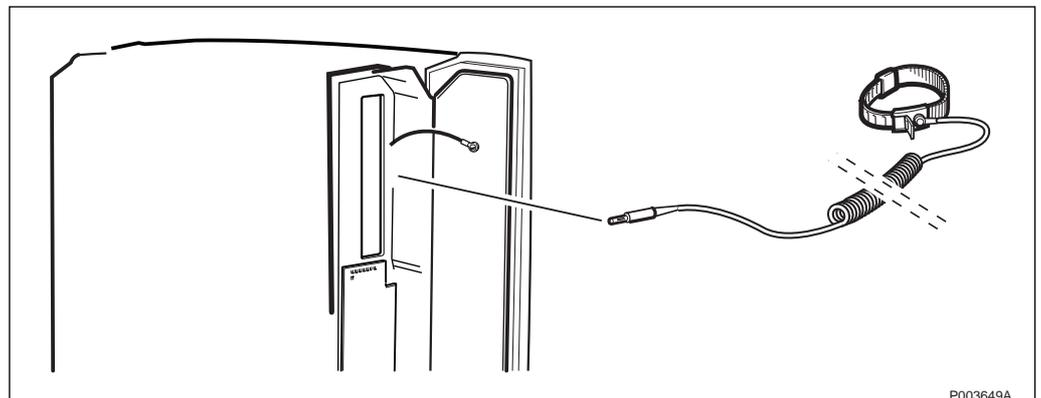
Figure 512 Connecting the ESD wrist strap
