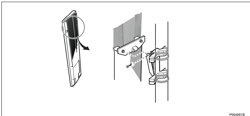
Figure 533 Unscrewing the screw on the upper mount
