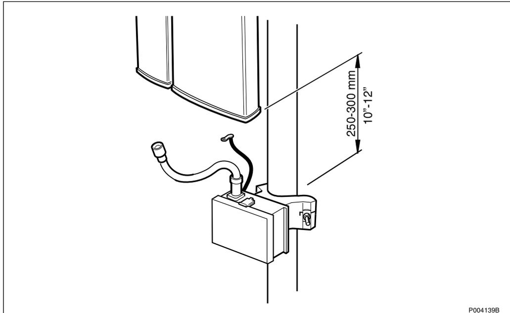
Figure 586 Lightning protection for 1250 W EIRP GSM 1900 antenna
