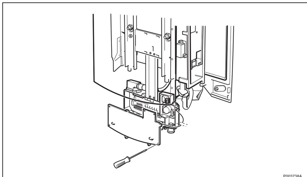
Figure 443 Loosening the interface box cover
