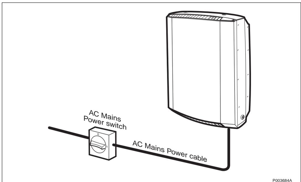
Figure 397 AC mains power switch turned on
