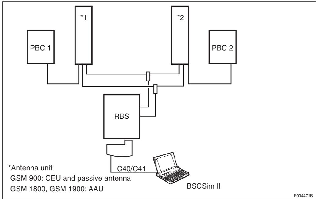
Figure 364 Test setup: 2 TRX Highway configuration
