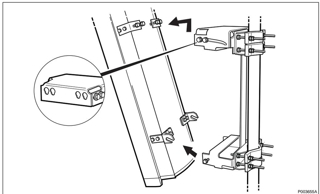
Figure 525 Unhooking the antenna
