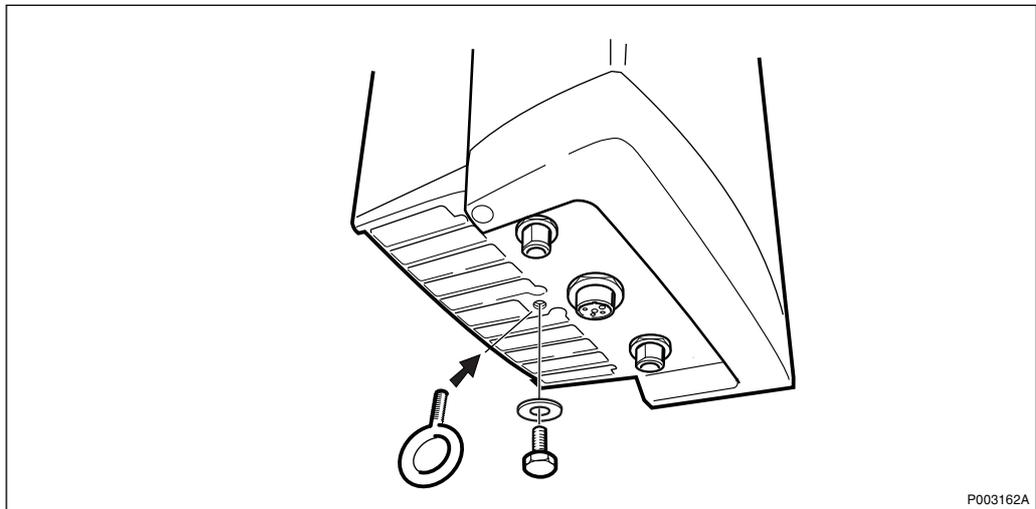
Figure 523 Replacing the earth screw with an eyebolt
