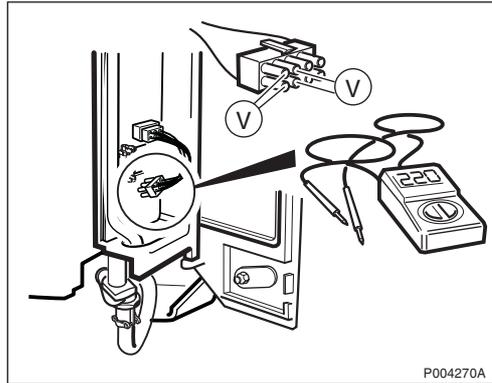
1/ The battery cabinet has no power and the batteries have been discharged. Check if 115/ 230 V is present to the battery cabinet by measuring on the internal AC cable.
