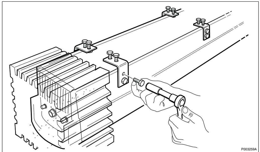
Figure 81 Attaching the angle supports to the antenna
