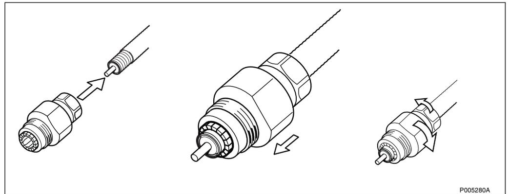
Figure 255 Mounting the cable entry
