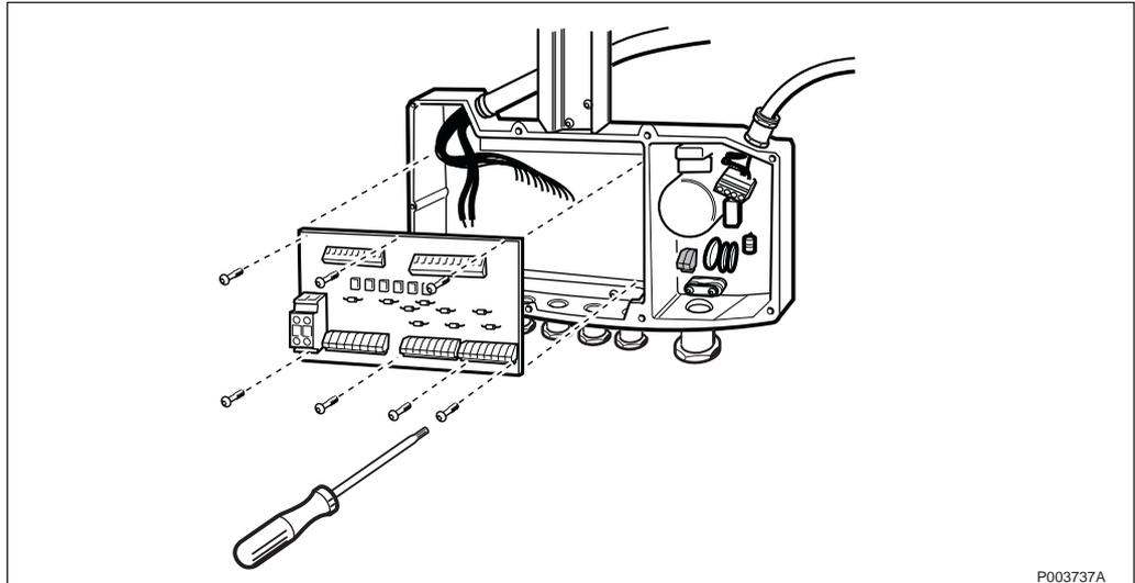
Figure 513 Removing the DC Surge board
