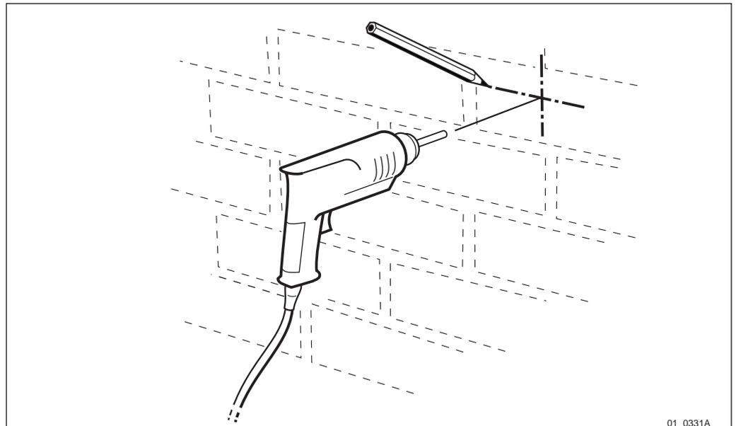
Figure 117 Marking the position of the mounting plate and drilling the hole
