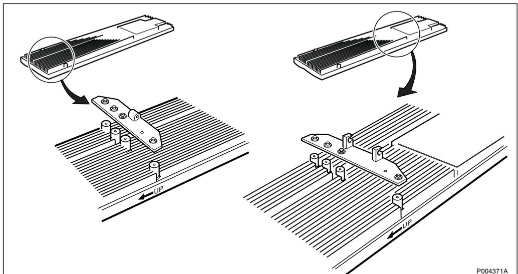
Figure 543 Remounting the brackets on the new antenna
