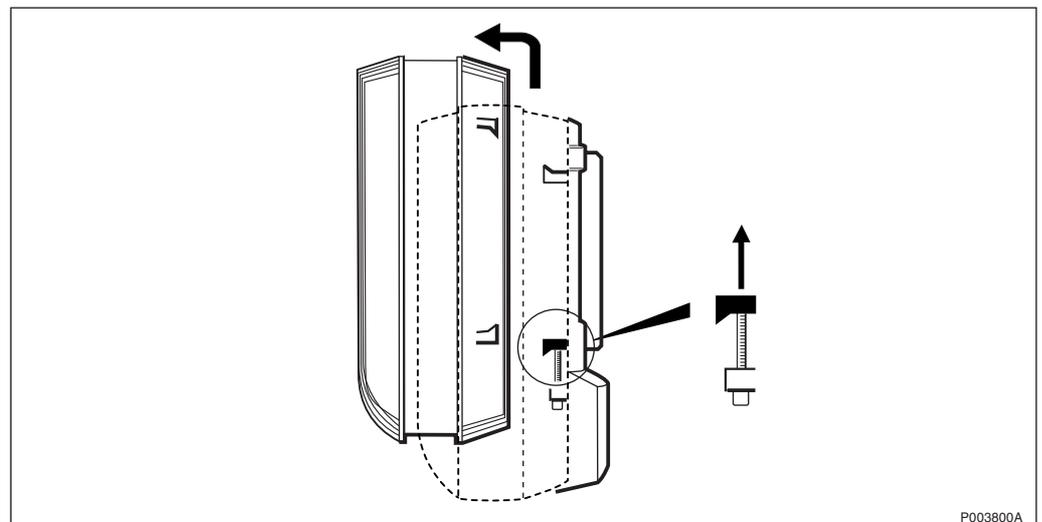
Figure 502 Unhooking the PBC
