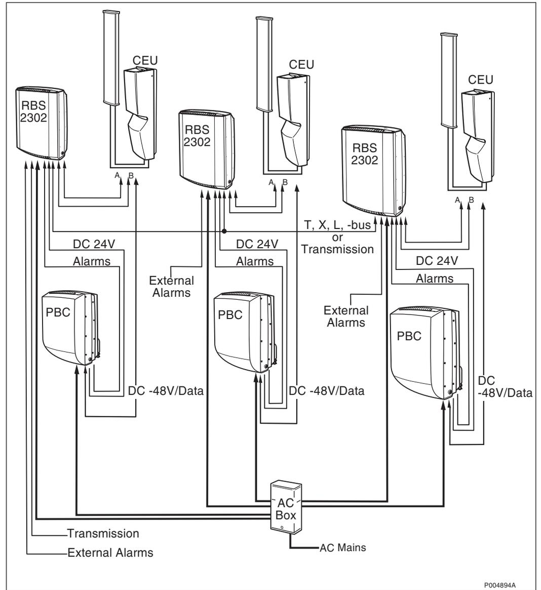
Figure 49 Configuration with 6 TRX
