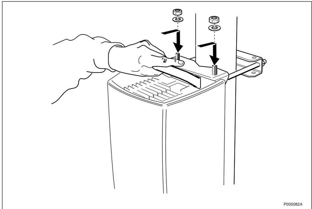
Figure 63 The CEU hooked on to the stud bolts on the upper mounting fixture
