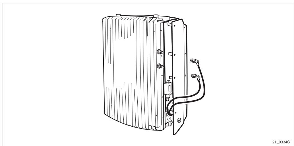
Figure 426 Disconnecting the Antenna cables
