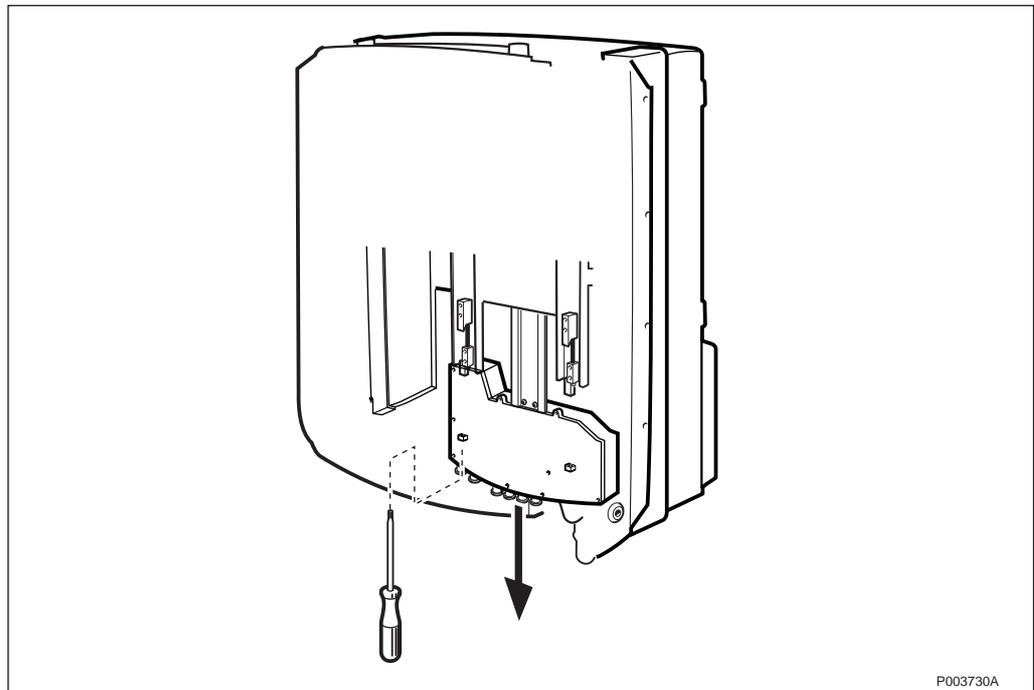
Figure 265 Pulling down the interface box
