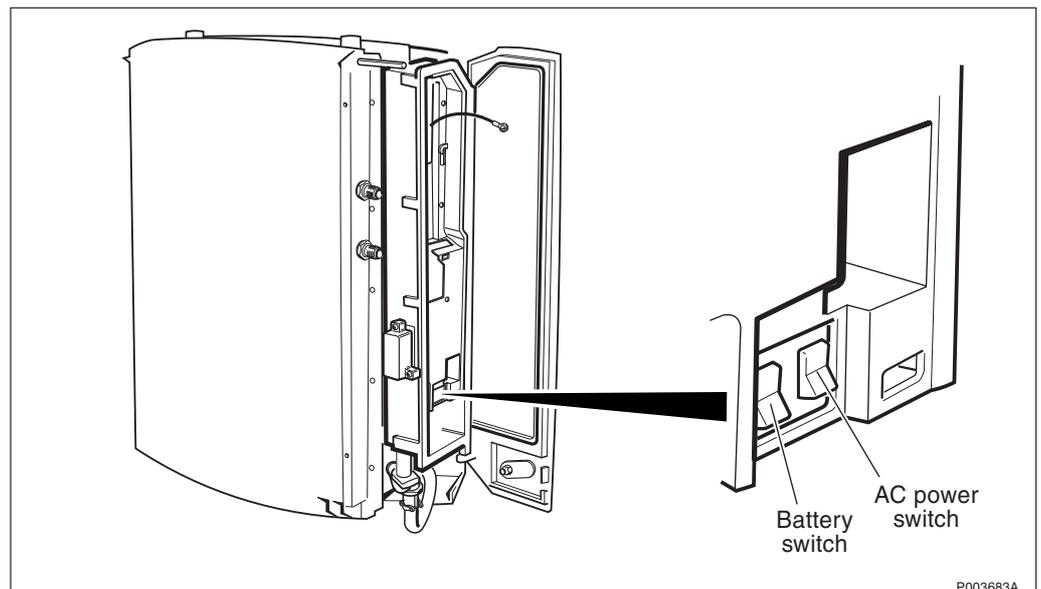
Figure 399 Battery and AC power switch
