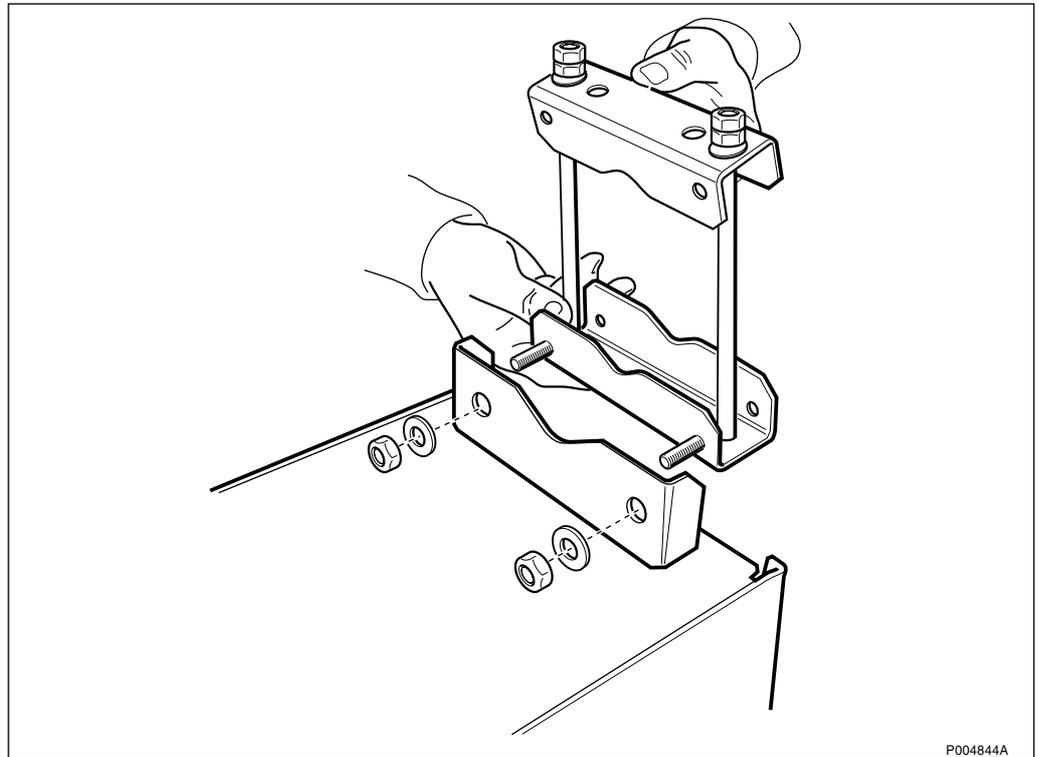
Figure 570 CEU mounting fixtures for poles
