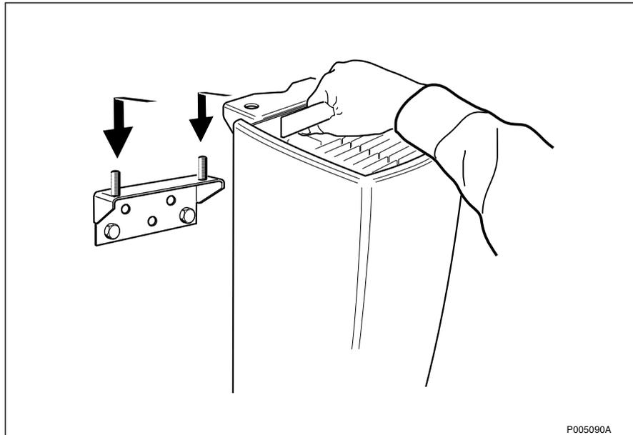
Figure 70 Placing the CEU on the wall bracket
