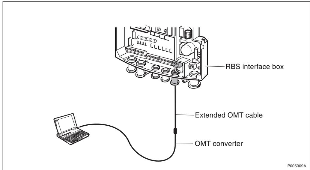
Figure 339 Test setup with extended OMT cable
