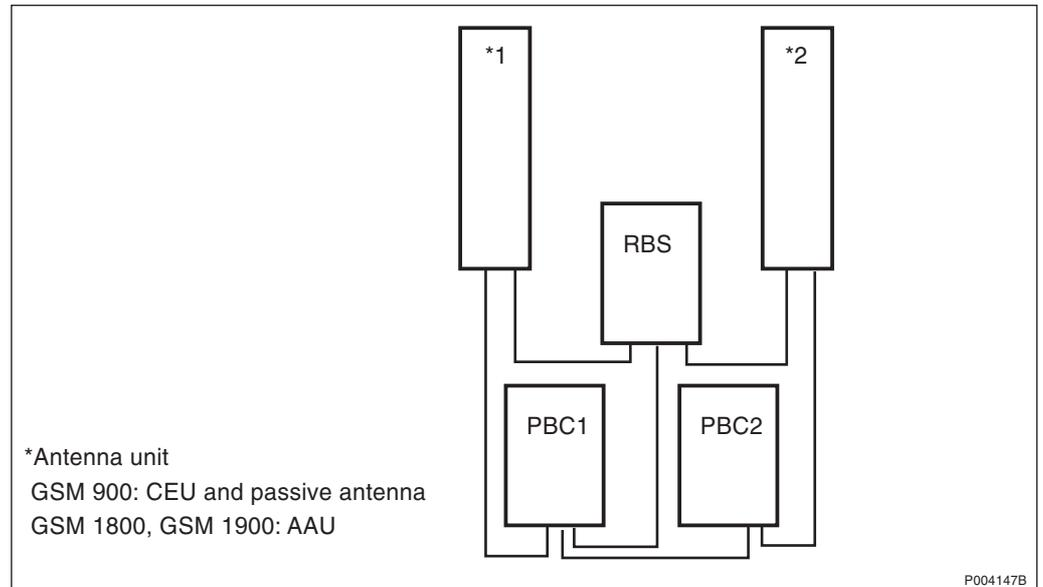
Figure 337 2 TRX Highway configuration
