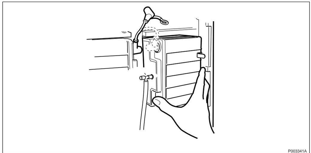
Figure 486 Connecting battery 2 and 4
