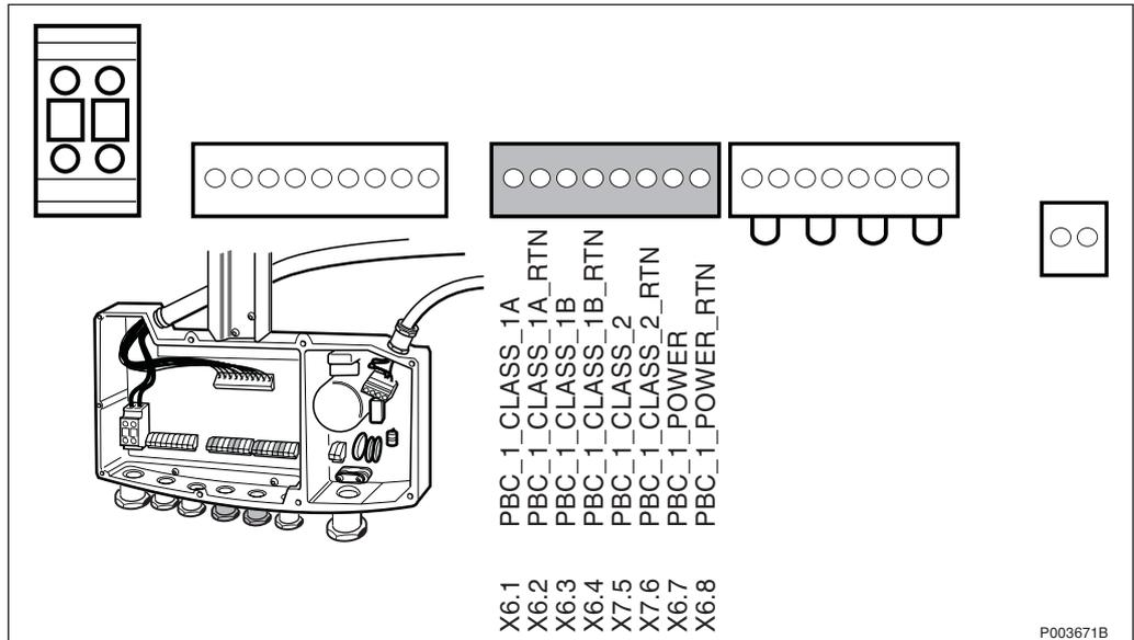
Figure 277 Alarm termination block
