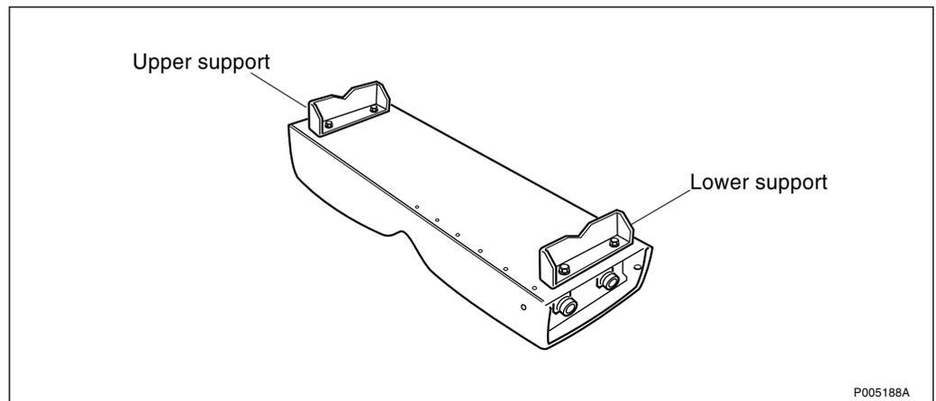
Figure 57 Definition of upper and lower angle support
