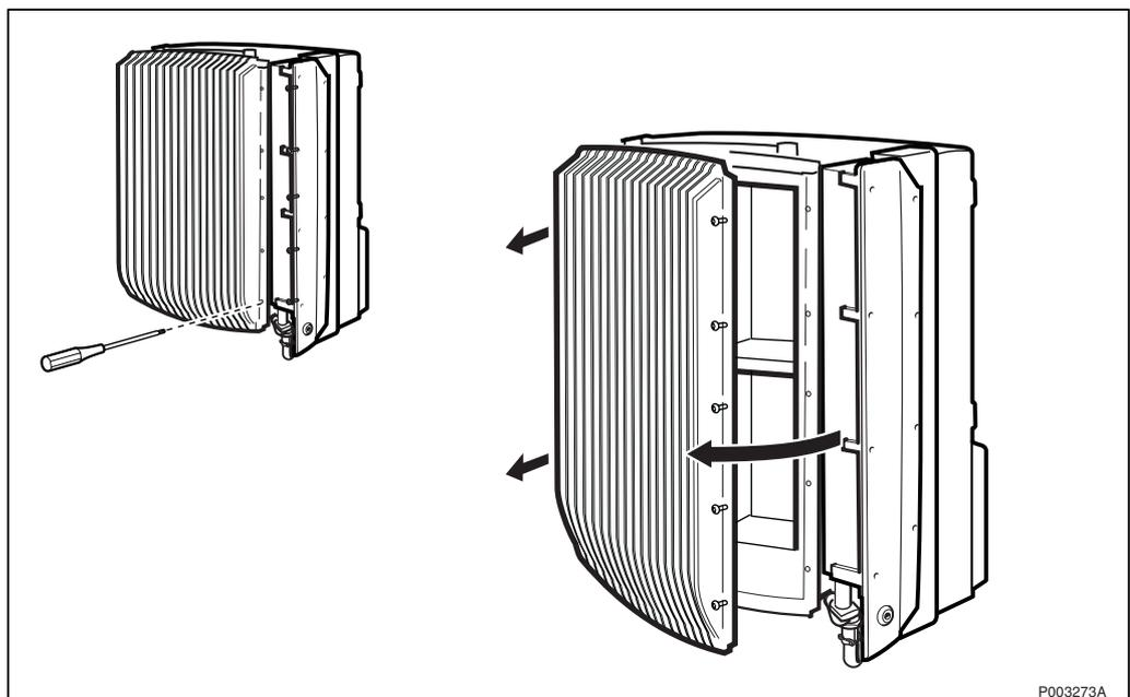
Figure 471 Opening the Battery cabinet door
