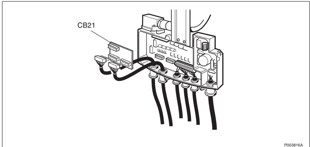
Figure 414 Mounting the CB21 connection board
