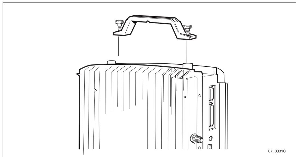
Figure 179 Mounting the lifting handle
