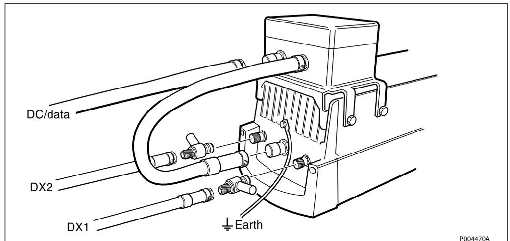
Figure 237 Connecting Lightning Protection for the GSM 1800 system
