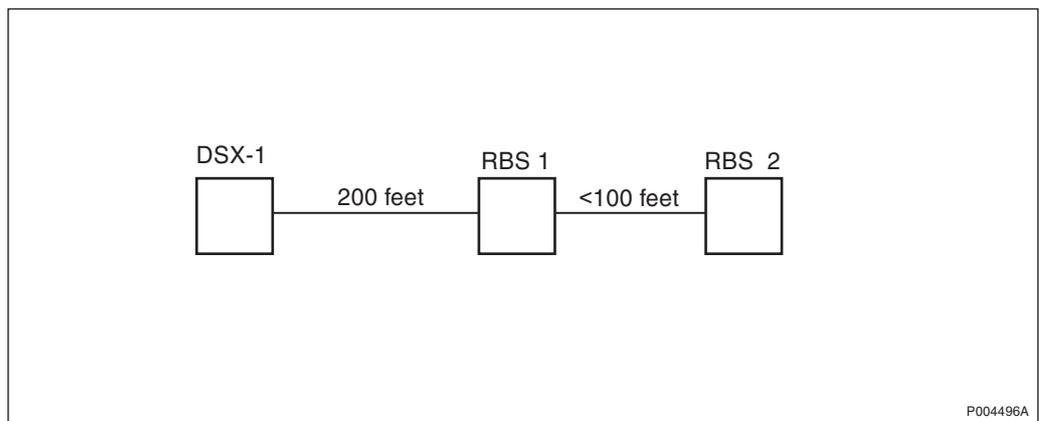
Figure 345 The Short Haul Multidrop principle
