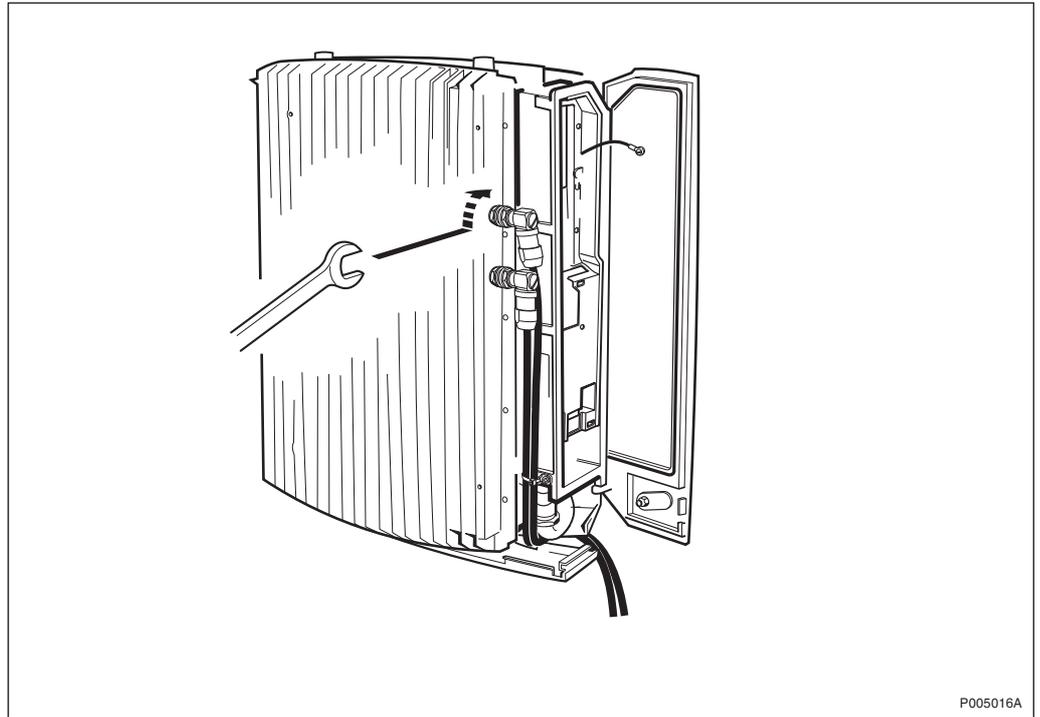
*Figure 313 Tightening of the nuts for the connectors*
