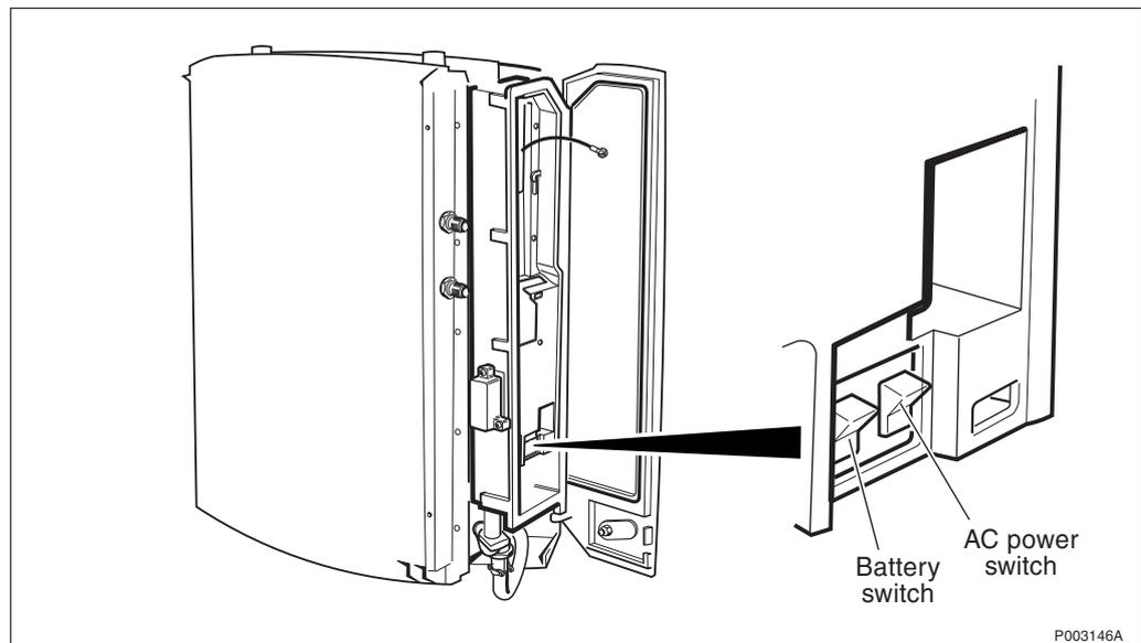
Figure 394 Battery and AC power switch in the RBS
