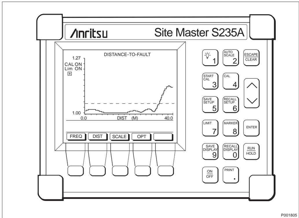
Figure 333 Measurement of an approved cable
