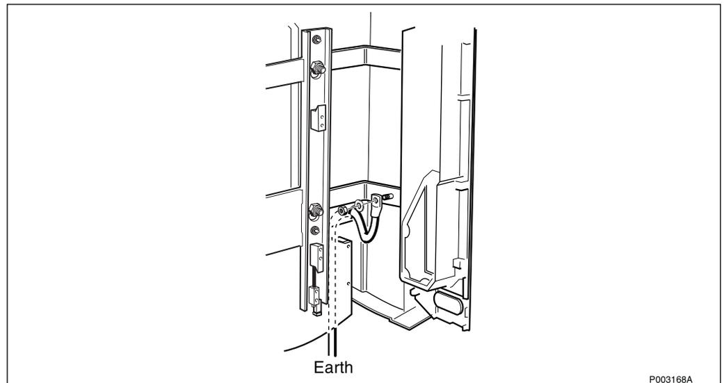
Figure 467 Removing the earth cable
