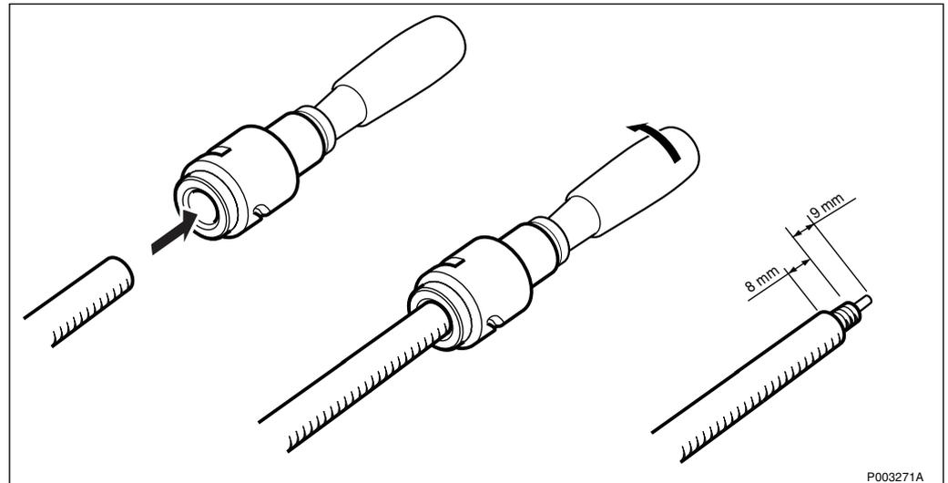
Figure 242 Dismantling the antenna feeder
