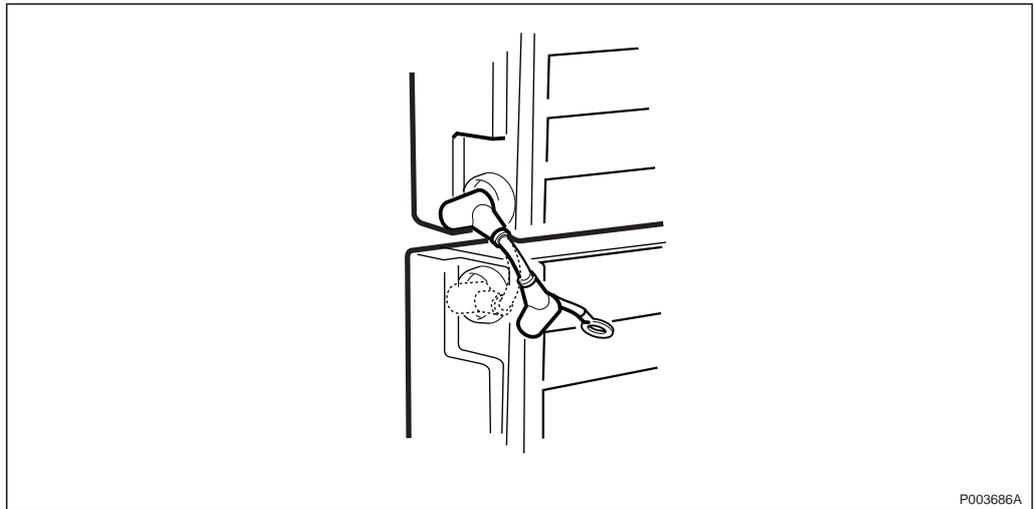
Figure 495 Disconnecting the plus-pole (+) of battery 3
