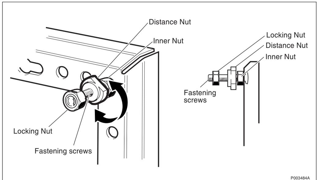
Figure 126 Adjusting the distance nuts
