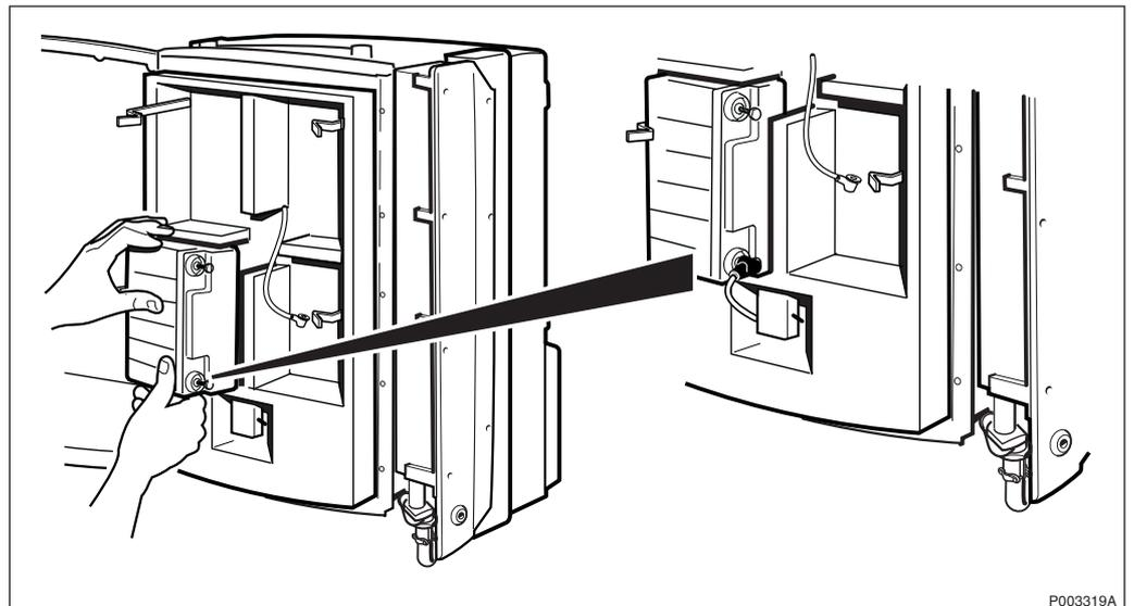
Figure 143 Inserting the battery 1
