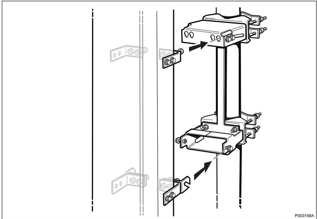
Figure 574 AAU mounting fixture
