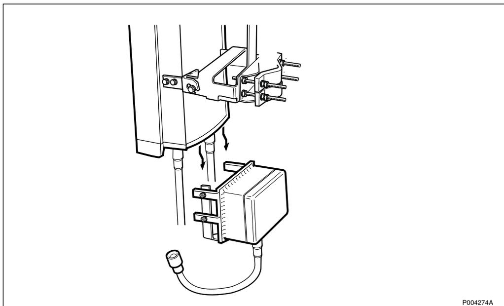
Figure 529 *Loosening the ALPU from the mounting fixture*
