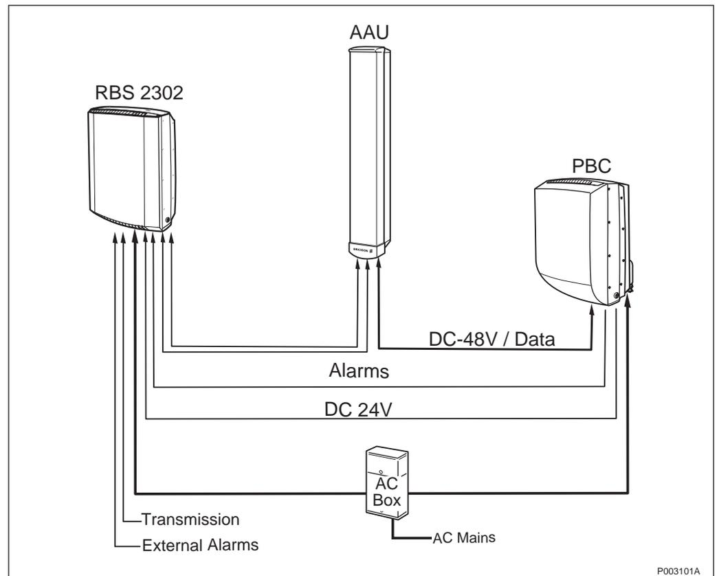
Figure 51 Configuration with 2 TRX
