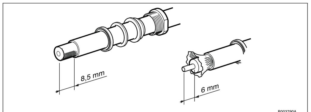
Figure 247 Dismantling the antenna cable
