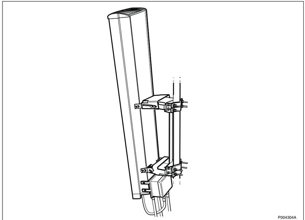
Figure 90 The DC/Data Lightning Protector mounted on the antenna
