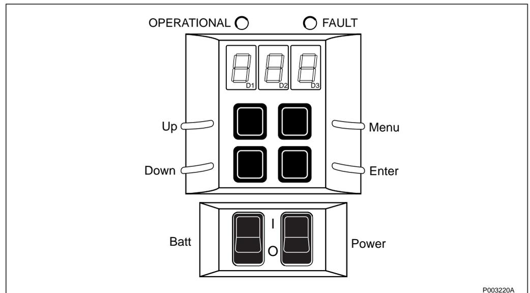
Figure 390 PBC control panel
