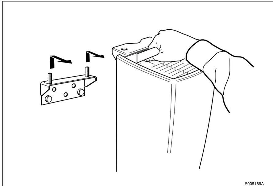
Figure 72 Removing the CEU from the wall bracket
