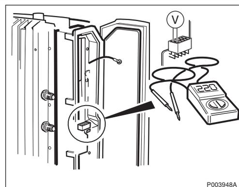
Measure that 115/230 V is present at the connector to the internal AC cable, to verify that the connection board is not defective.
