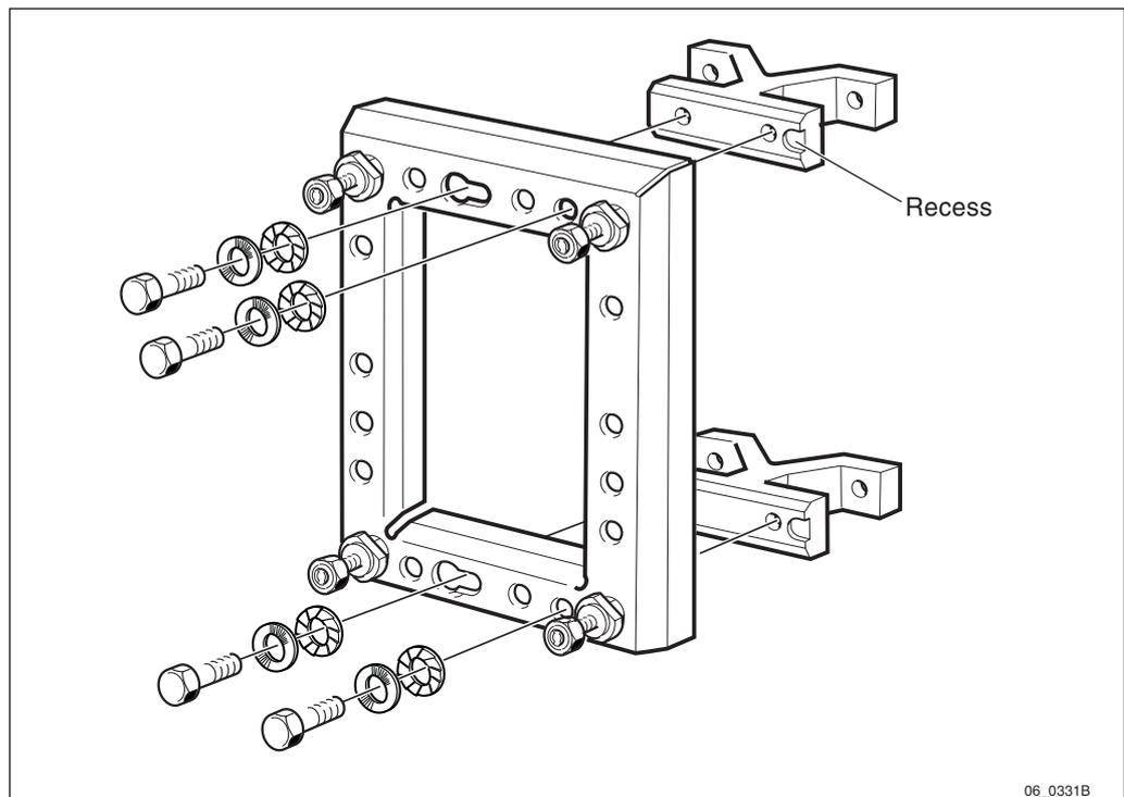
Figure 122 Fastening the clamps and mounting the washers
