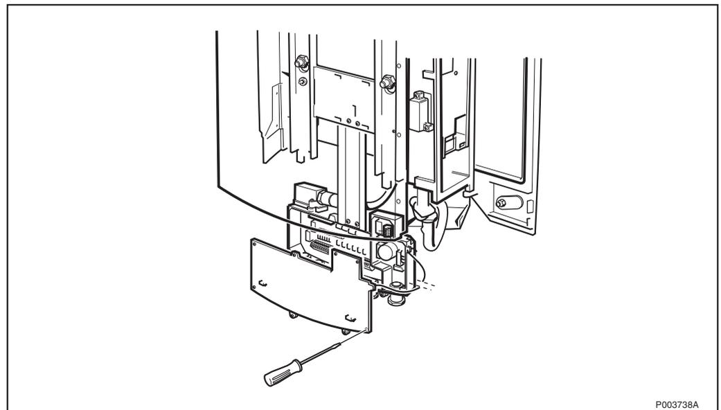
Figure 412 Loosening the interface box cover
