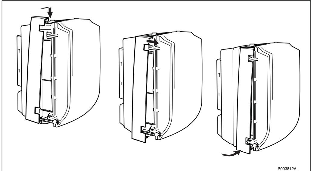
Figure 153 Mounting the left sunshield
