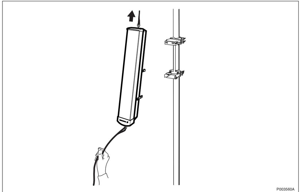
Figure 87 Using the control rope to guide the antenna when hoisted
