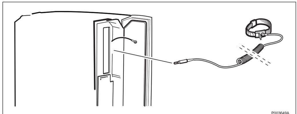
Figure 506 Connecting the ESD wrist strap
