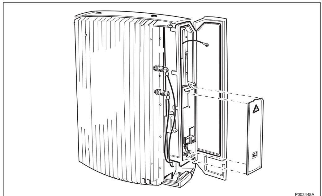
Figure 432 Removing the outer protective cover
