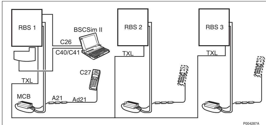
Figure 359 Test setup for 4 TRX and 6 TRX configurations
