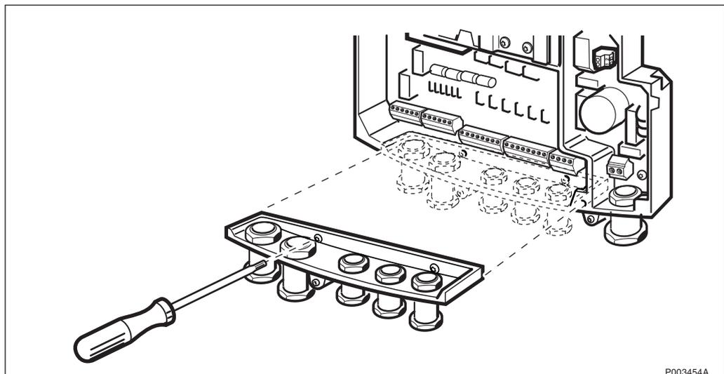
Figure 456 Loosening the gland plate
