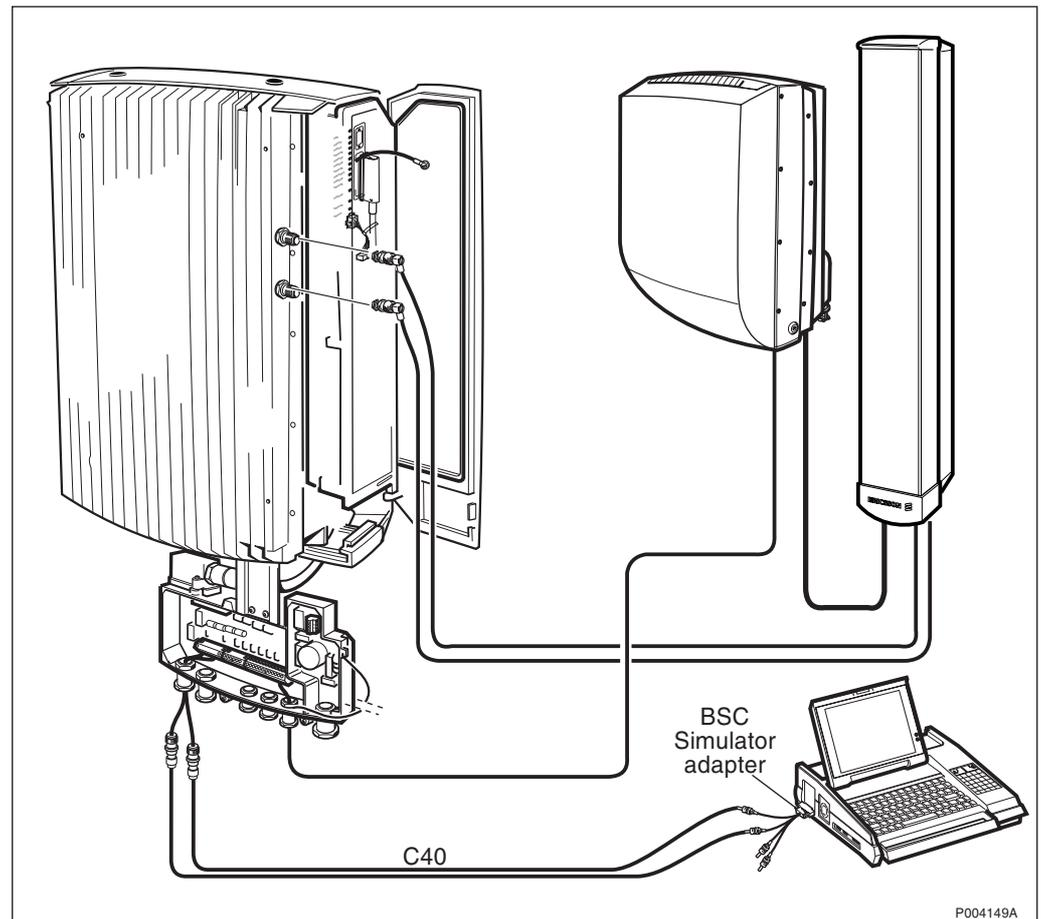
Figure 361 Test setup for GSM 1800 and GSM 1900: 2 TRX Sector Configuration for E1 75  $\Omega$  (2.0 Mbit/s)
