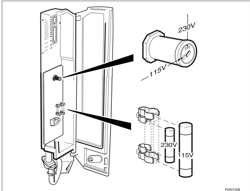
Figure 433 Replacing the fuses
