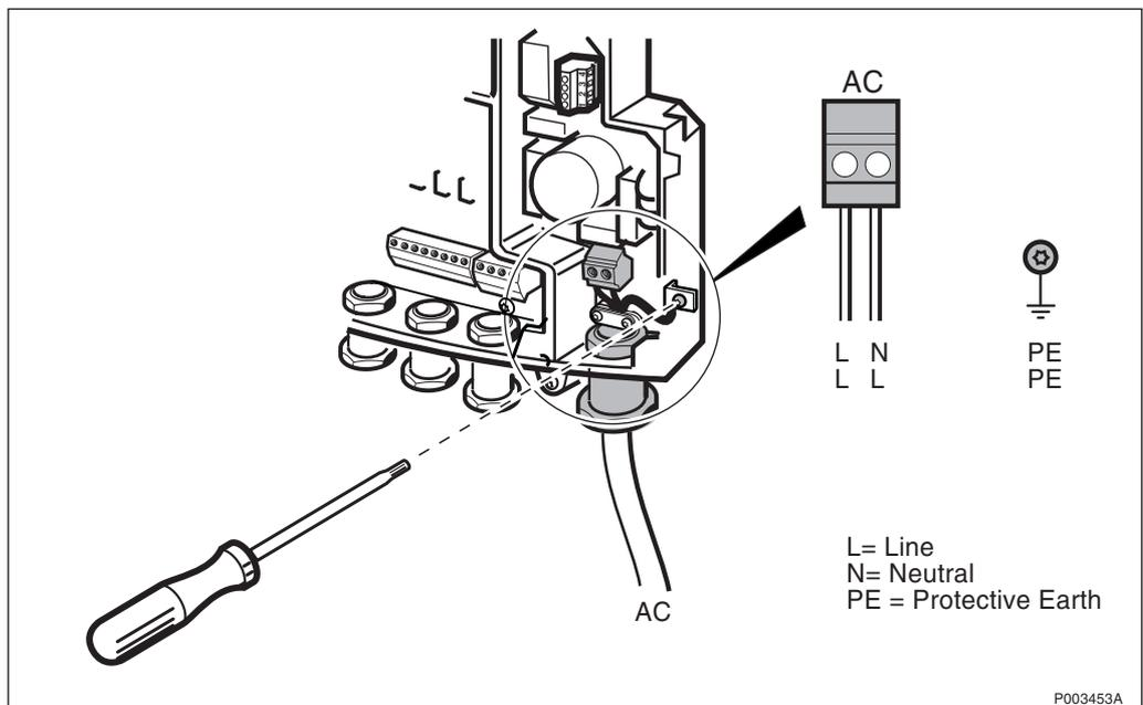
Figure 415 Loosening the Protective Earth in the AC section of the interface box
