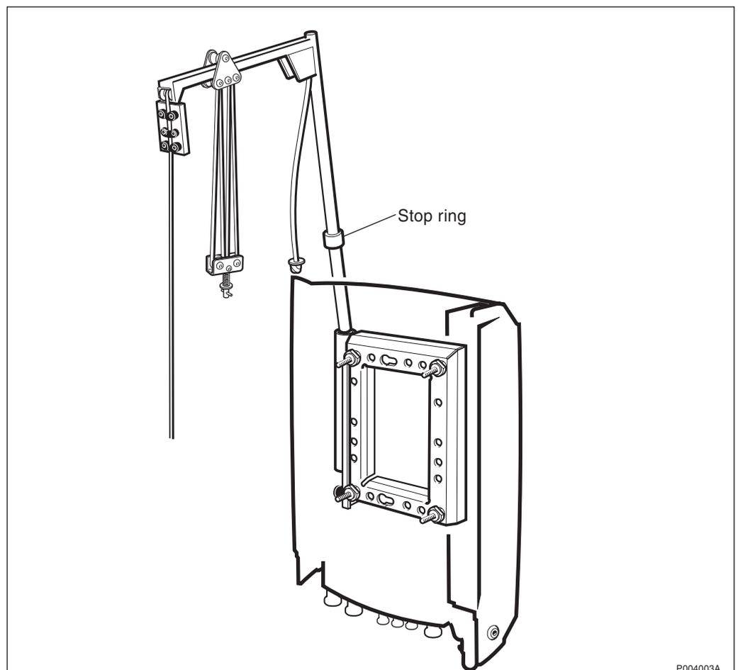
Figure 200 Inserting the lifting device in the tube-bracket
