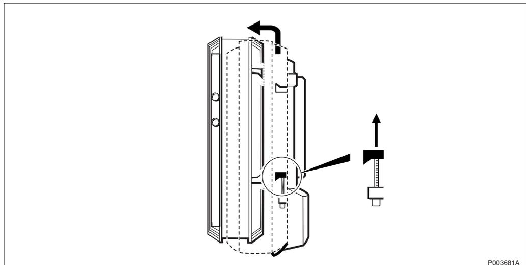
Figure 430 Unhooking the radio cabinet
