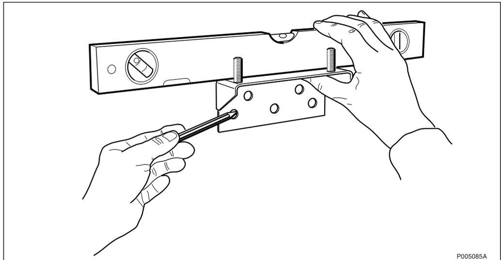
Figure 66 Positioning the upper wall bracket using a spirit level
