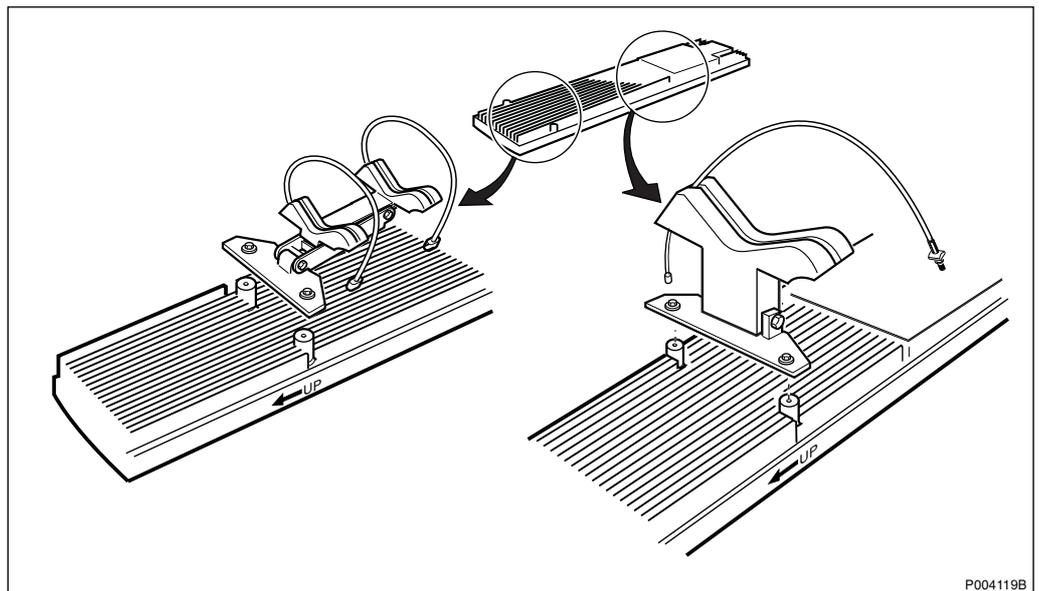
Figure 580 AAU mounting fixture
