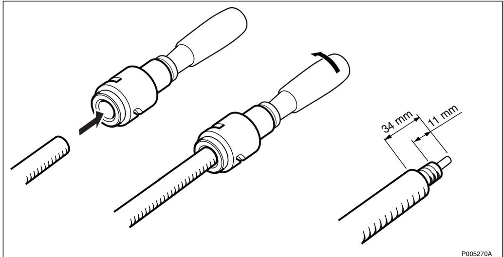
Figure 252 Dismantling the antenna feeder
