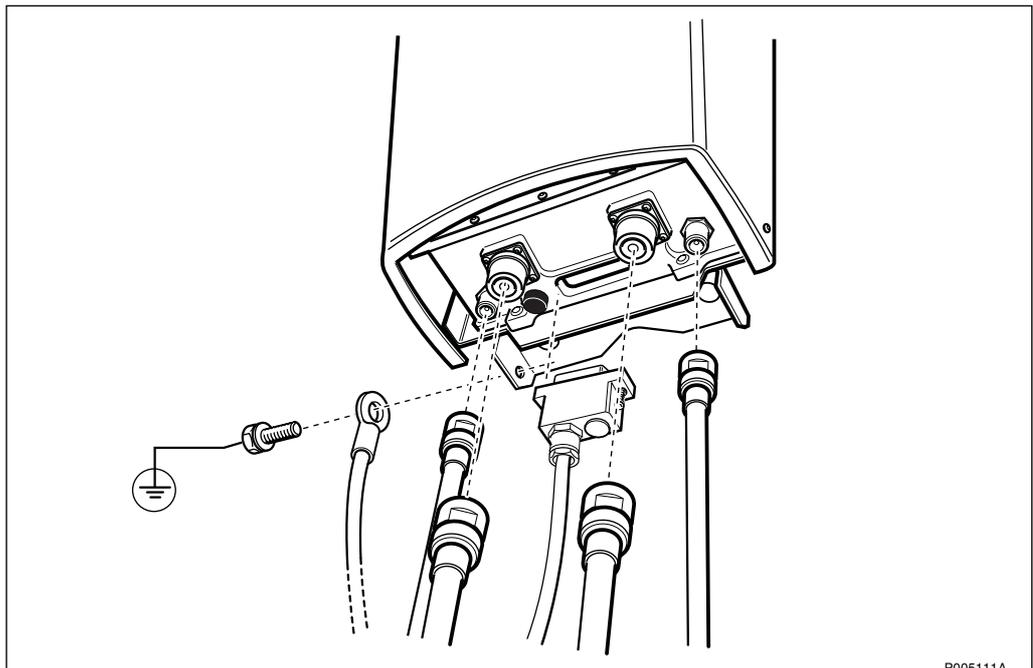
Figure 518 Loosening the cables of the CEU
