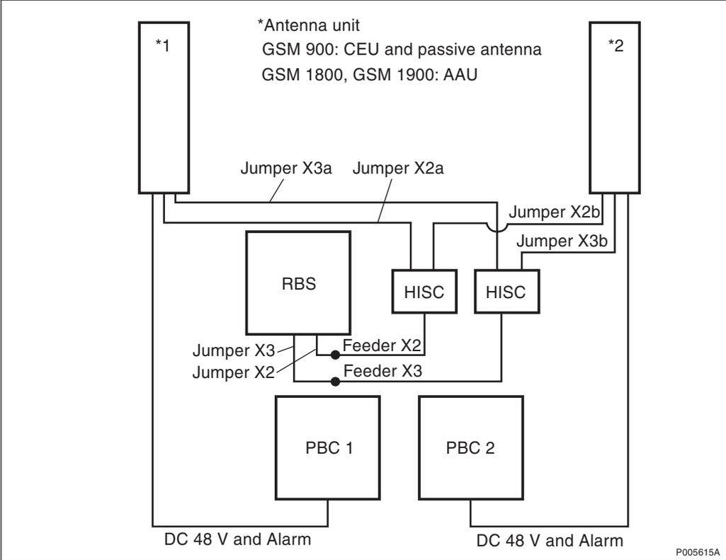
Figure 327 Highway configuration
