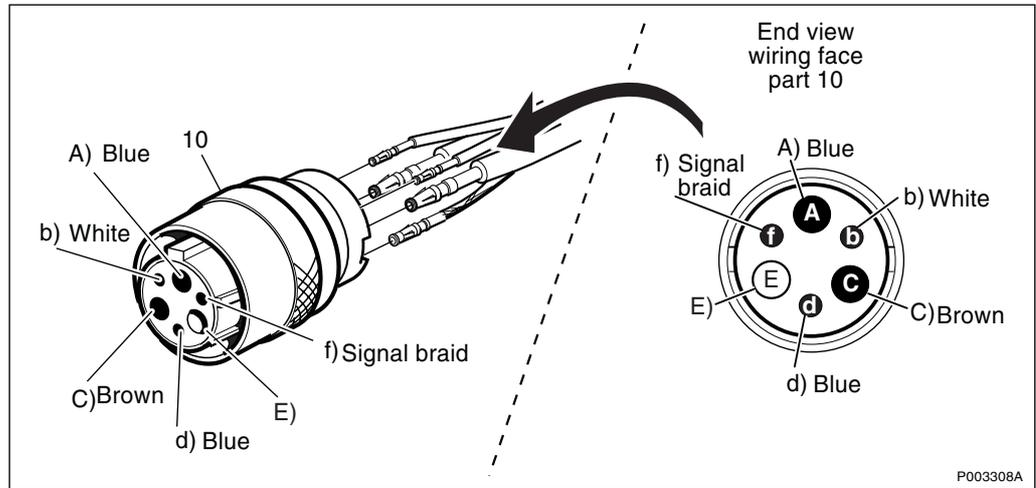
Figure 235 Connector pin overview
