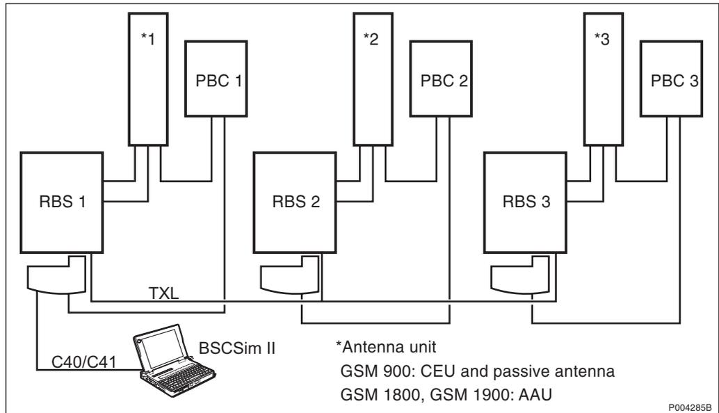
Figure 365 Test setup: 4 TRX and 6 TRX Configurations
