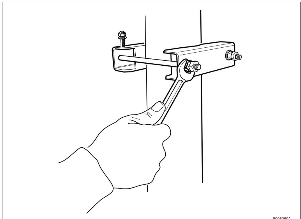
Figure 60 Fastening the upper mounting fixture
