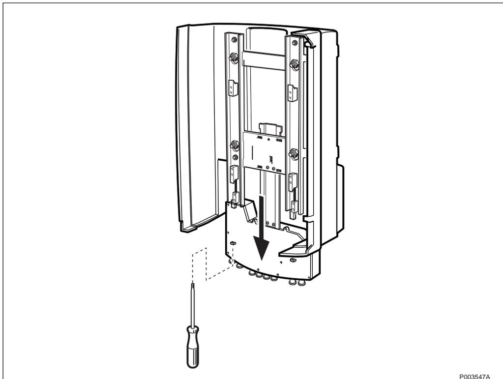
Figure 464 Releasing the interface box
