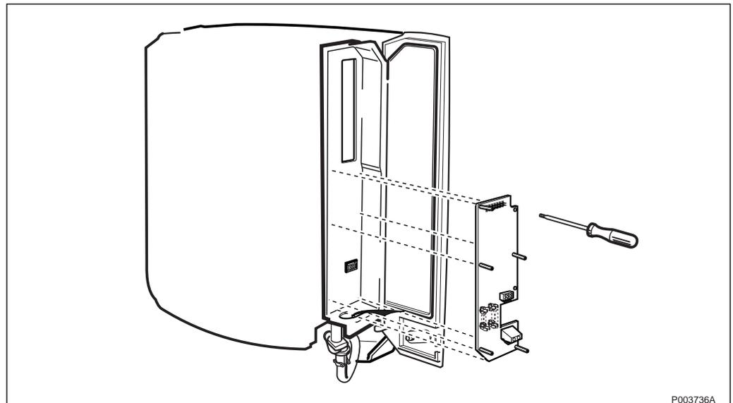
Figure 509 Removing the EMC board
