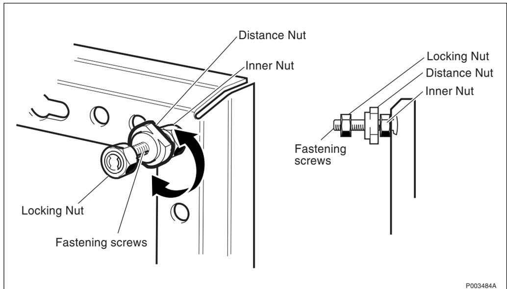
Figure 170 Adjusting the distance nuts
