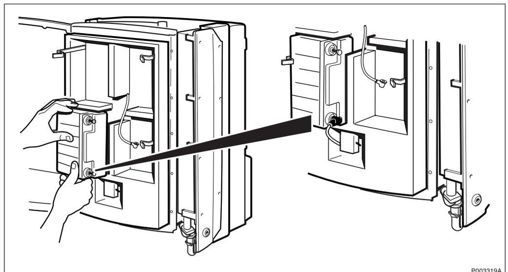
Figure 482 Installing battery 1
