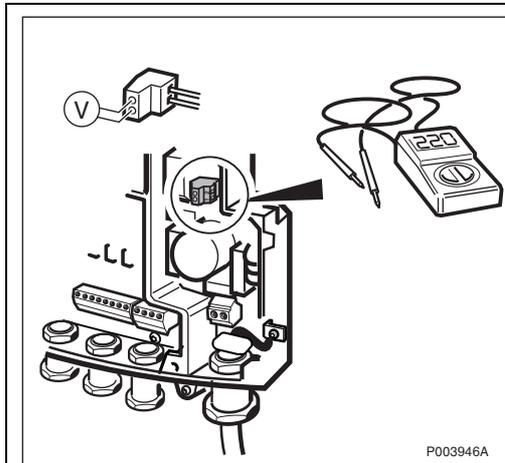
Measure that 115/230 V is present at the upper AC plinth on the AC-board, to verify that the AC-board is not faulty.
