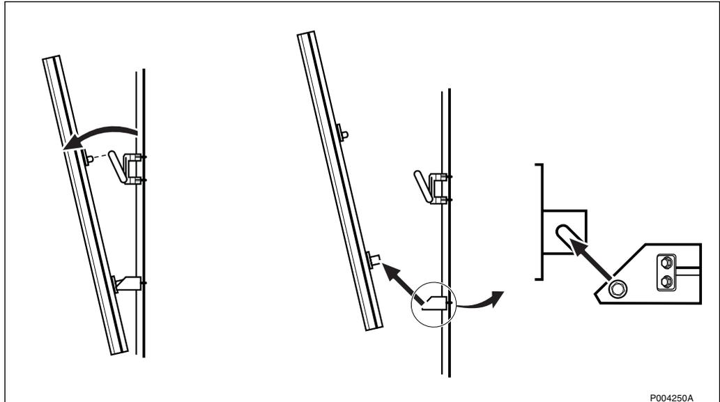
Figure 542 Lifting the antenna out of the mount while guiding it
