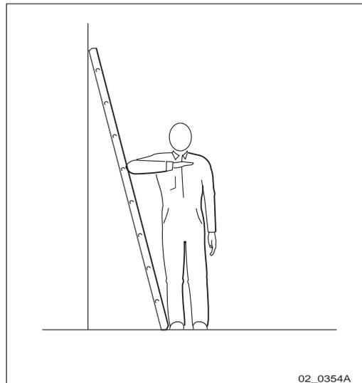
*Figure 9 Checking the angle*
