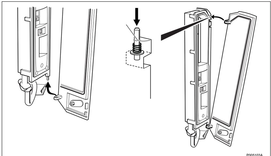
Figure 127 Mounting the installation box door
