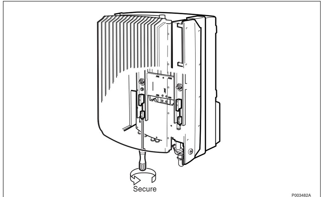
Figure 135 Securing the cabinet
