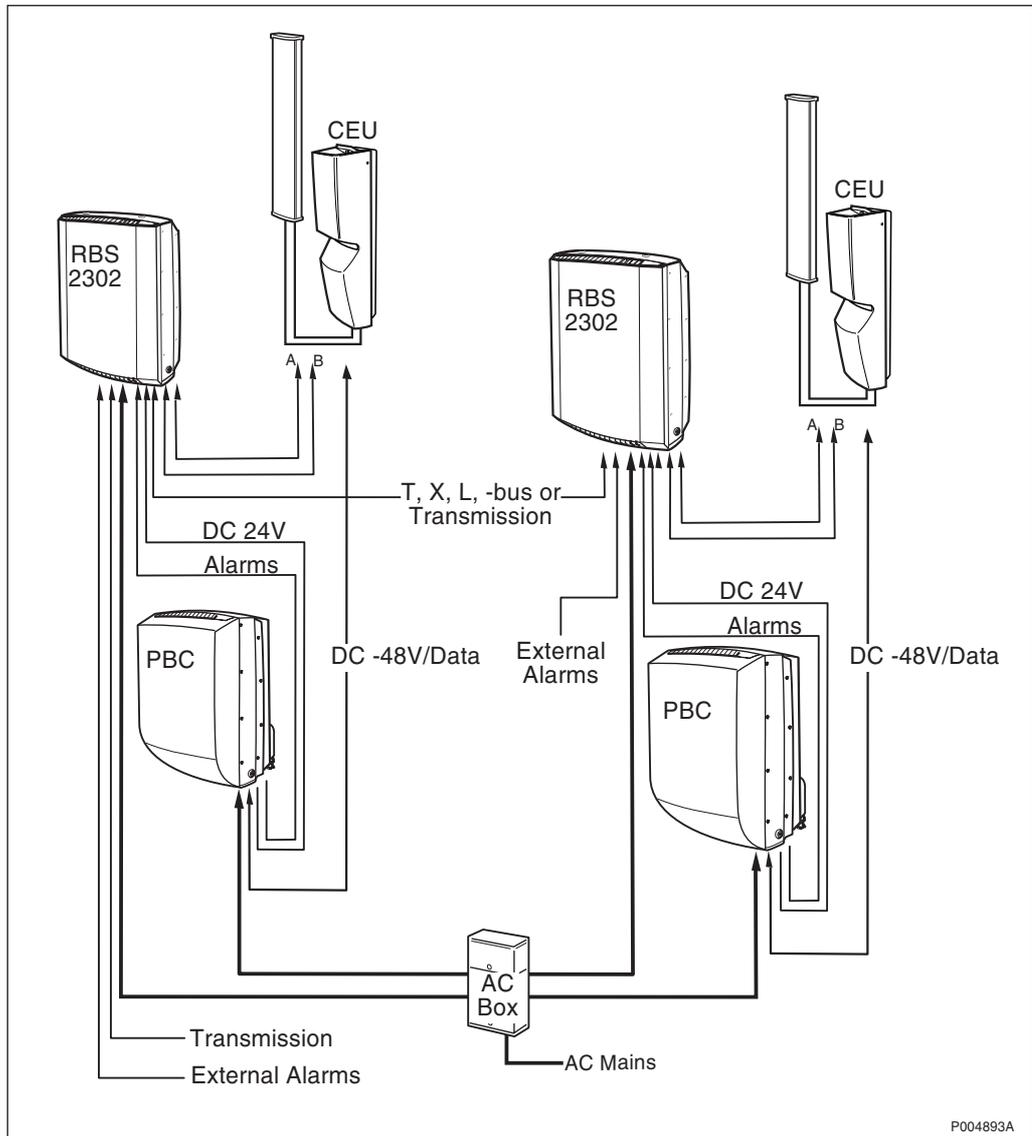
Figure 48 Configuration with 4 TRX
