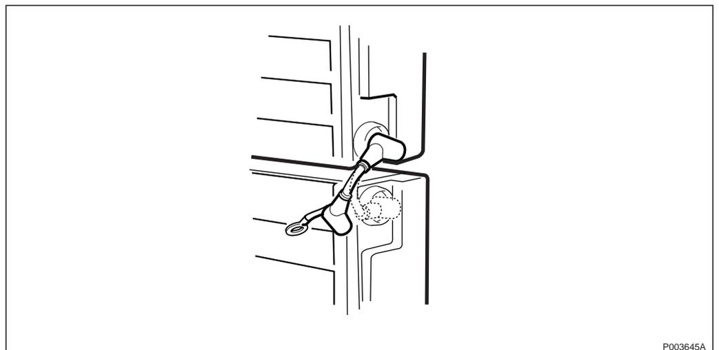
Figure 498 Disconnecting the minus-pole (-) on battery 1
