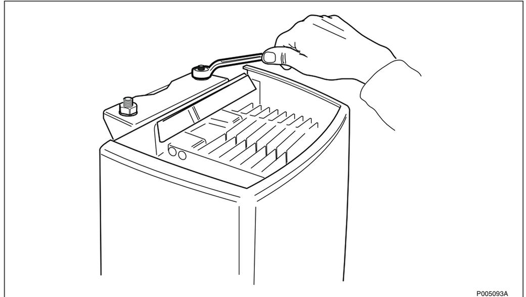
Figure 76 Fastening the CEU to the upper wall bracket
