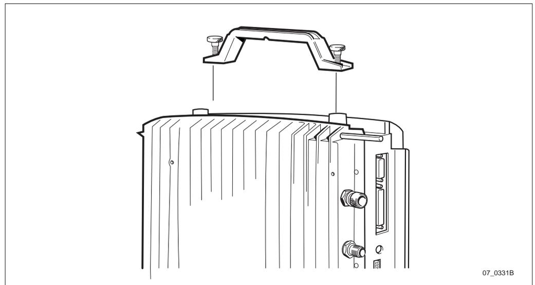
*Figure 427 Mounting the handle*
