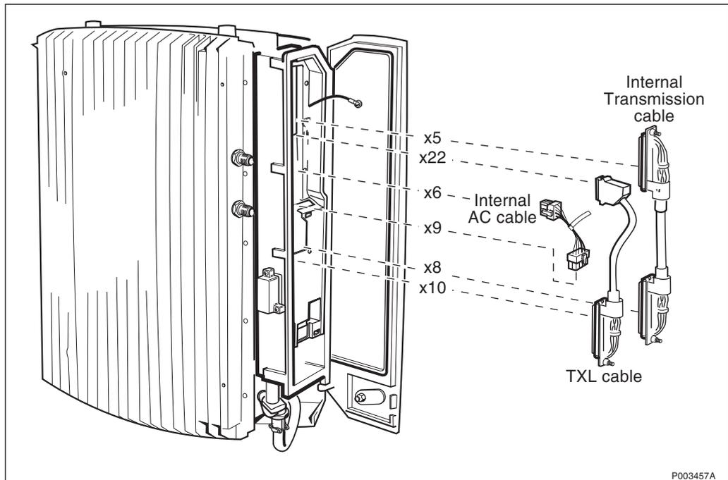
Figure 425 Internal cables
