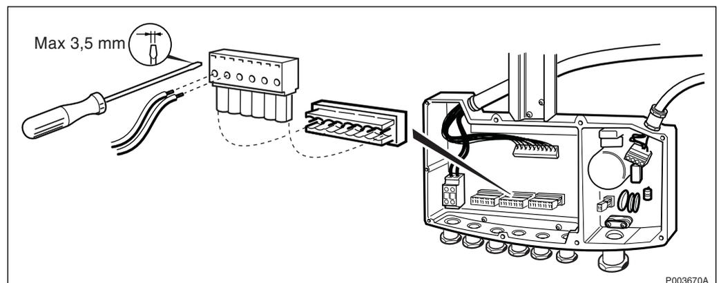
Figure 268 Loosening the termination block
