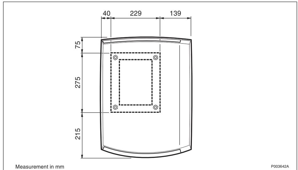
Figure 160 Mounting plate and equipment contour, front view
