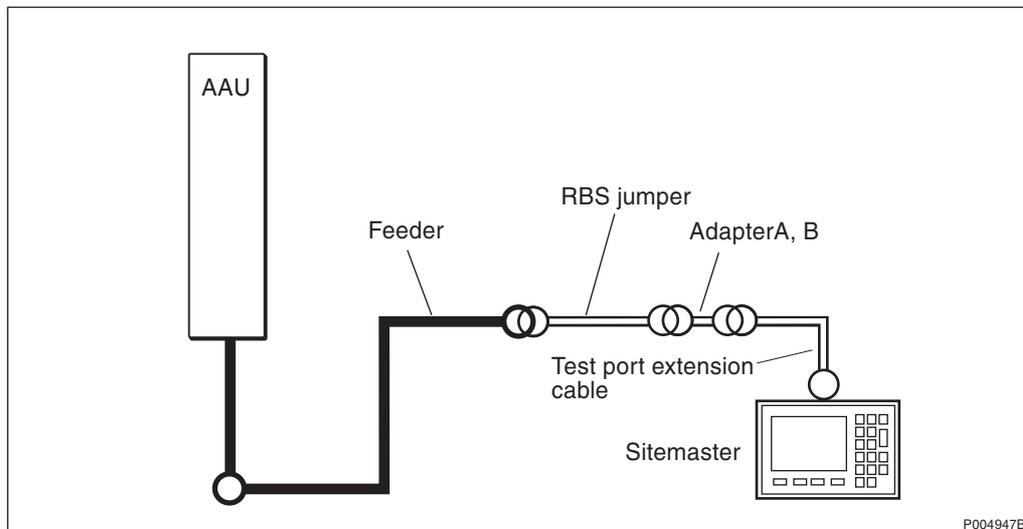
Figure 331 Test setup for GSM 1800, GSM 1900: Sector configuration with AAU
