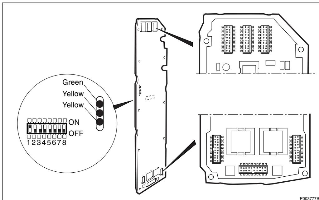
Figure 353 Location of DIP switches, LEDs and connectors
