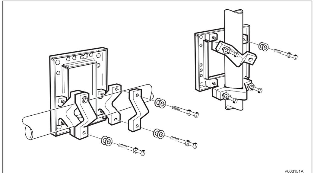
Figure 124 Placing the mounting plate correctly
