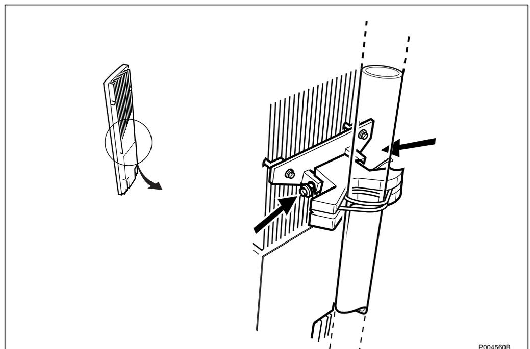
Figure 532 Releasing the two screws on the lower mount
