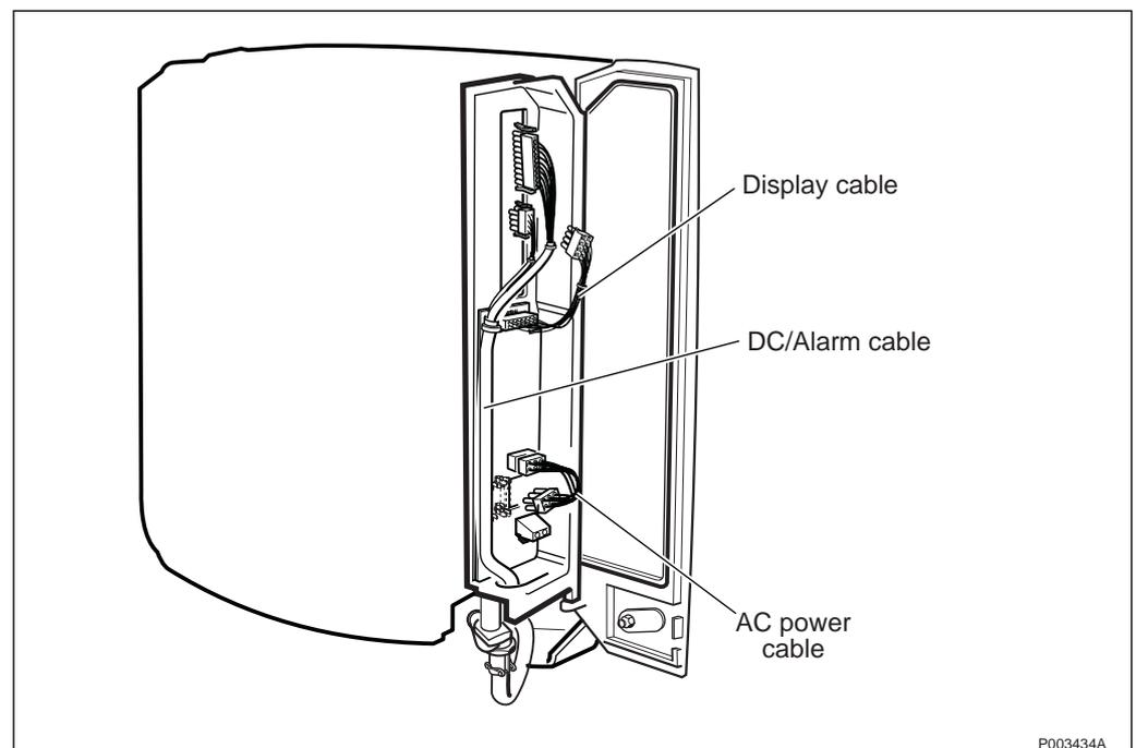
Figure 489 Loosening the AC cable and the Display cable
