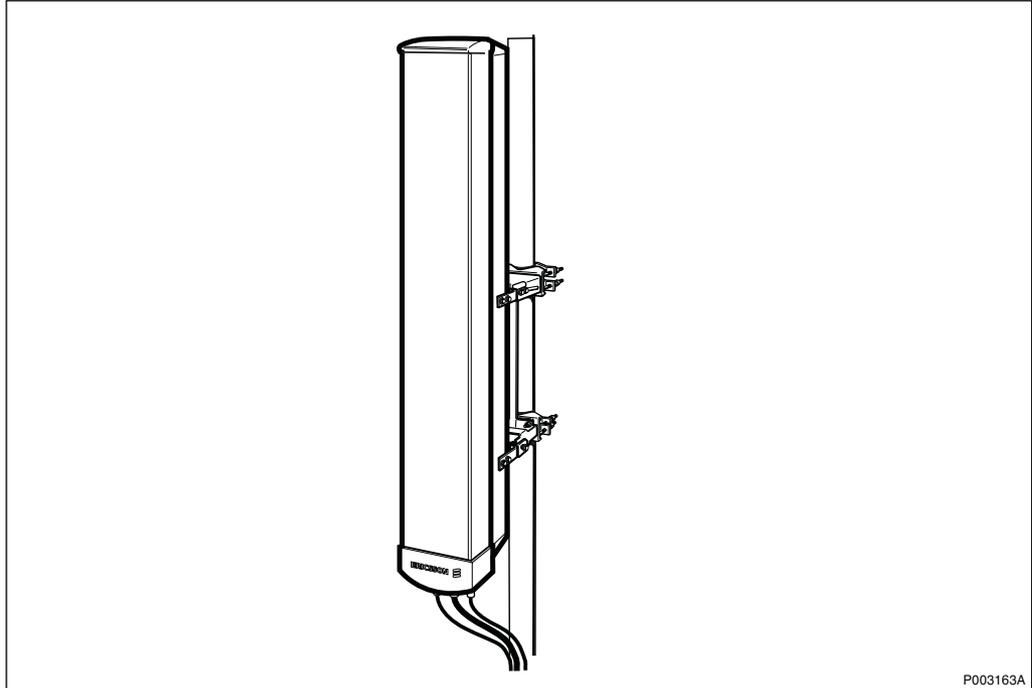
*Figure 78 The antenna mounted on a pole*
