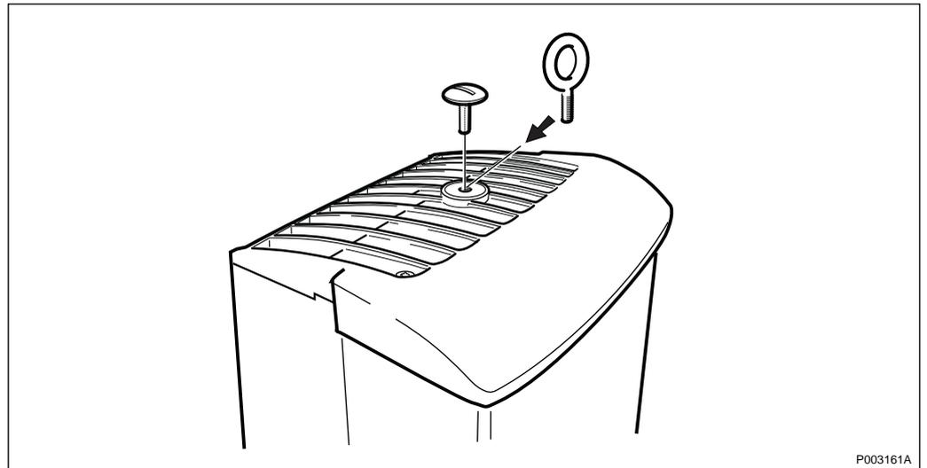
Figure 84 Preparing the upper end of the antenna for lift, by replacing the sealing plug with an eyebolt
