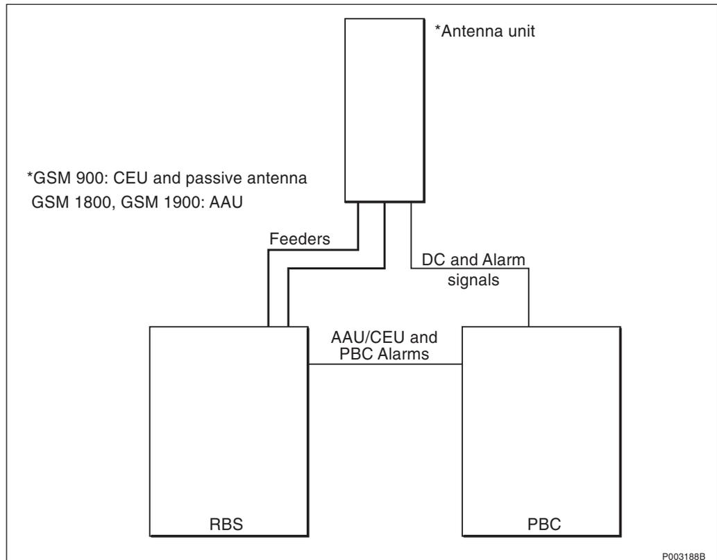
Figure 322 Overview of alarm system functions
