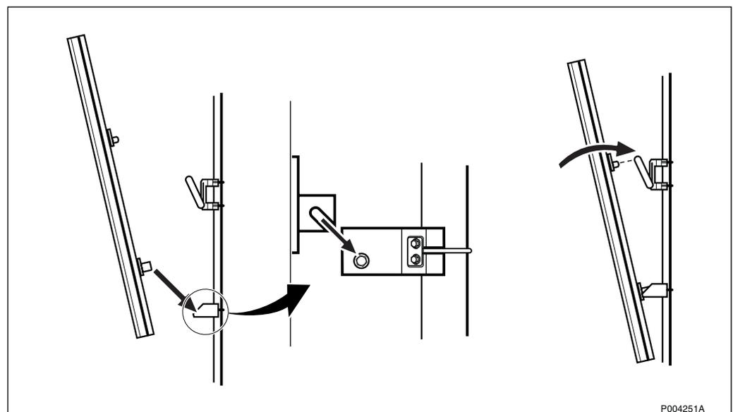
Figure 536 Sliding the antenna into the lower mount and tilt it up
