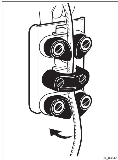
Figure 204 Fastening the rope
