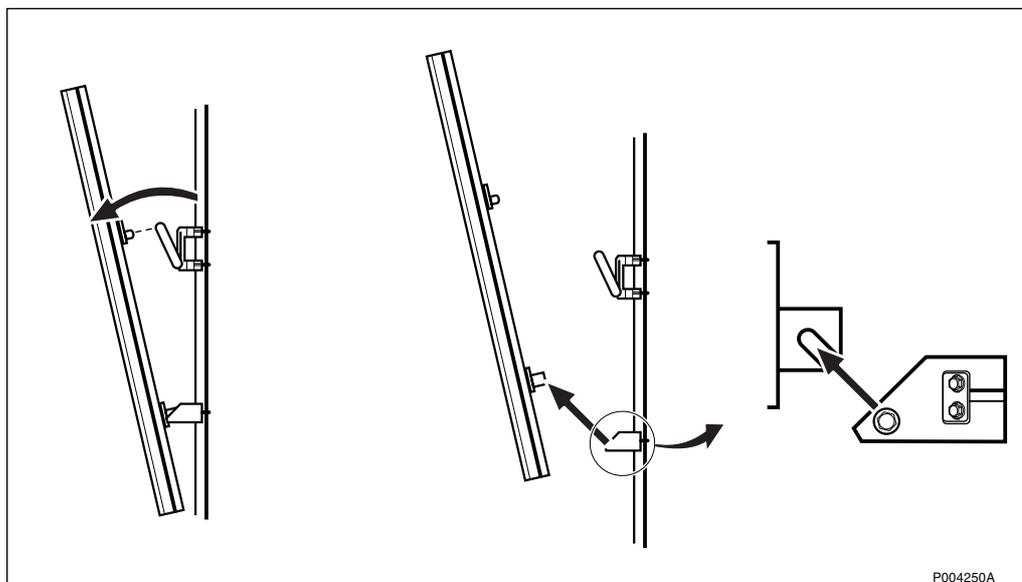
Figure 534 Lifting the antenna out of the mount while guiding it
