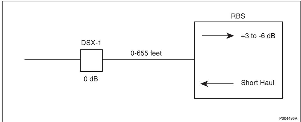
Figure 344 The Short Haul principle
