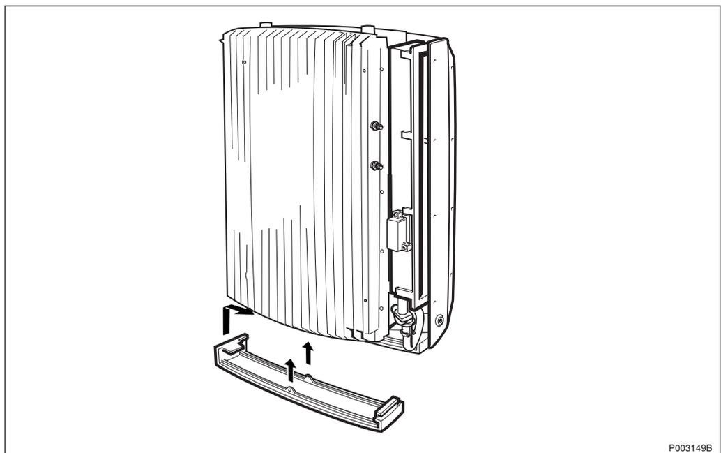
Figure 191 Hooking on the lower sunshield
