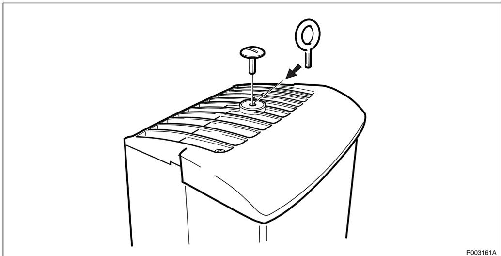
Figure 575 Lifting eye bolt (top)
