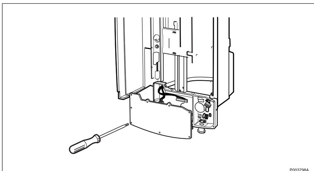
Figure 465 Loosening the interface box cover
