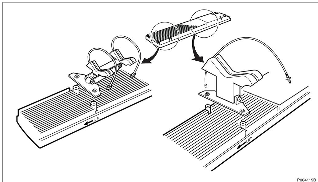
Figure 100 Attaching the upper and lower mounting fixture to the antenna (500 W EIRP)
