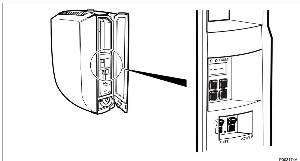
Figure 389 Location of the control panel in the PBC
