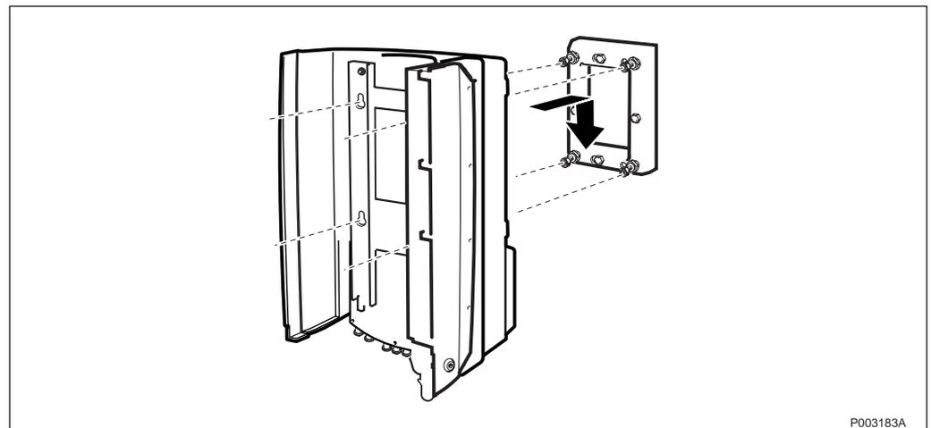
Figure 125 Mounting the mounting base on the mounting plate
