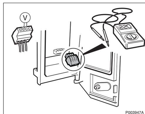
Measure that 115/230 V is present at the incoming AC plinth on the connection board, to verify that the cables are not faulty.
