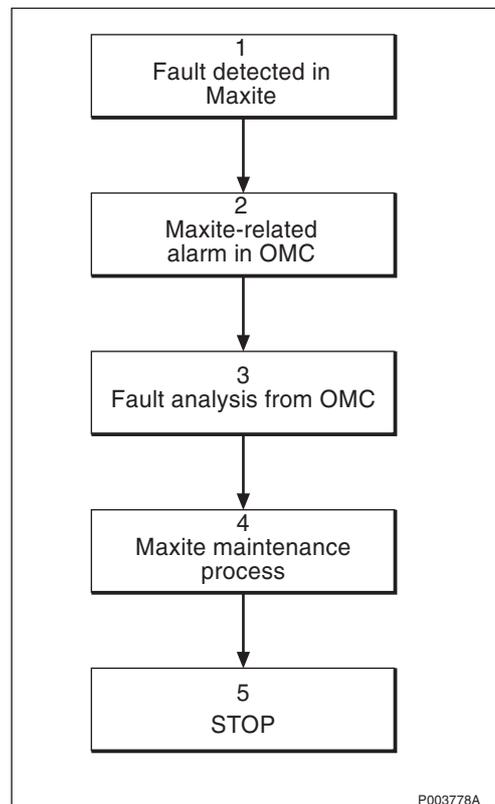
Figure 383 Fault handling workflow
