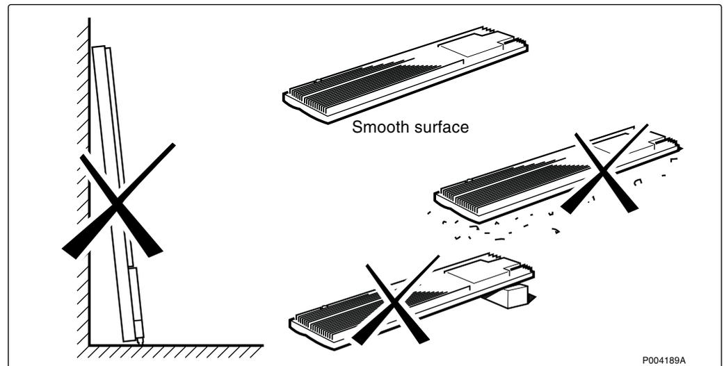
Figure 99 Handle the antenna with care (Antenna 1250 W EIRP shown)
