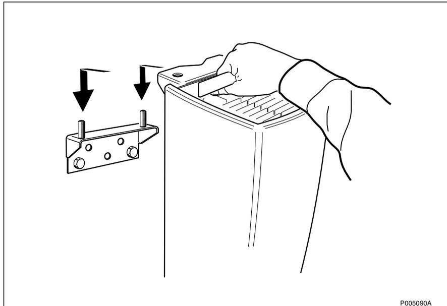
Figure 74 Placing the CEU on the upper wall bracket
