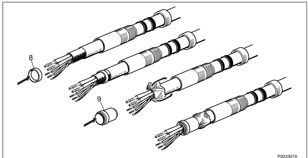
*Figure 234 Fit the clamping ring and clamping cone*
