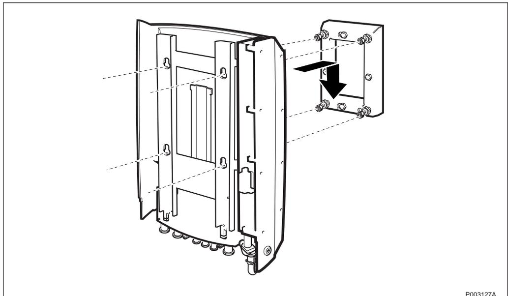
Figure 553 Mounting base and mounting plate
