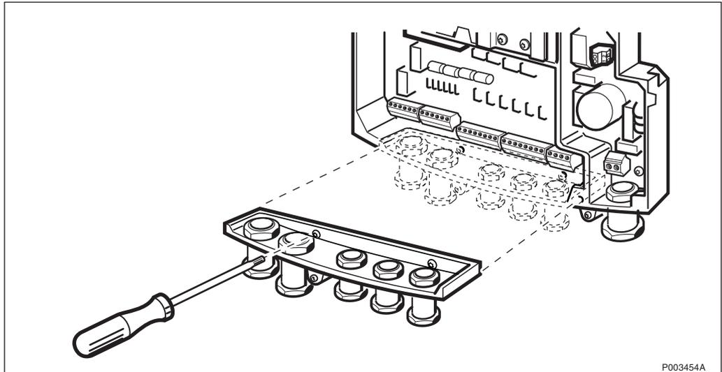
Figure 283 Loosening the gland plate
