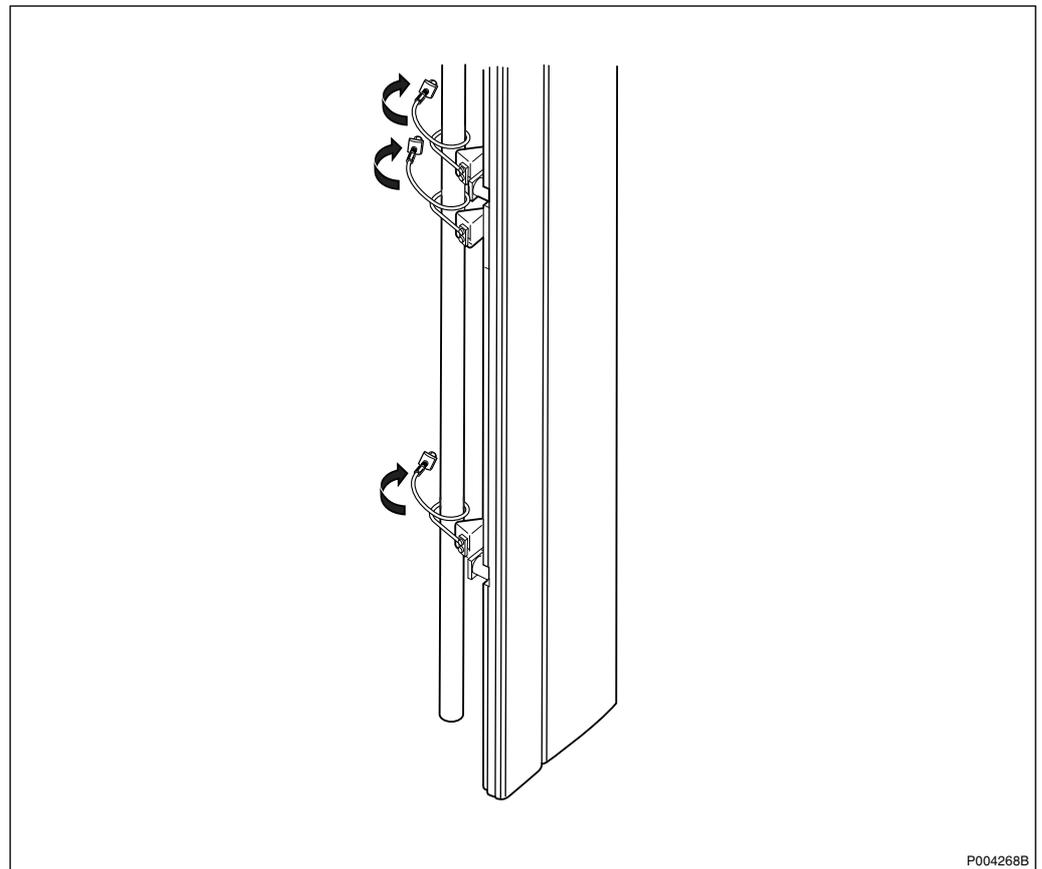
*Figure 107 Pulling the cables around the pole (Antenna 1250 W EIRP shown)*
