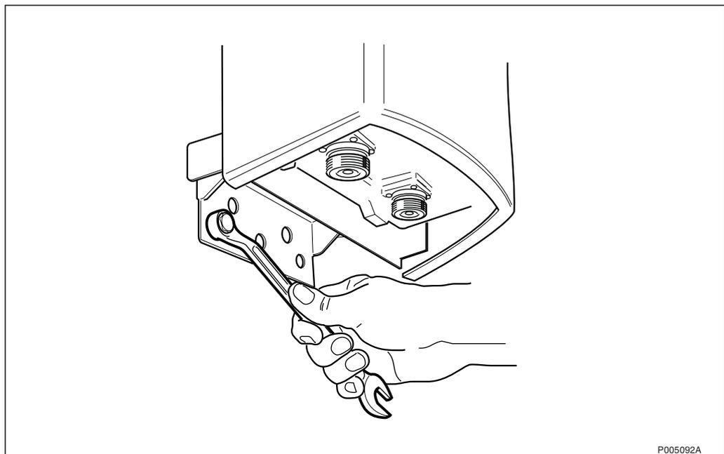
Figure 75 Fastening the lower wall bracket to the wall
