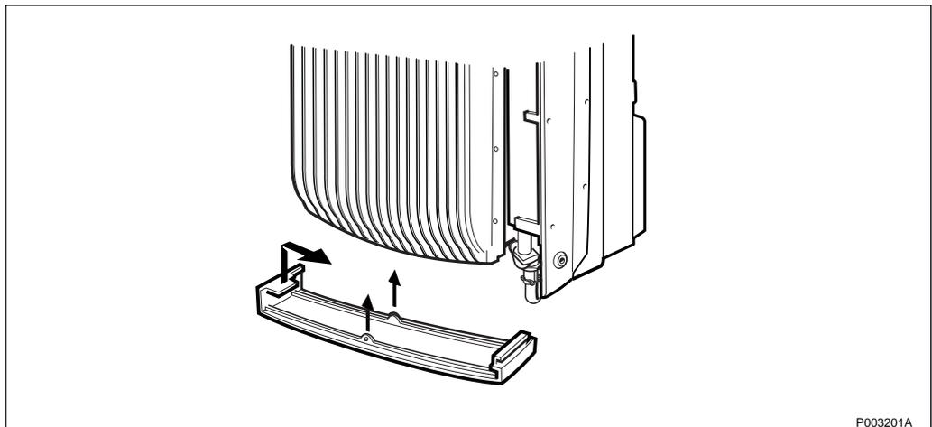
Figure 154 Hooking on the lower sunshield
