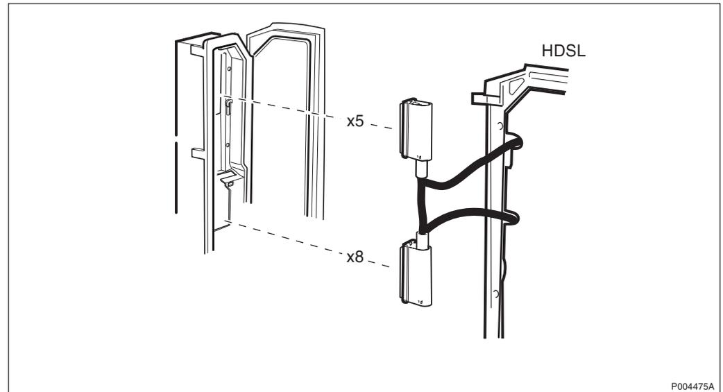
Figure 402 Disconnecting the cables
