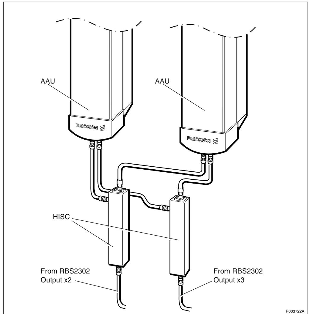
Figure 257 Connection of the HISC (Highway Splitter Combiner)
