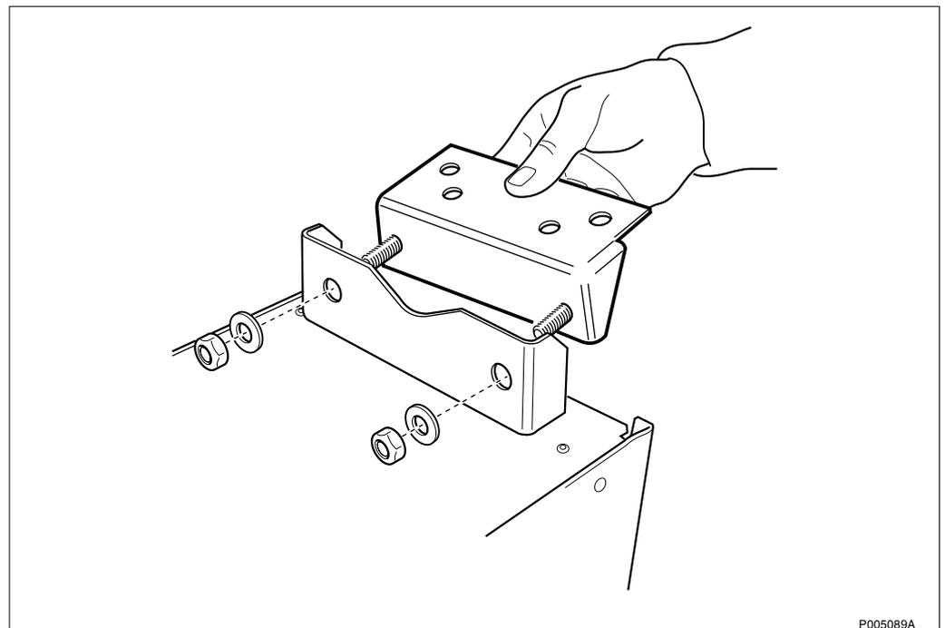
Figure 69 Mounting the lower mounting bracket on the CEU
