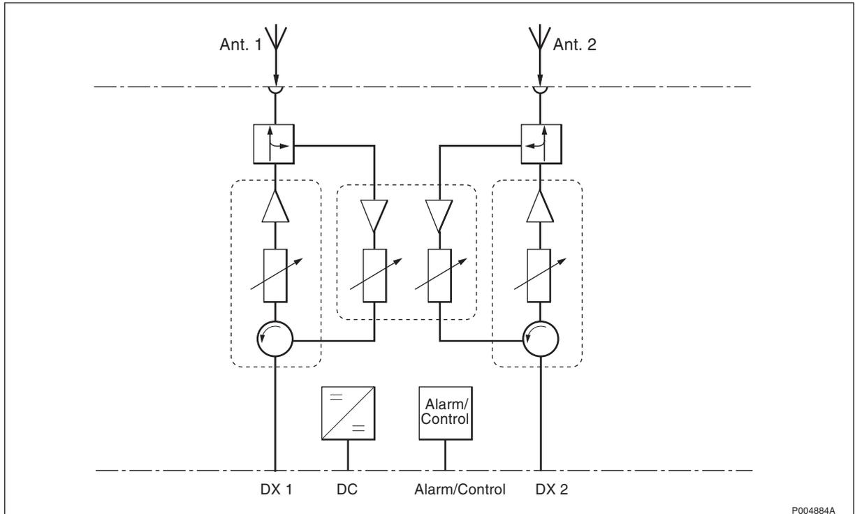
Figure 44 Block diagram Coverage Extension Unit for GSM 900
