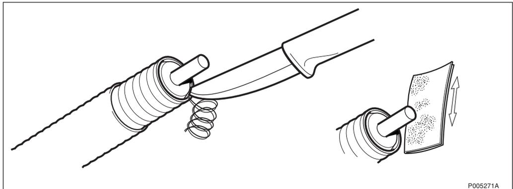
Figure 253 Loosening the dielectricum from the copper mantle and cleaning of the inner conductor with abrasive paper
