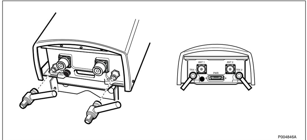
Figure 572 Connection of lightning protector
