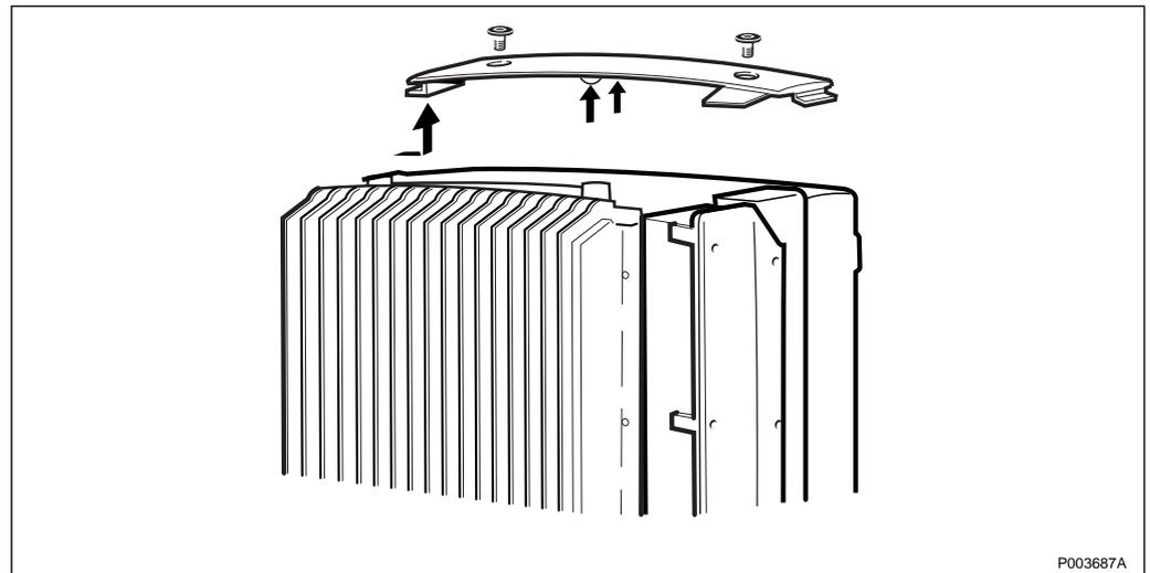
Figure 463 Replacing the upper sunshield
