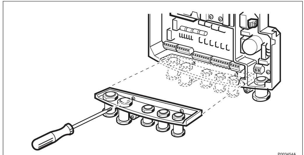
Figure 416 Loosening the gland plate
