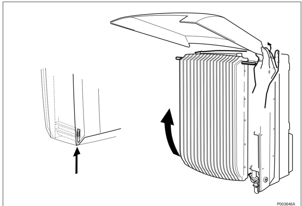
Figure 460 Replacing the front sunshield
