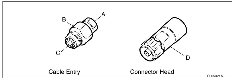
Figure 254 Connector parts
