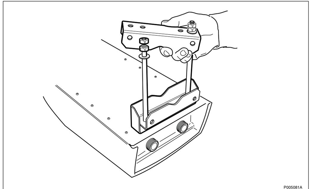
Figure 61 Preparing the CEU for hoisting
