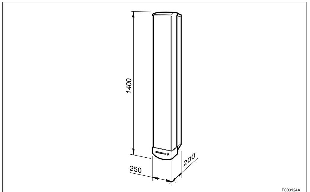
Figure 577 Active Antenna Unit dimensions
