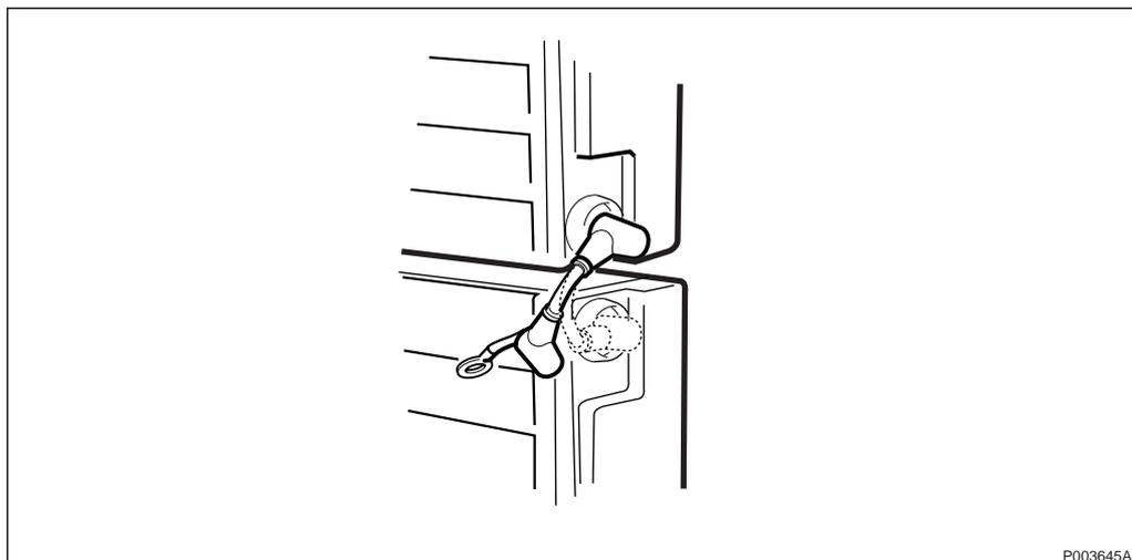
Figure 483 Installing battery 2
