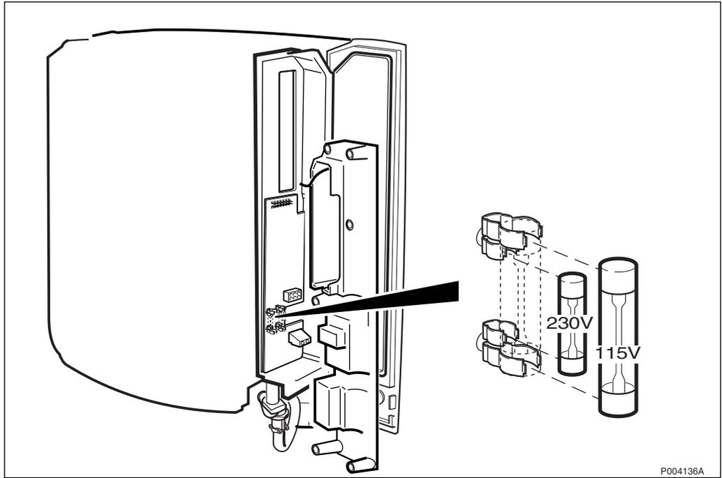
Figure 130 Installing the fuses
