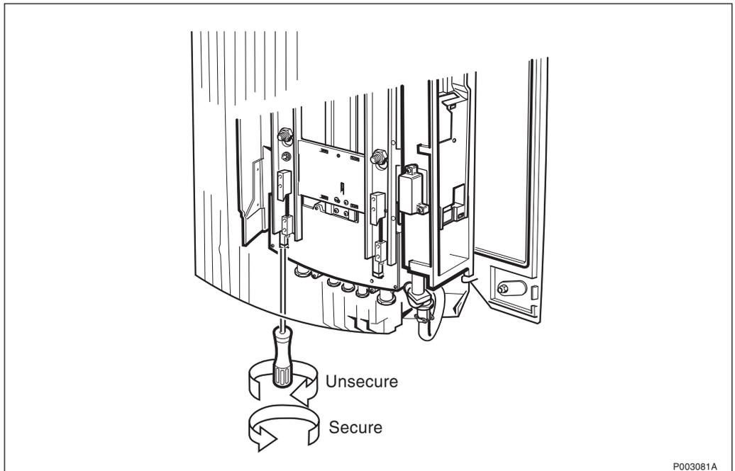
Figure 209 Securing the cabinet
