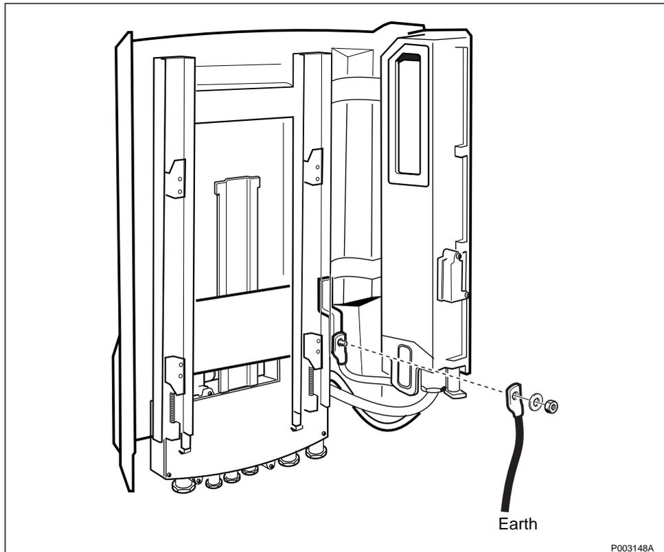
Figure 177 Connecting earth and lightning protection
