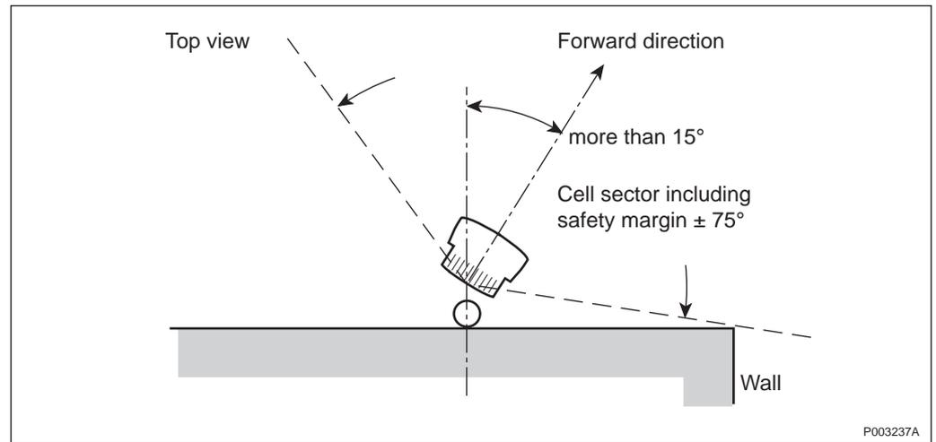
Figure 24 Antennas close to corner
