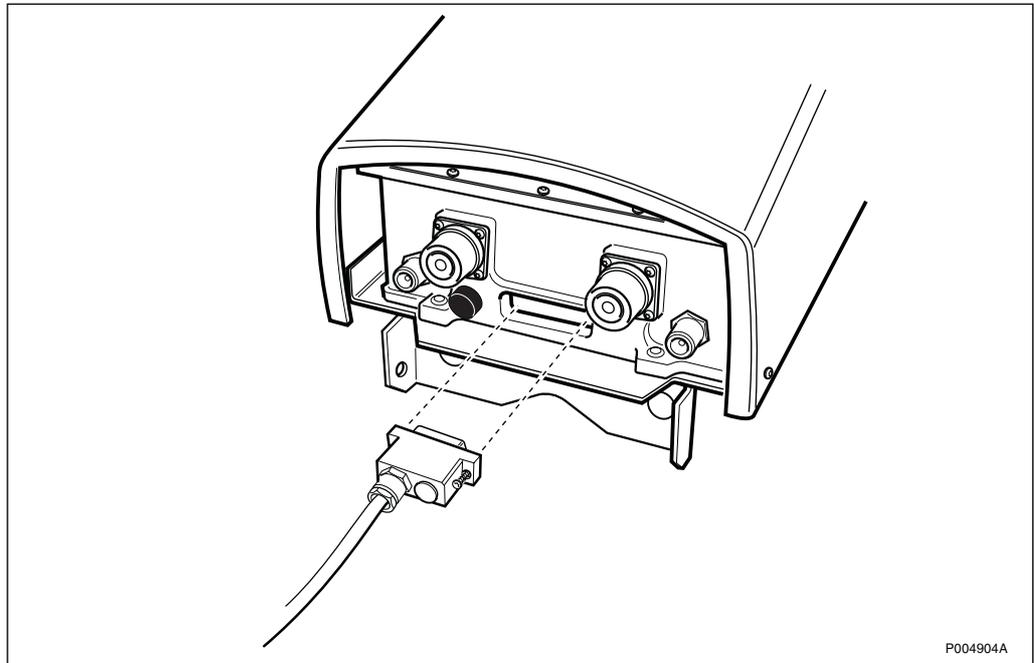
*Figure 218 Connecting the DC/Data-cable*
