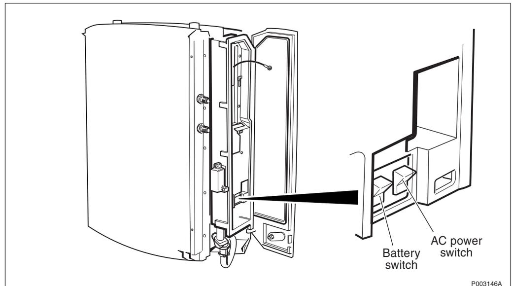
Figure 336 Power switches in the RBS
