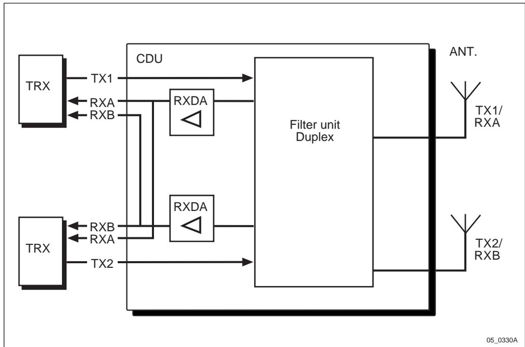
Figure 45 Block diagram of RBS 2302
