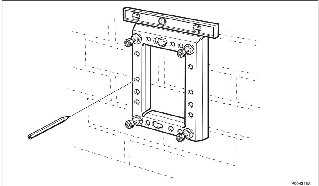
Figure 162 Marking the rest of the holes
