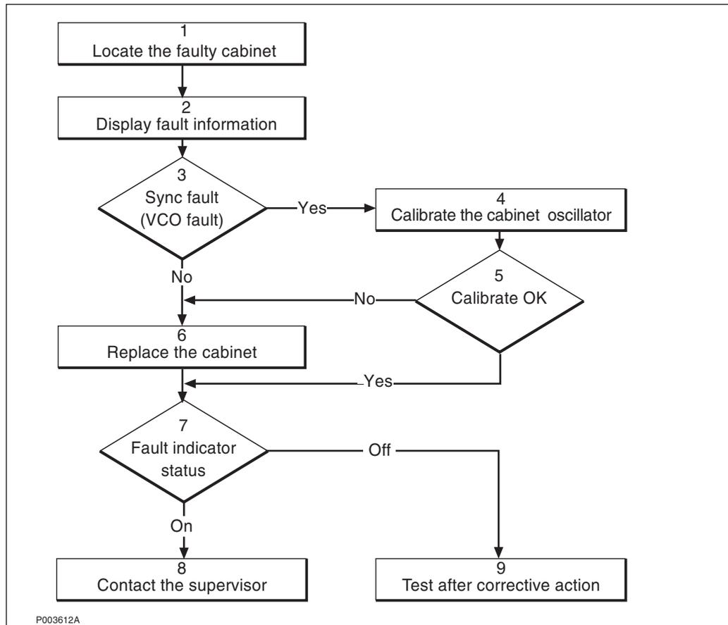
Figure 458 Internal Synchronization fault localization
