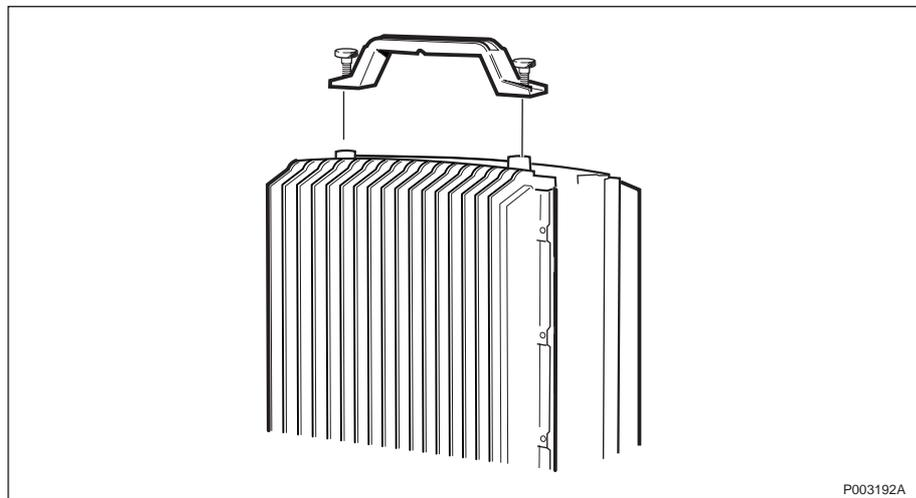
Figure 133 Mounting the lifting handle
