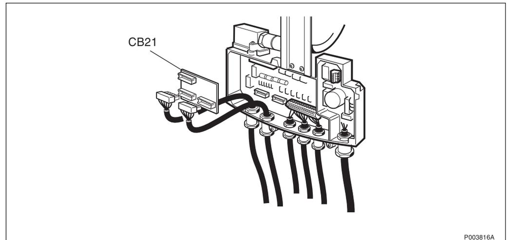
Figure 447 Dismounting the CB21 contact
