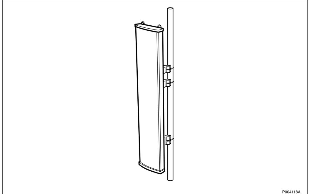
Figure 579 Active Antenna Unit 500 W EIRP for GSM 1900
