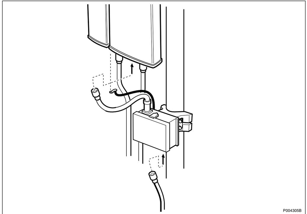
Figure 239 Connecting the ALPU (Antenna Lightning Protection Unit)
