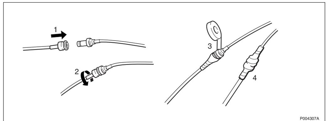
Figure 299 Connecting the and sealing the TNC connector for the PCM 75  $\Omega$  cable
