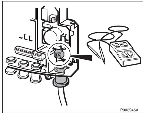
4. Measure with a multimeter to verify that the PBC has correct voltage on the AC terminal in the interface box.
