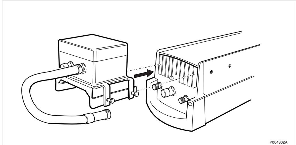
Figure 92 Sliding the DC/Data Lightning Protector into the cooling flanges
