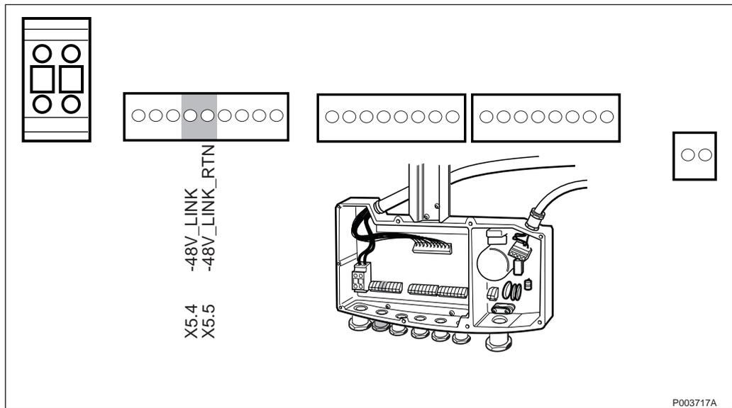
*Figure 279* -48 V DC power supply to Radio Link equipment
