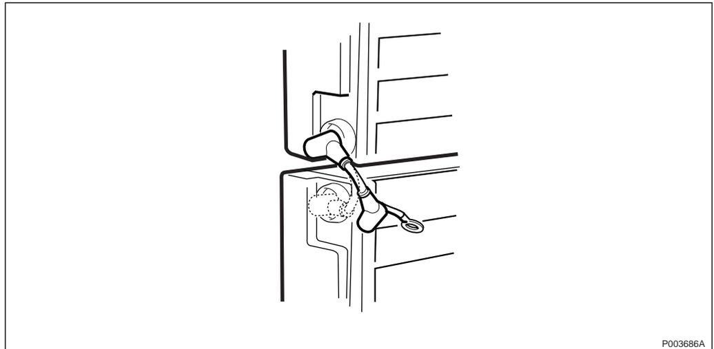
Figure 475 Disconnecting the plus-pole (+) of battery 3
