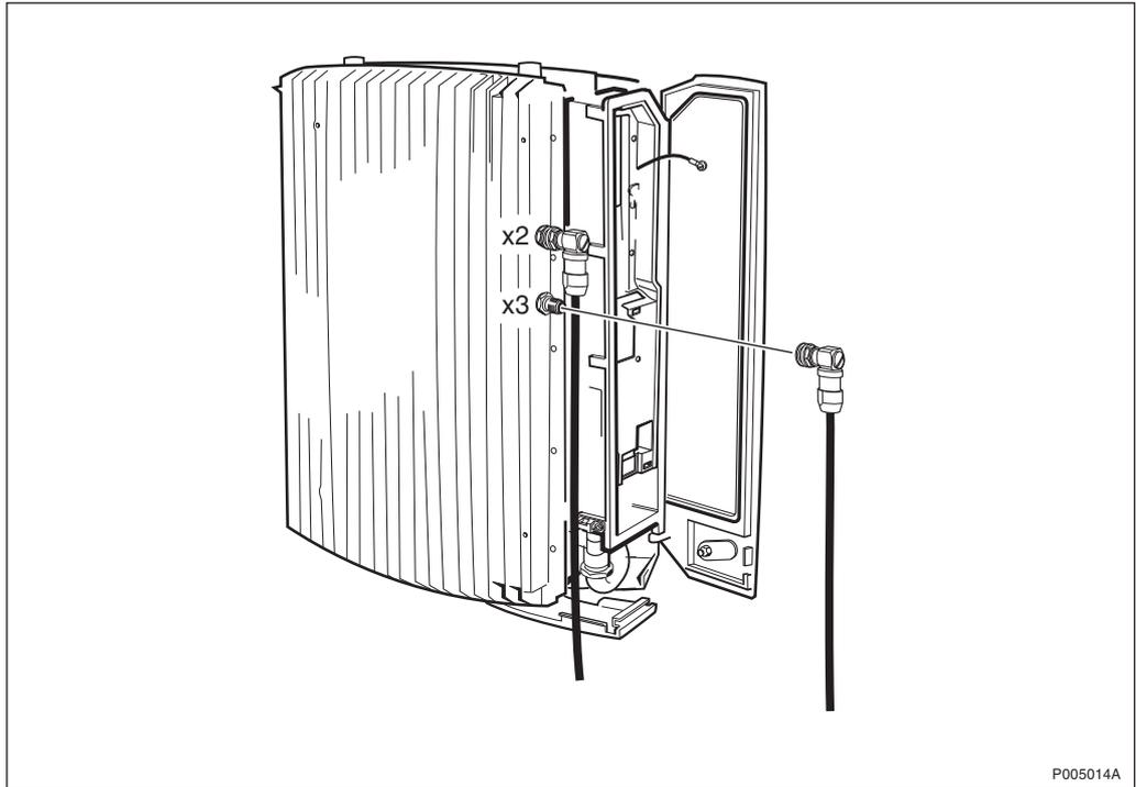
Figure 311 Connecting the antenna jumper cable to the RBS
