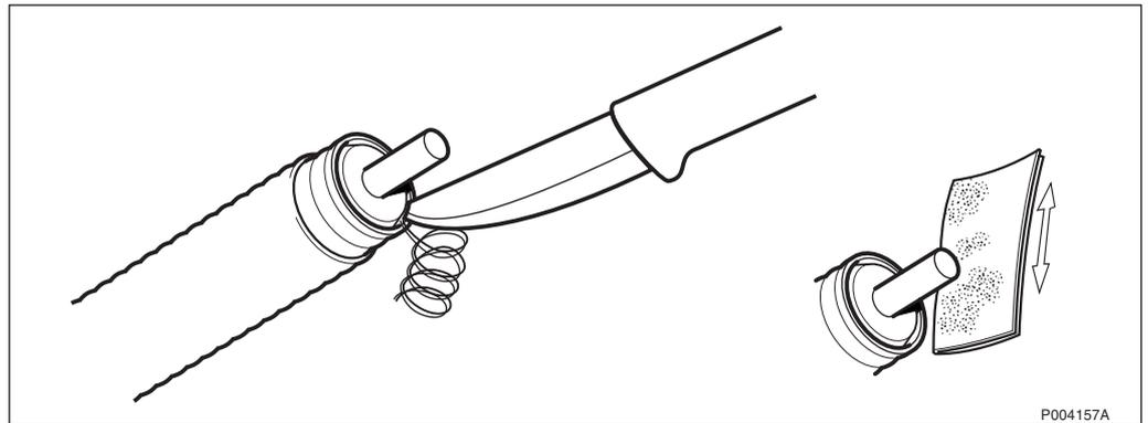
Figure 243 Loosening the dielectricum from the copper mantle
