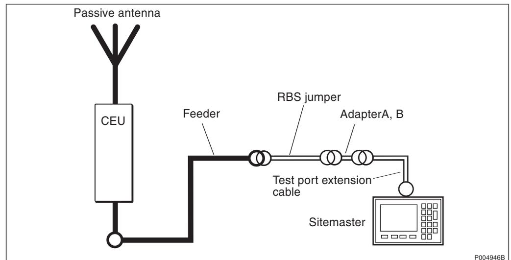
Figure 330 Test setup for GSM 900: Sector configuration with CEU and passive antenna
