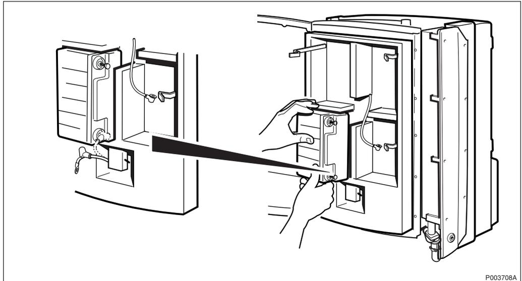
Figure 479 Disconnecting the plus-pole (+) of battery 1
