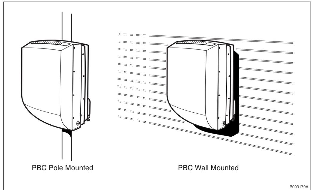
Figure 112 Installation alternatives
