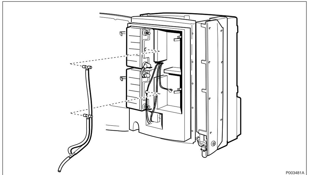
Figure 497 Removing the ventilation hoses
