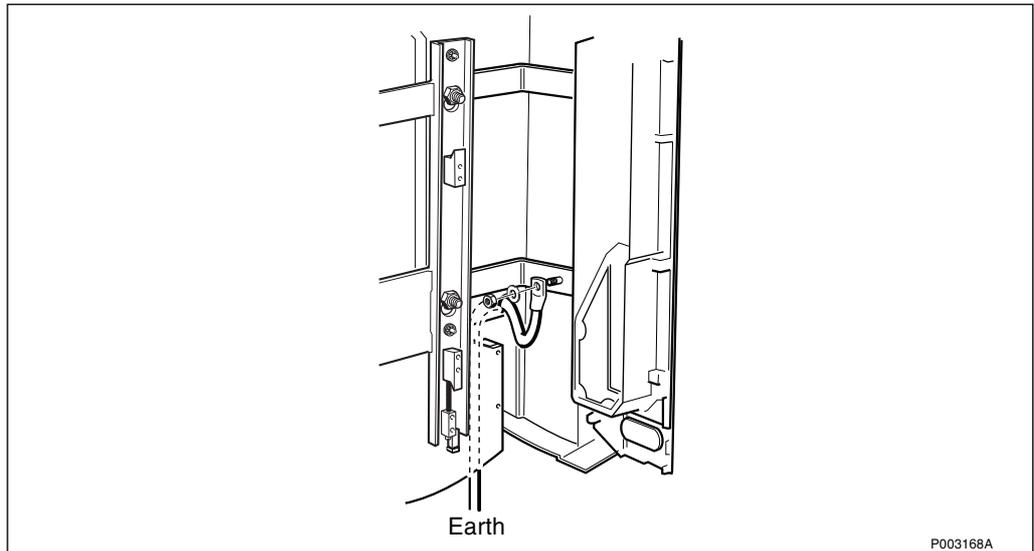
Figure 131 Connecting earth and lightning protection
