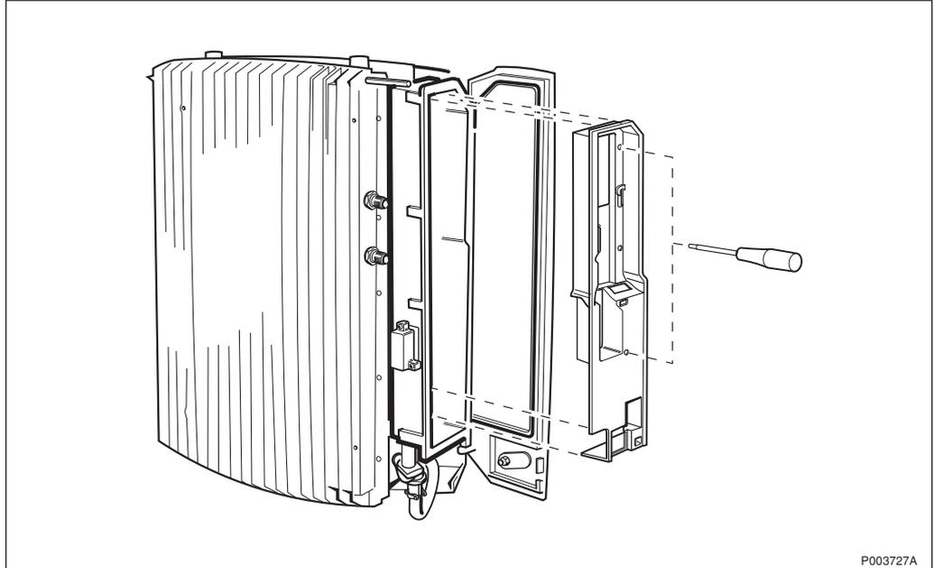
Figure 440 Removing the inner protective cover
