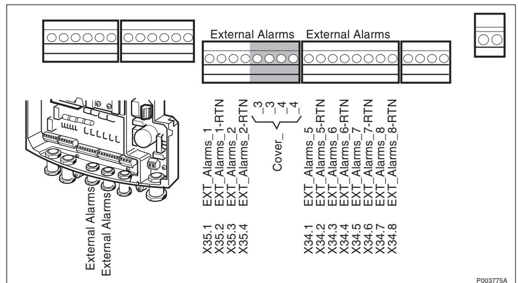
Figure 307 Covering of External Alarms
