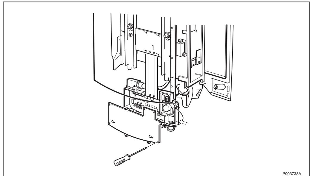
Figure 449 Loosening the interface box cover
