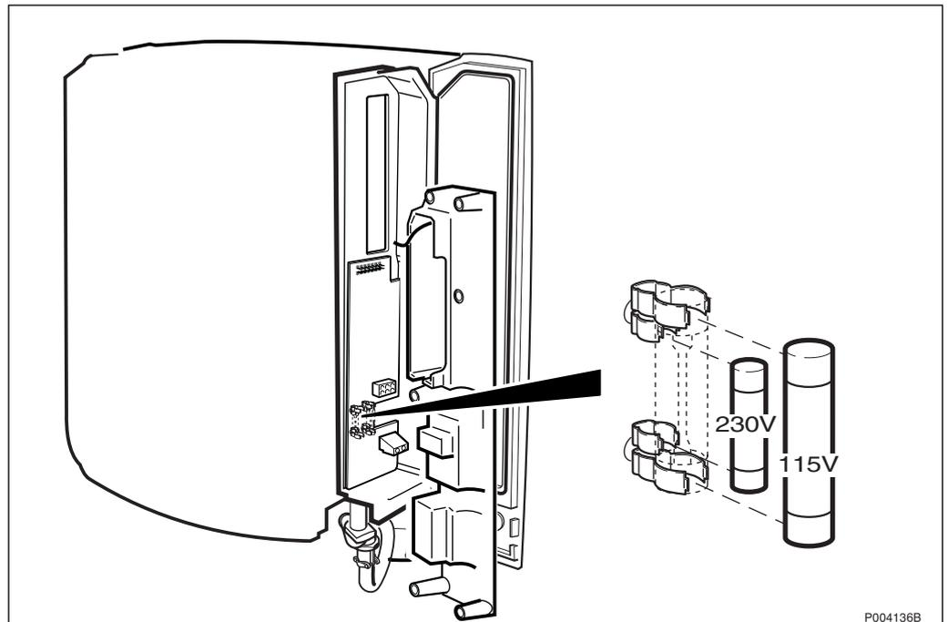
Figure 504 Replacing the fuses
