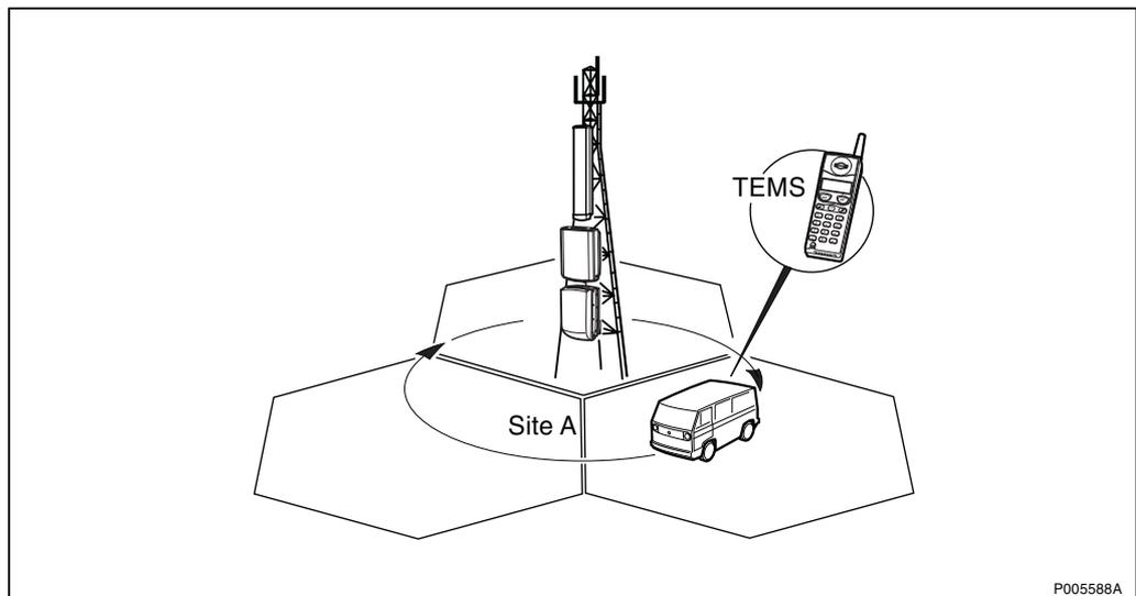
Figure 374 A drive test for checking that the call is handed over between the cells
