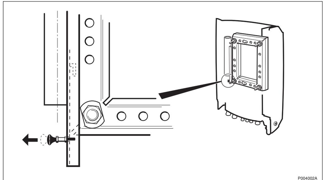
Figure 199 Locking pin position
