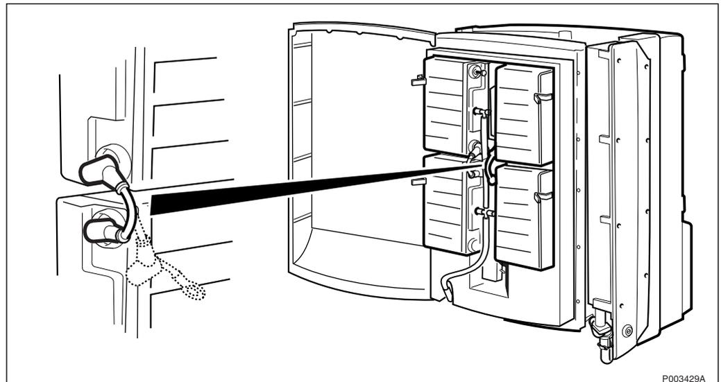
Figure 485 Connecting battery 3 and 4
