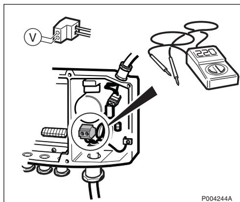
Measure with a voltage meter that 115/230 V is present at the incoming AC plinth on the AC board in the interface box.
