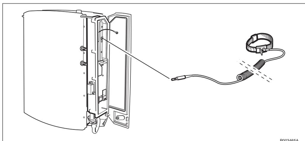
Figure 444 Connecting the ESD wrist strap
