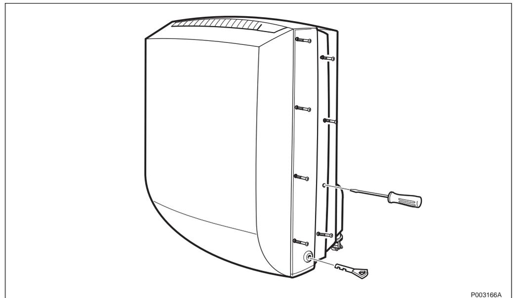
*Figure 469* Opening the installation box door
