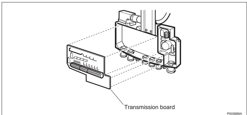
Figure 446 Loosening the transmission board
