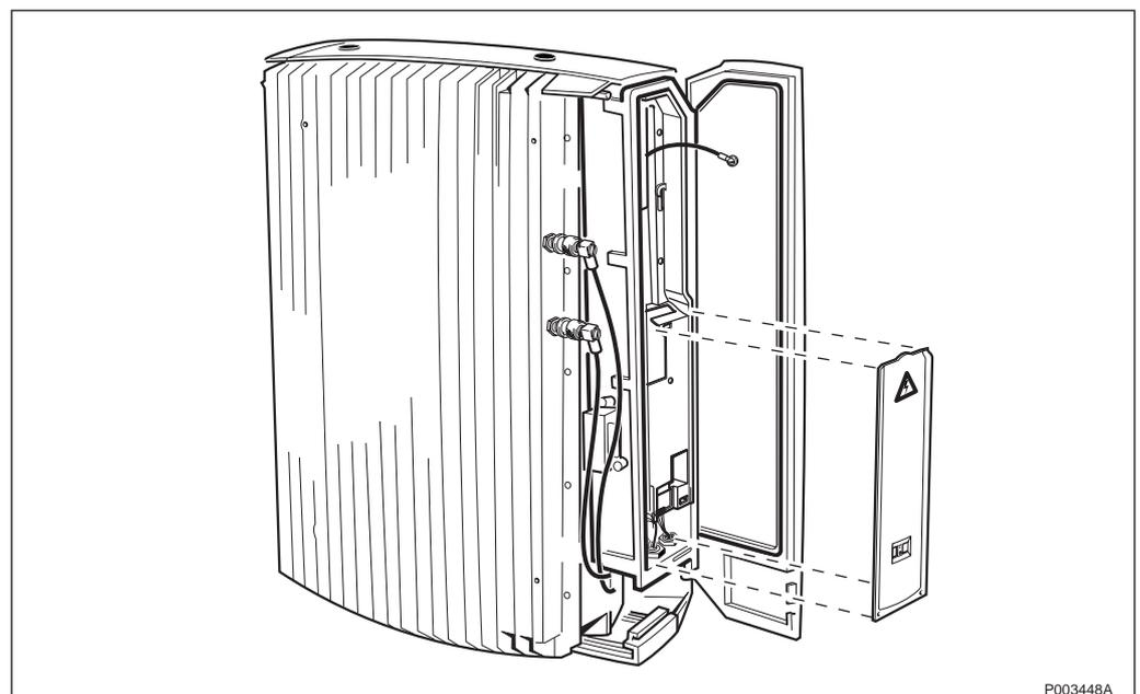
*Figure 434 Removing the outer protective cover*
