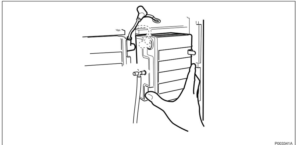
Figure 149 Connecting battery 2 and 4
