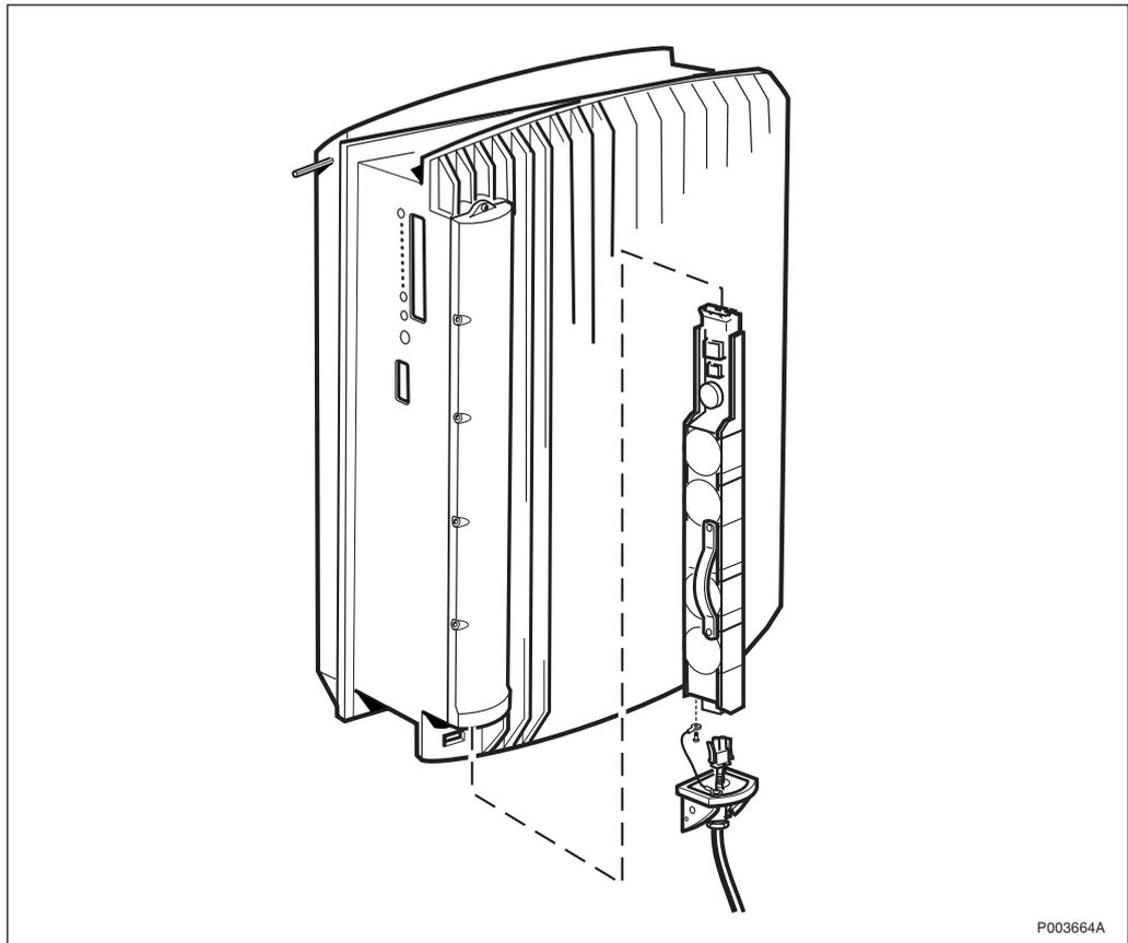
Figure 431 Replacing the PSA
