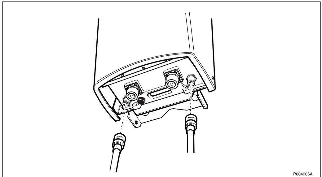
Figure 220 Connection of the Antenna Feeder Cables
