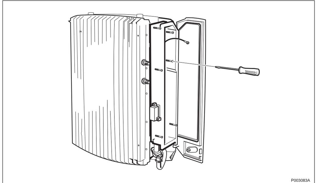
Figure 182 Fastening the installation box
