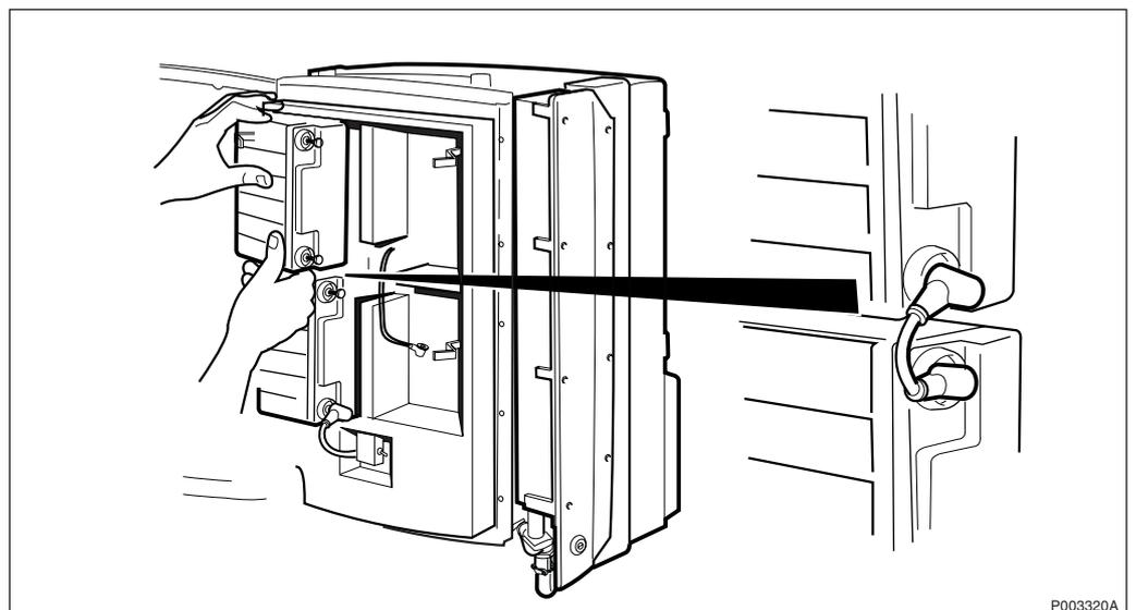
Figure 144 Connecting battery 1 and 2
