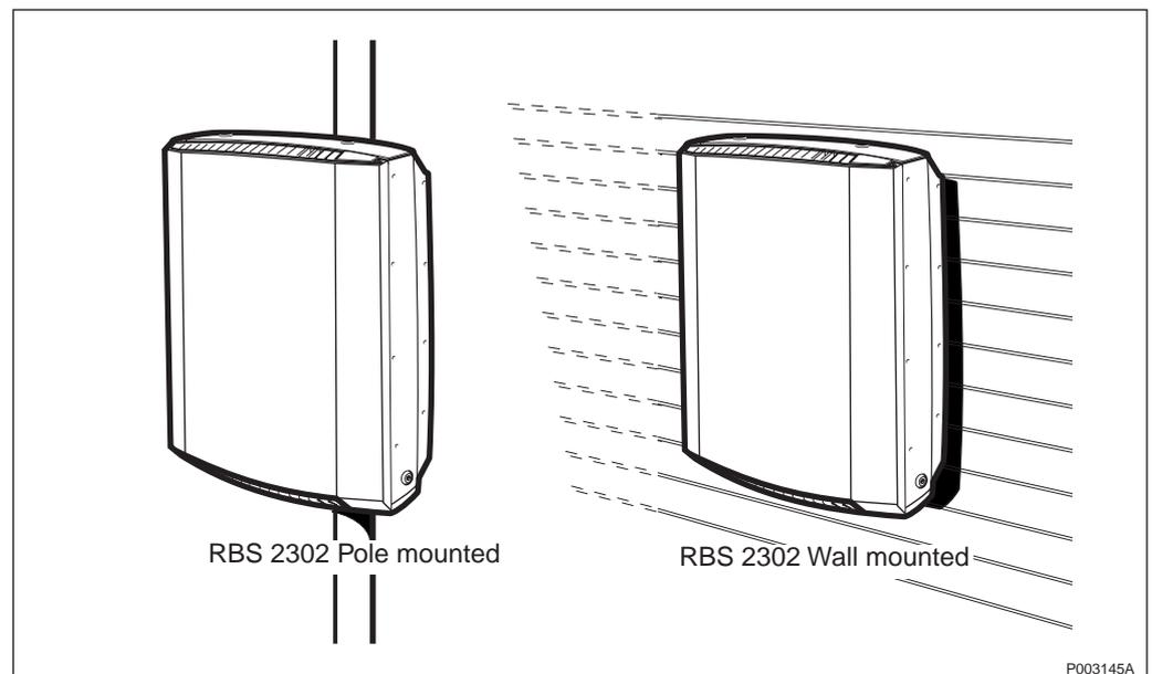
Figure 156 Installation alternatives
