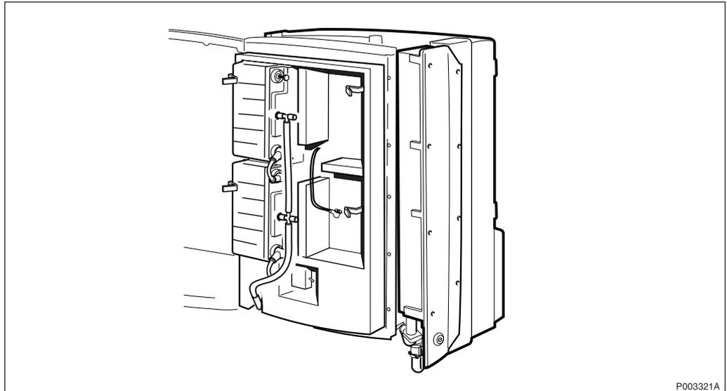
Figure 145 Connecting the ventilation hose
