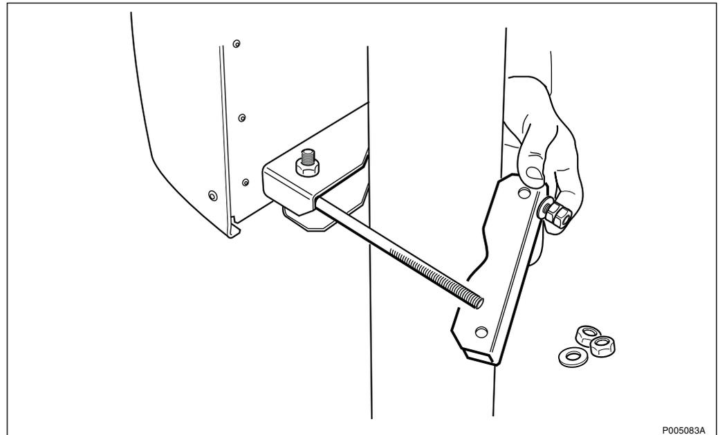
Figure 64 Putting the loose end of the lower mounting fixture clamp in place
