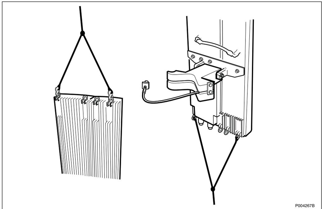
Figure 106 Upper lifting shackles and lower control shackles, antenna 1250 W EIRP
