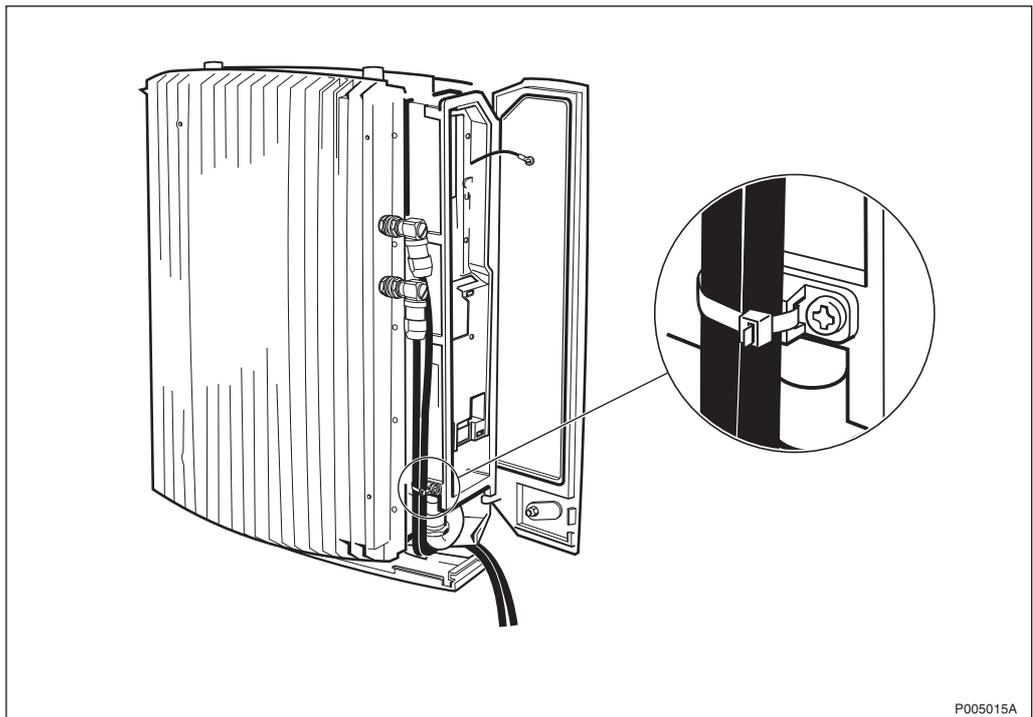
Figure 312 Installation of jumper cable
