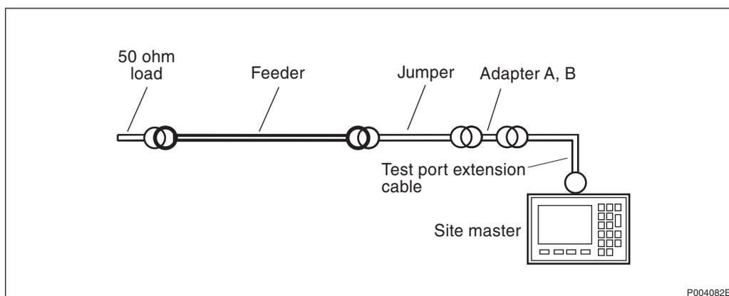
Figure 332 Test setup, Highway configuration
