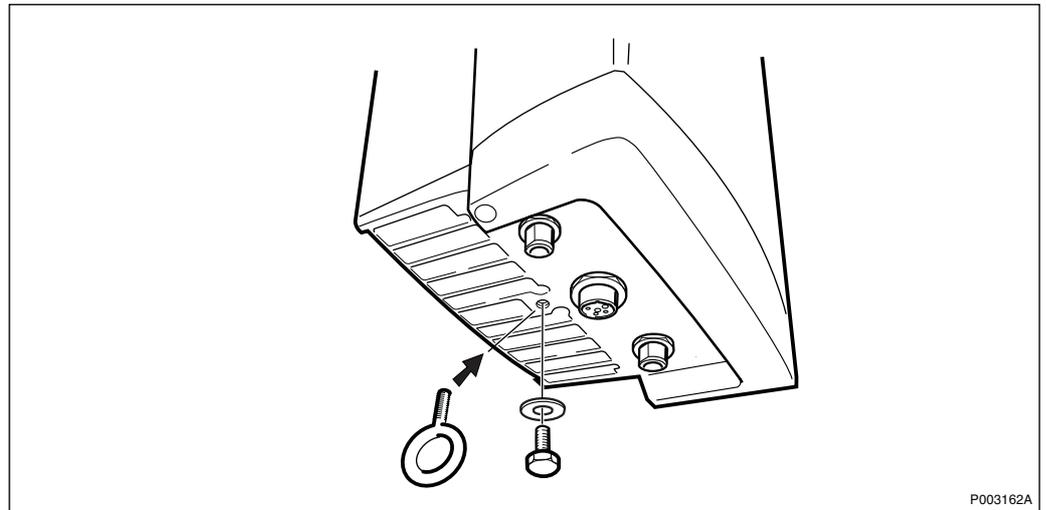
Figure 576 Lifting eye bolt (bottom)
