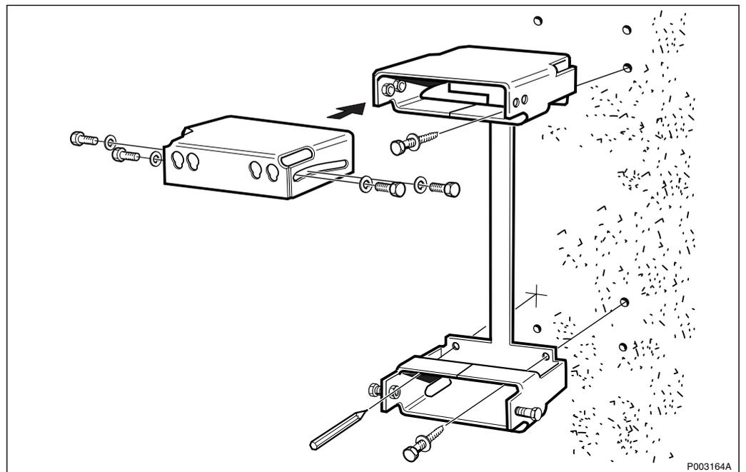
Figure 85 Mounting the mounting fixture assembly on a wall
