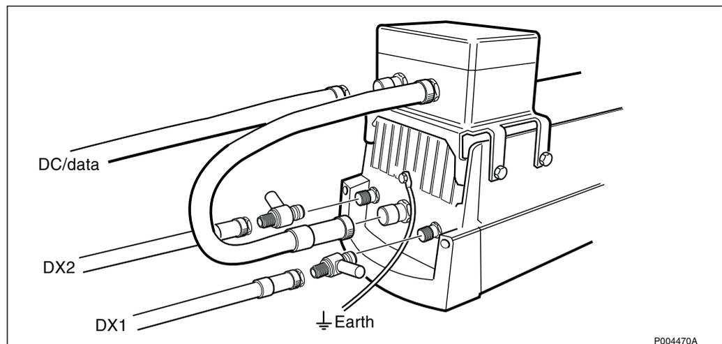
Figure 578 Lightning protection for 500 W EIRP GSM 1800 antenna
