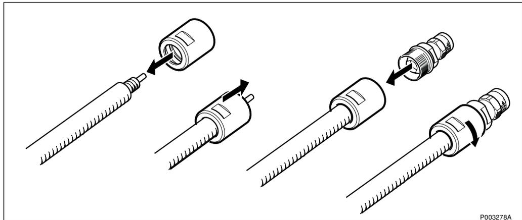
Figure 244 Mounting the antenna connector
