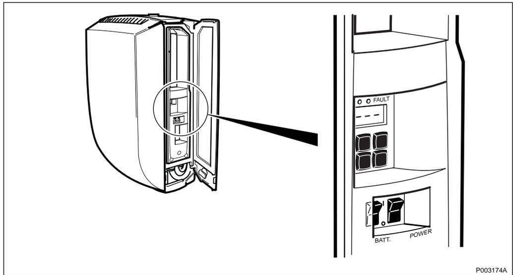
Figure 137 Position of the AC power and battery switches
