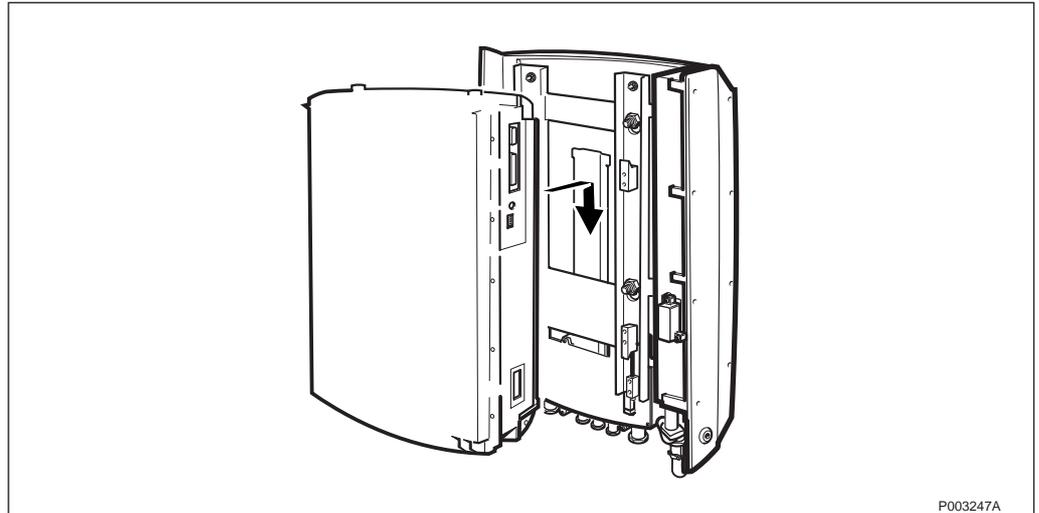
Figure 178 Mounting the cabinet
