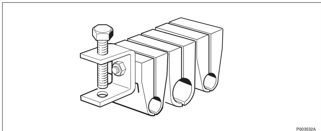
Figure 262 Cable Clamp NTM 201 215/5
