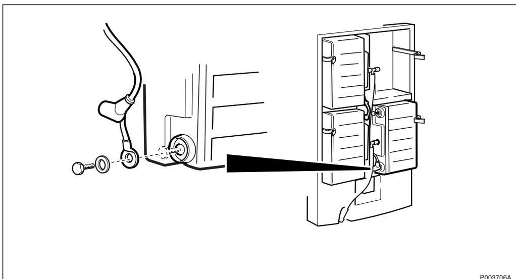
Figure 484 Connecting the minus-pole (-) of battery 3
