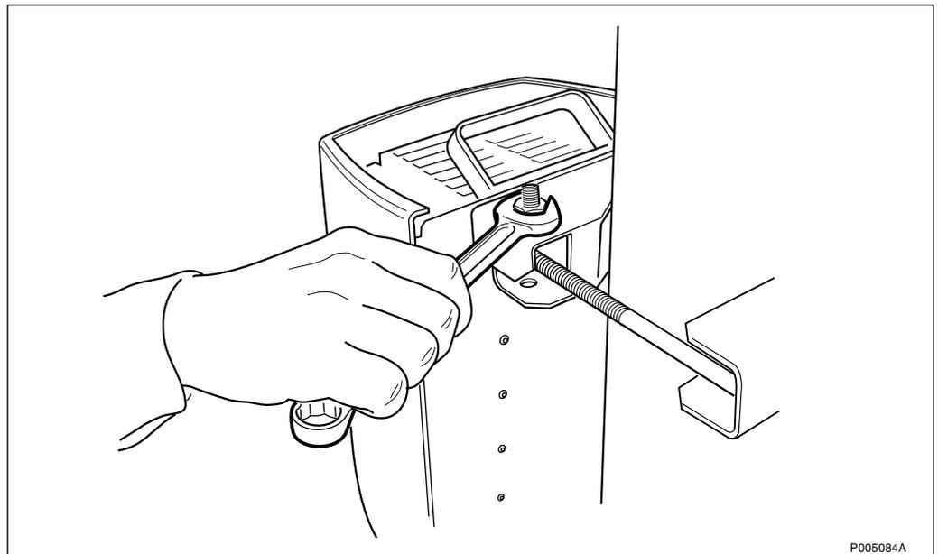
Figure 519 Loosen the locking nuts
