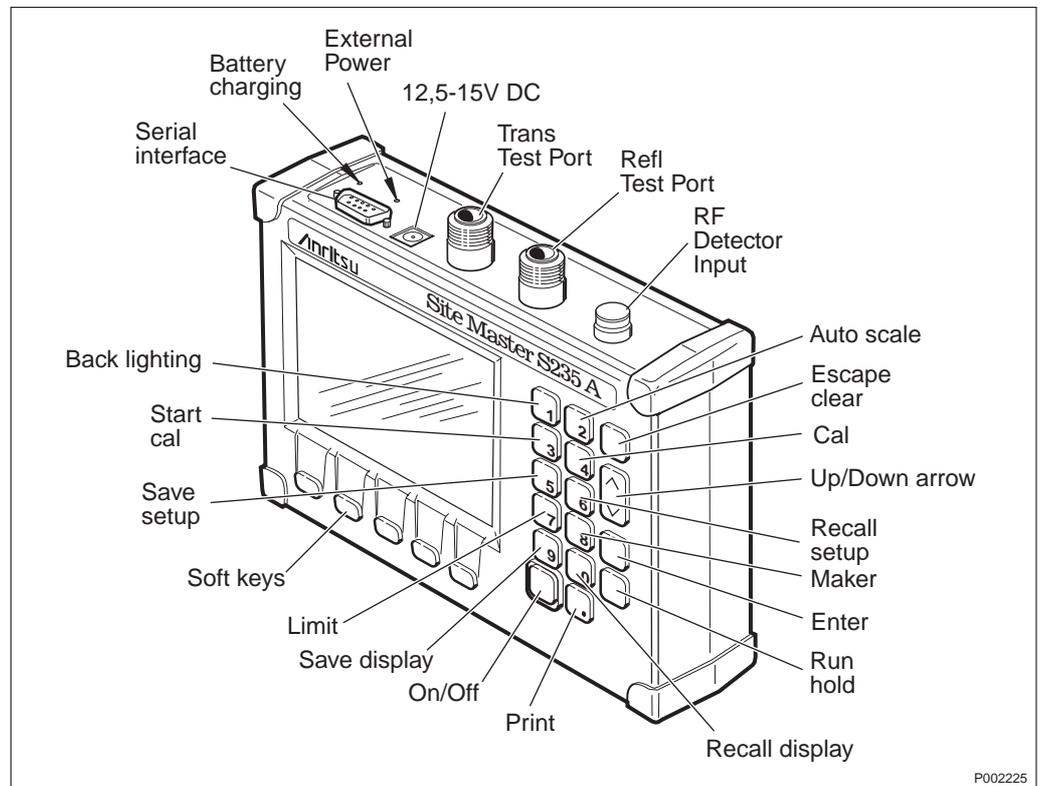
Figure 328 Anritsu Site Master S235A (exterior of S120A is similar to S235A)
