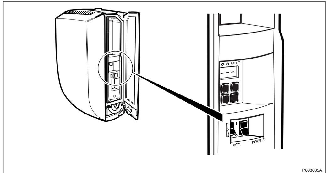
Figure 398 Battery and AC switch in the PBC
